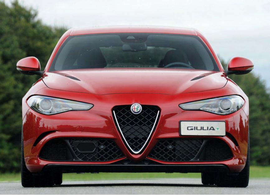
Every Giulia from the cooking 178bhp diesel to the 503bhp QV has the raw materials to be a big deal: lightweight steel chassis with aluminium panels for extra shavings. There's a carbonfibre prop shaft, double wishbone front suspension and a multi-link setup at the back. Alfa Romeo says the weight distribution is an even 50:50.
