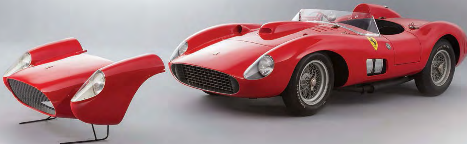
ABOVE: Spare nose section for when the car ran at Caracas in 1957 with pontoon wings to provide extra brake cooling
