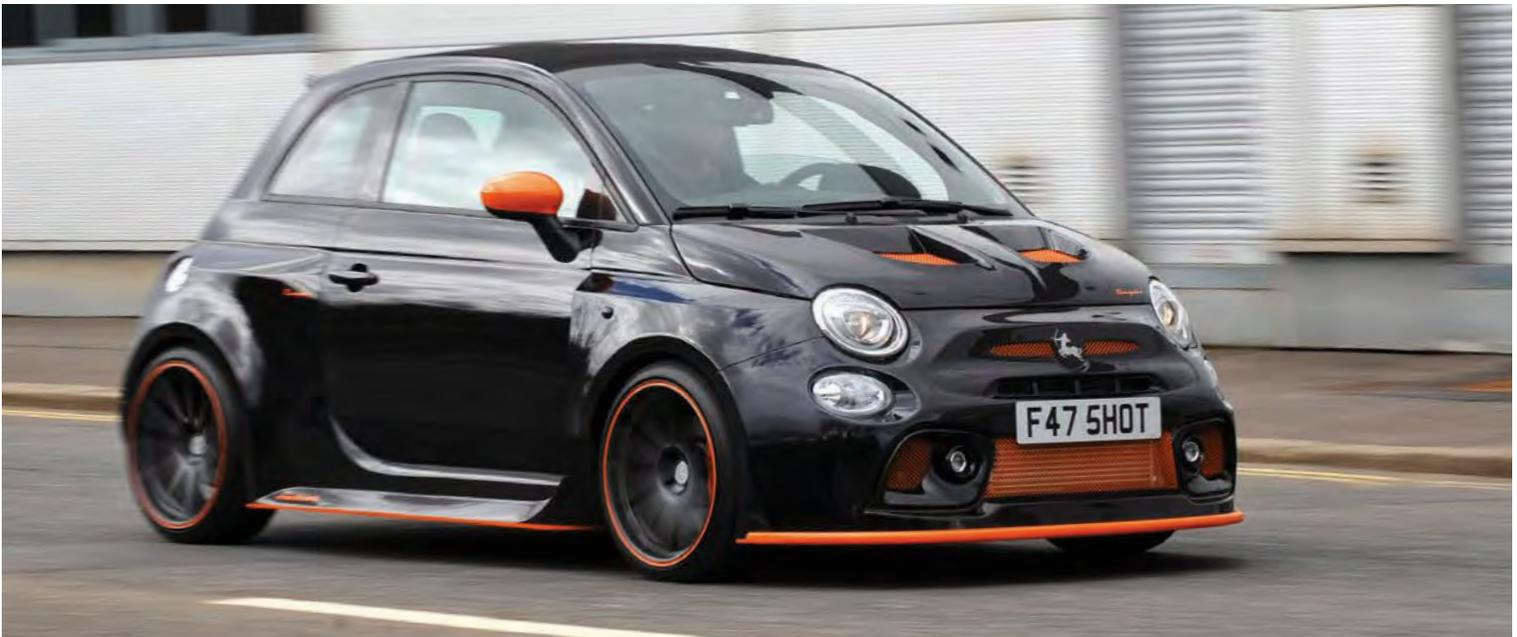
*Big front end has function as well as fury, allowing air to flow into the front-mounted intercooler*
