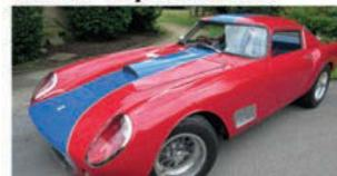
Based on UK supplied 250 GTE from 1962. Aluminium handmade body in the style of a 1958 "Tour de France", mounted on 250 GT chassis. Engine rebuilt to 250 GTO specification, complete with six twin choke carburettor, tuned and "run in" on a dynamometer with output of 307bhp. **£449,990**
