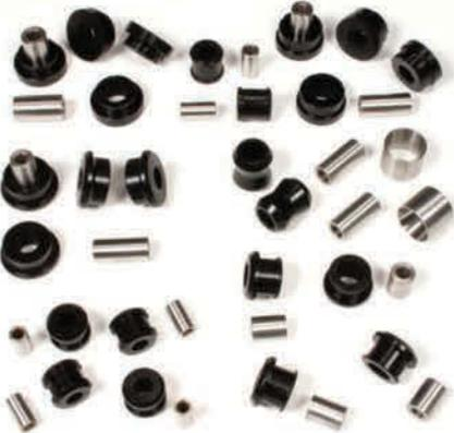
It came to light that there are two size options on the rear spring pan arm outer bush, so we offer both shell size options 39.9 & 42.2 mm OD, so please be aware of this option when ordering. The spring pan arm outer bushes are designed to rock as the original greased steel ball, whilst minimising radial movement – hence the hour glass profile & suitable stainless shell. The sharp edges of the arm housing would be detrimental to a conventional flanged bush.
