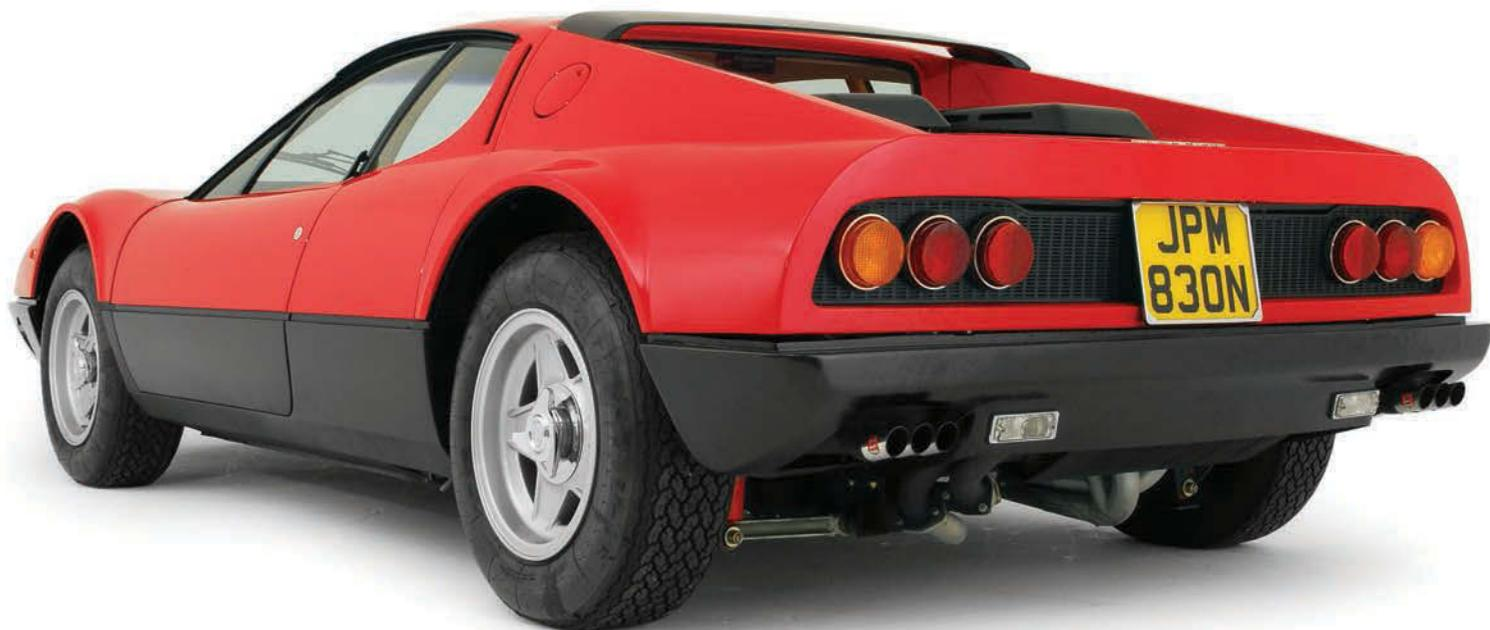
With its 4.4-litre flat-12 engine, Ferrari claimed a top speed of 188mph – a little fanciful, admittedly (it was merely a ‘theoretical’ maximum). But there’s no doubt that this was one of the world’s fastest cars in its day, with a tested 0-60 time of around 6.5 seconds.
