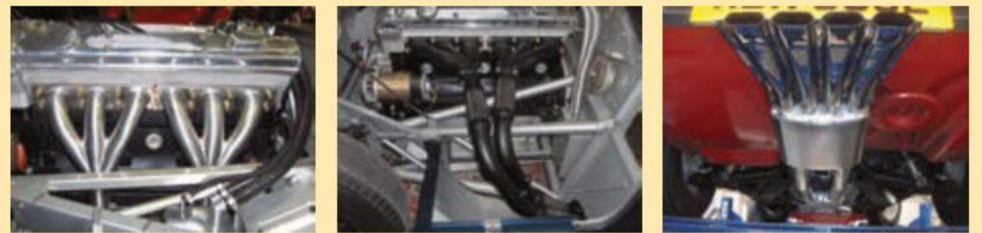
Racing E Type exhaust under construction, with 3 x re-packable silencers
