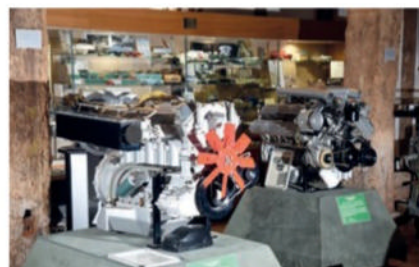
Two of the engines on display include a straight-six from a DB4GT (foreground) and a 5.3-litre V8
