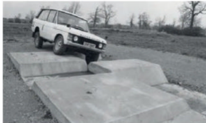
The articulation gauge for Land Rovers in use at BL Technology Gaydon Proving Ground in 1980
