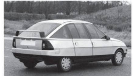
The BL Technology ECV3, a fuel-efficient and aerodynamic prototype developed by BL Technology at Gaydon
