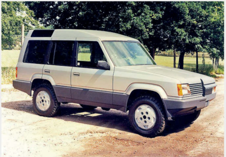
A 1986 design clay for the successful Land Rover Discovery that launched three years later
