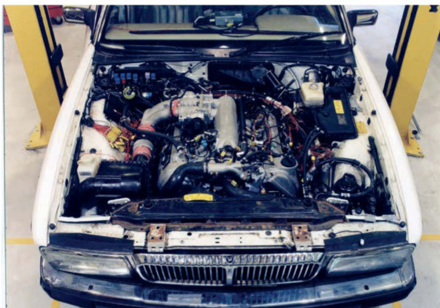
Heart of the XK8 was a new 4.0-litre V8, seen here in an XJ40 test mule
