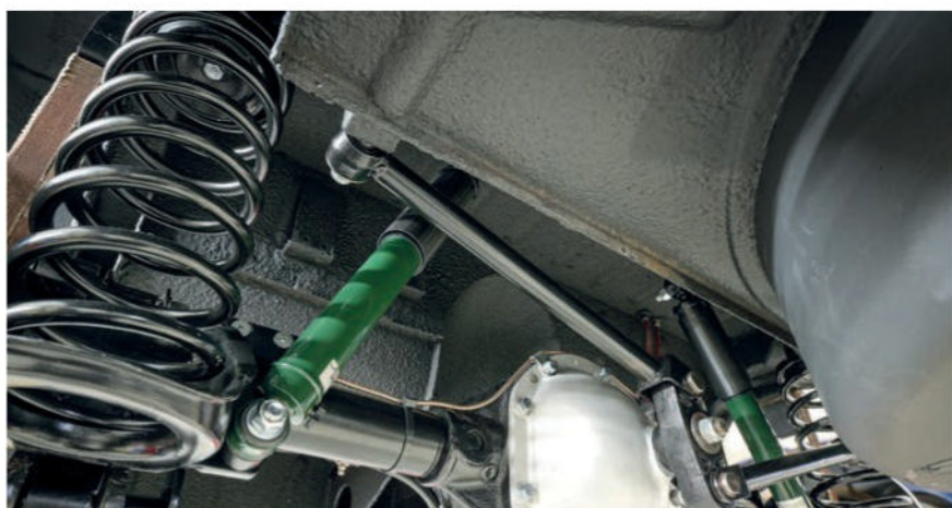
Salisbury 4HA live axle was refitted with new coil springs and modern telescopic adjustable dampers. A Watt's linkage is secured to the centre of the diff casing and there are trailing radius arms at the outer edges of the axle.
