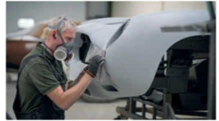
Getting to the stage of a primer'd bodyshell took several weeks, then to the final paint and reassembly took just as long.
