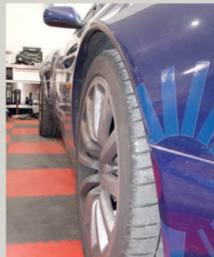
David has fitted spacers to the rear wheels of his V12 Vanquish to help fill out the arches
