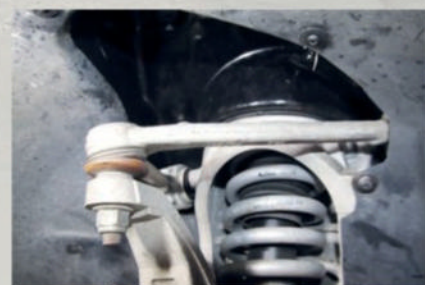
David has discovered that some components on his V12 Vanquish are from Jaguar, such as these front upper wishbones that are also fitted to the S-TYPE
