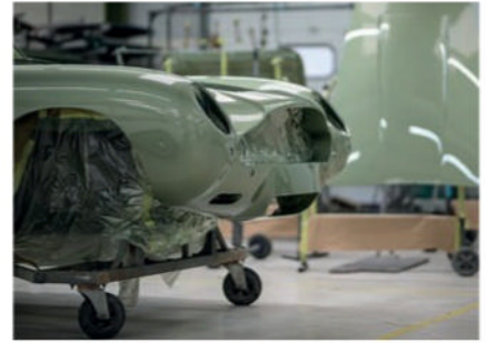
Getting to the stage of a primer'd bodyshell took several weeks, then to the final paint and reassembly took just as long.
