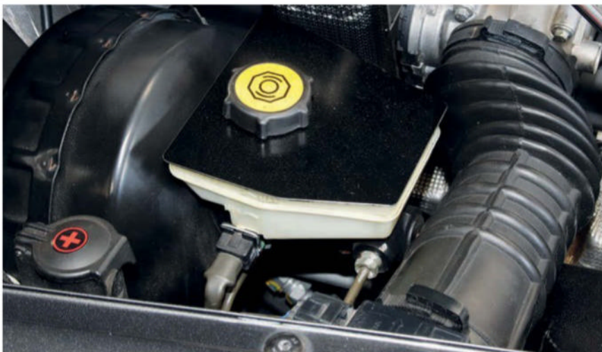
Metal cover over the top of the brake fluid reservoir protects the plastic from sunlight damage
