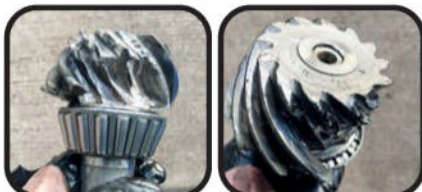
A pinion missing several teeth
