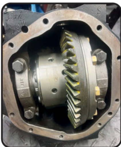
Differential built with a helical automatic torque biasing (ATB) unit
