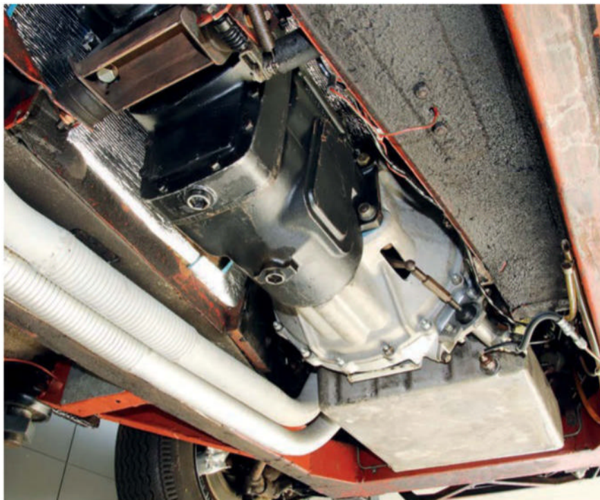
This DBS was originally equipped with a Borg-Warner three-speed automatic transmission, but it has been changed for a ZF five-speed manual
