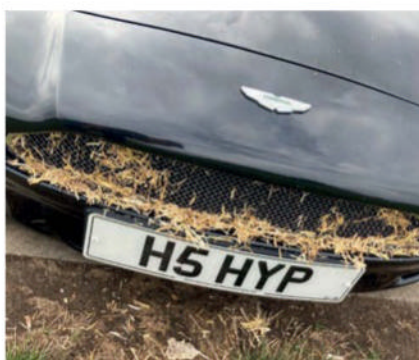
The grille becoming covered in straw saw the engine temperature rise
