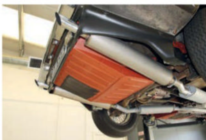
The boot area accommodates the twin fuel tanks and a full-size spare wheel. Judging by the red lead coating on the underside of the boot floor, it has perhaps been cleaned and painted
