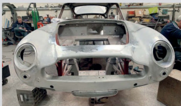
The front end was cut off to repair the steel framework behind it, the aluminium door skins were replaced as a matter of course (the hidden framework cannot be checked without removing the skins) and the rear valance was replaced because it was corroded
