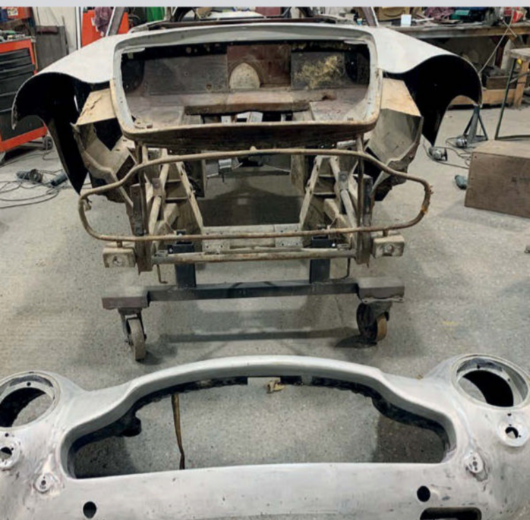
The front end was cut off to repair the steel framework behind it, the aluminium door skins were replaced as a matter of course (the hidden framework cannot be checked without removing the skins) and the rear valance was replaced because it was corroded
