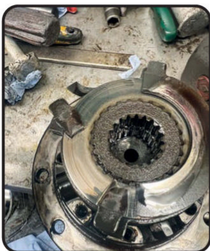
Cracked clutch plates
