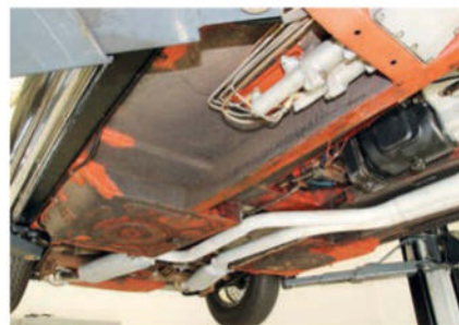
Steel floors and footwells are often notorious rot spots, but these appear to have survived
