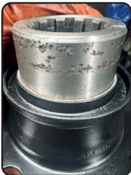
A pinion flange with a damaged seal track
