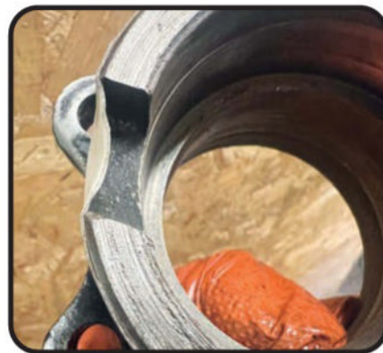
This output shaft housing is damaged because the bearings have been spinning inside the casing
