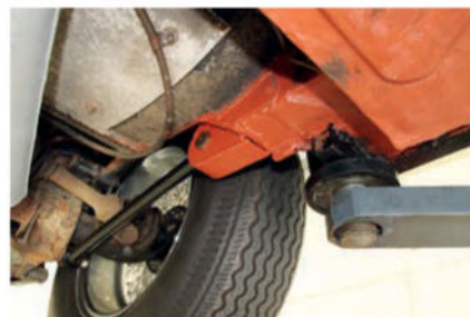
Welding work can be seen around the nearside rear mounting point for the lower trailing arm that's part of the Watt's linkage
