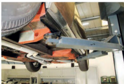
Outriggers and jacking points look new and don't crunch when raising the vehicle on a two-post lift
