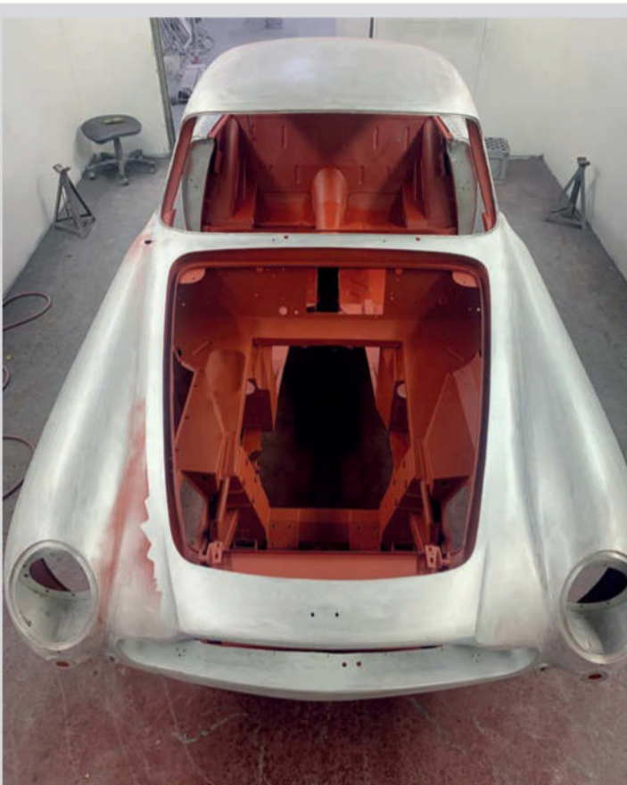
Following the repairs, the chassis areas were coated in the traditional red lead, and the engine bay was finished in gloss black
