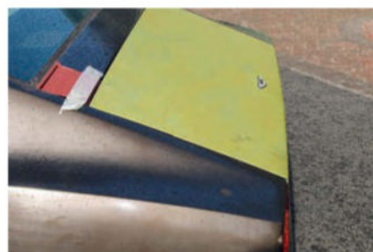
The boot area accommodates the twin fuel tanks and a full-size spare wheel. Judging by the red lead coating on the underside of the boot floor, it has perhaps been cleaned and painted
