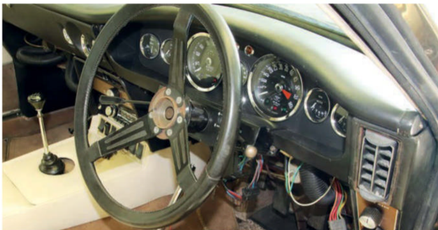
Judging by the wiring that's hanging down, someone has been working underneath the dashboard area. Instruments and switches all appear to be present
