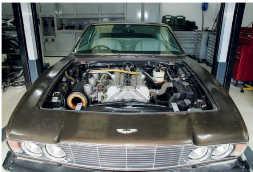
Straight-six 3,995cc twin-cam engine is equipped with triple SU carburettors
