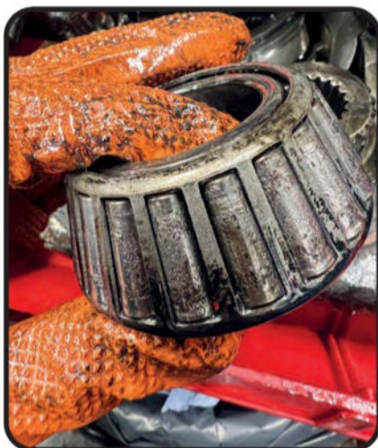
A pinion inner tail bearing with very worn and damaged rollers
