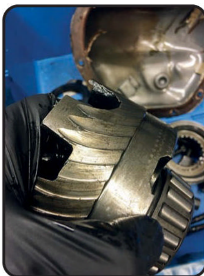
An LSD carrier where the pinion nut has come loose and the pinion has eaten the LSD carrier
