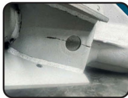
4HA axle with cracked bracketry
