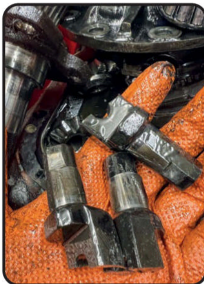
Broken LSD cross shafts are a common occurrence
