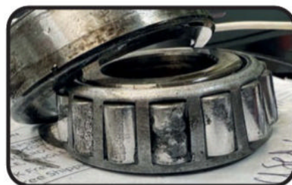
This outer pinion front bearing has visibly damaged roller bearings
