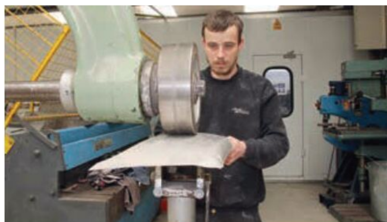
Welder and panel beater Paul demonstrates the dying art of using an English Wheel.
