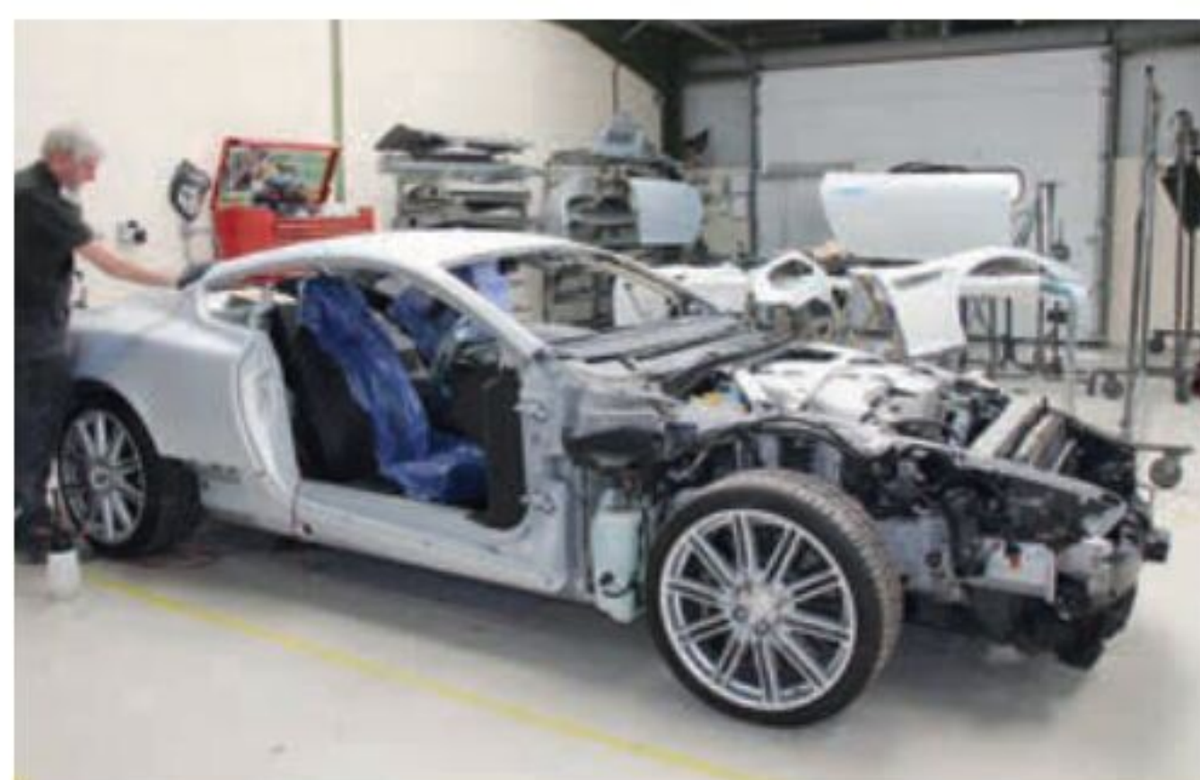
One of the last DBS models stripped of its exterior panels and ready for a respray in the spray booth.
