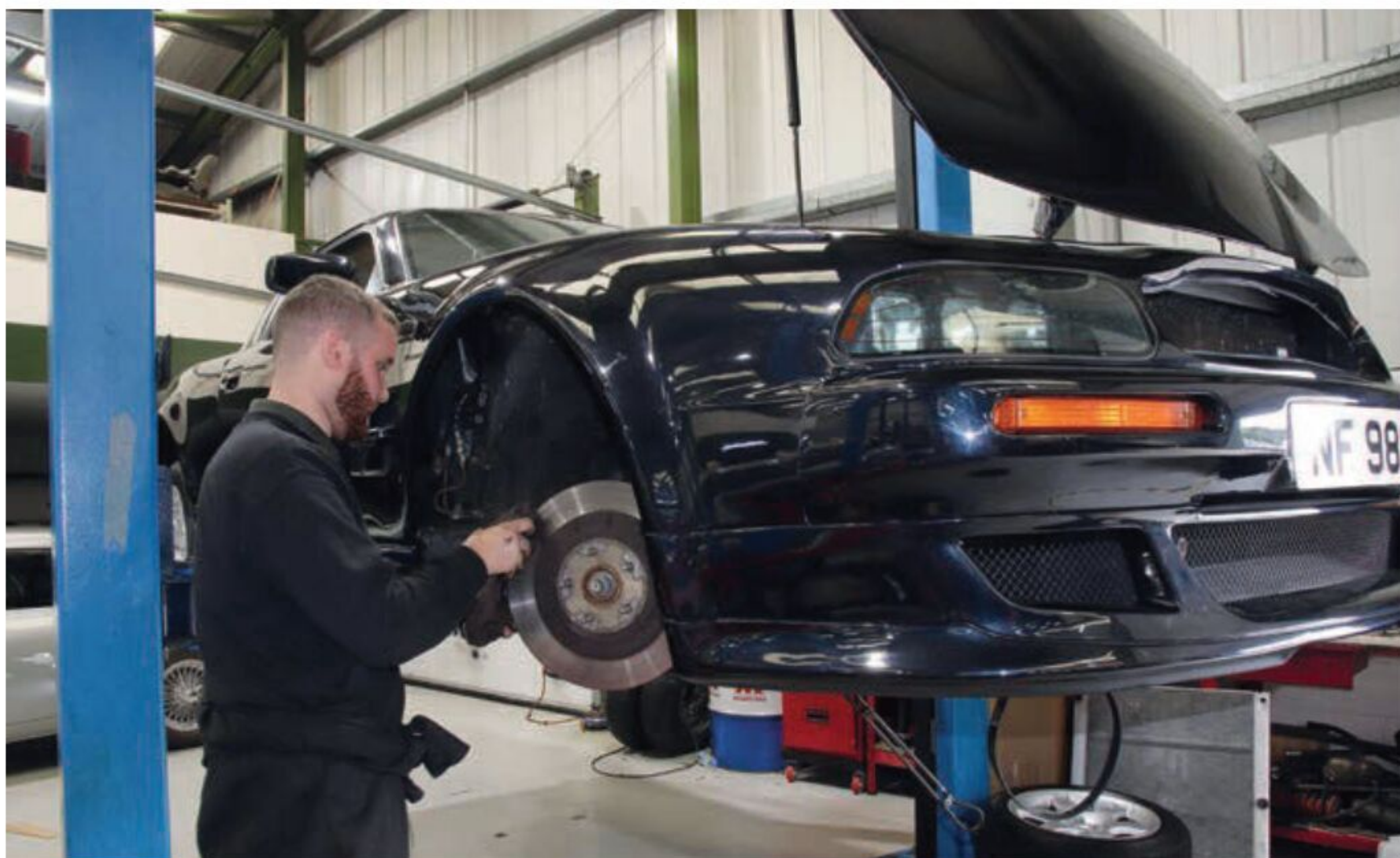
Technician Luke removes the brake calipers from a late Nineties V8 Coupé as part of a thorough and comprehensive service.
