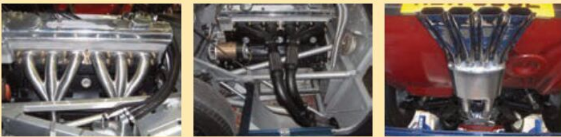
Racing E Type exhaust under construction, with 3 x repackable silencers
