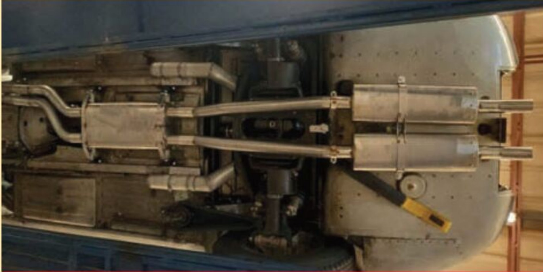
Racing E Type exhaust under construction, with 3 x repackable silencers
