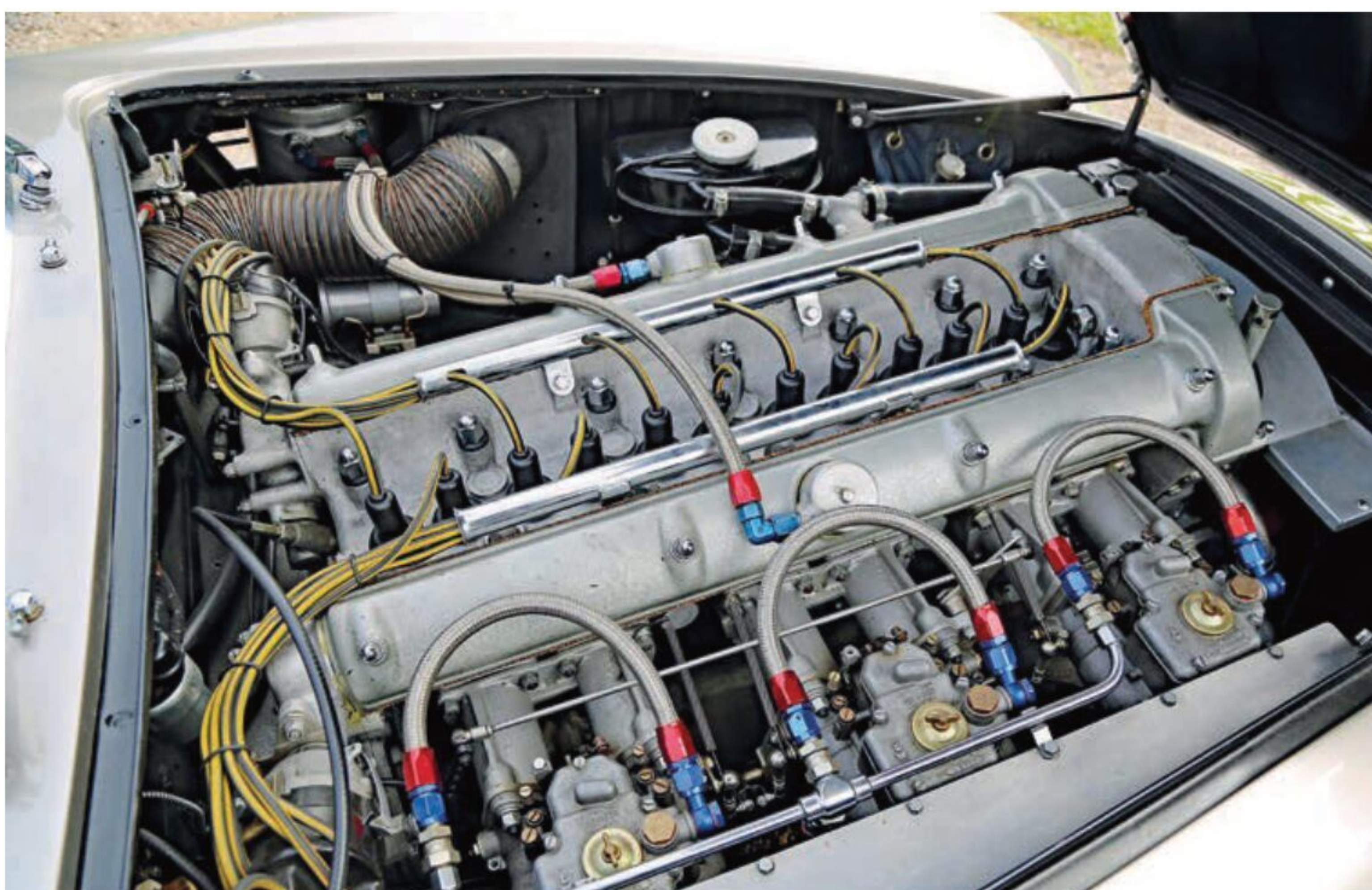
▼ Tadek Marek's six-cylinder engine for Aston Martin went on to power DB4s, DB5s, DB6s and DBSs
