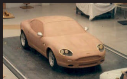
A clay model of the ▶ now Aston Martin-led Project NPX in the early Nineties
