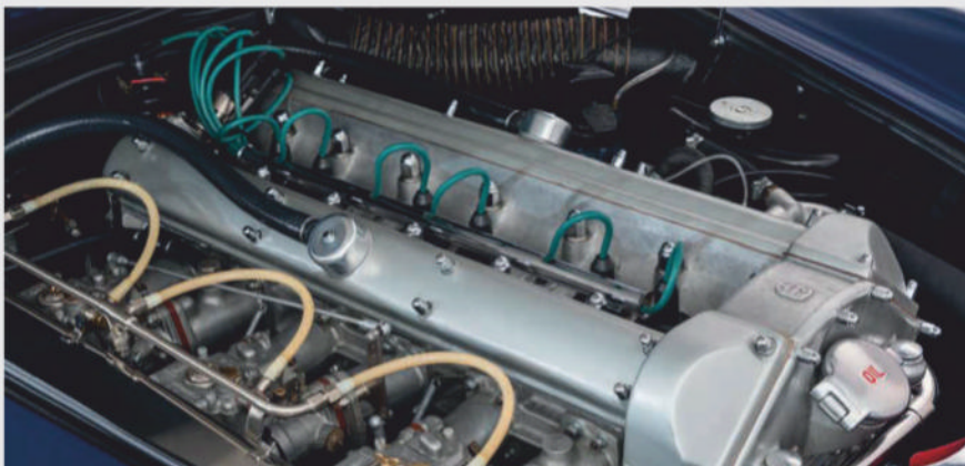
The DB4 was the first road car to use Tadek Marek’s new 3.7-litre straight six
