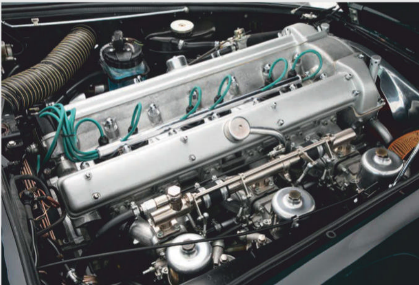
The DB5 used a 4.0-litre version of Marek's straight six which in standard form produced 282bhp
