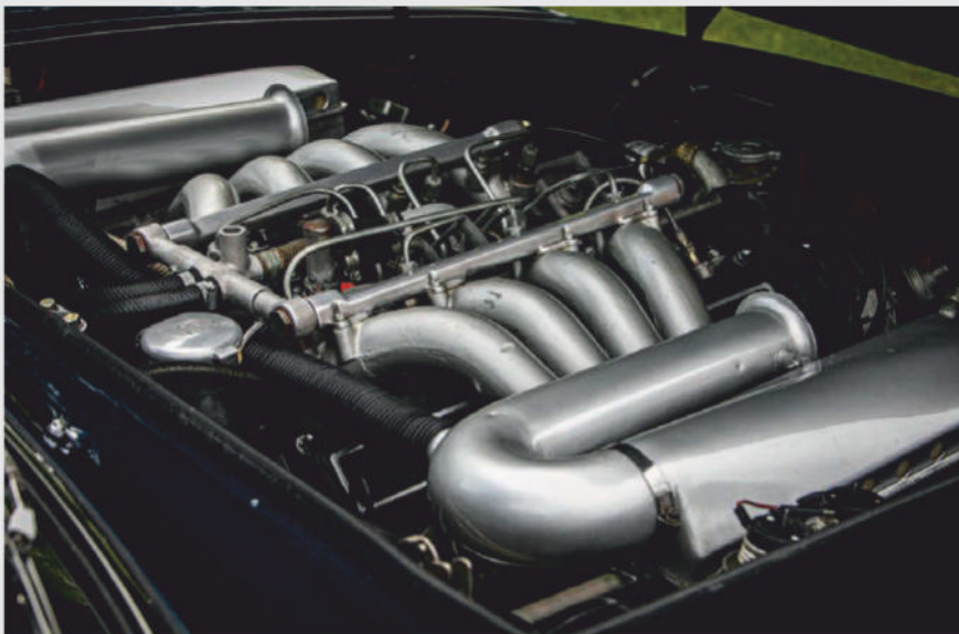
In 1969 the DBS was finally fitted with Marek's new 5.3-litre V8, an engine the car always meant to have
