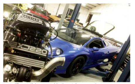
V6's extensive black ceramic coating helps to keep engine bay temperatures down
