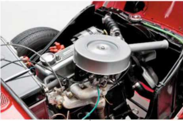
Front-hinging bonnet allows almost unrivalled accessibility to the engine bay
