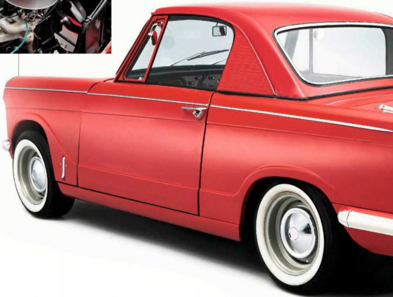
Front-hinging bonnet allows almost unrivalled accessibility to the engine bay
