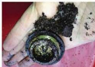
Filth came out with fuel-tank drain plug
