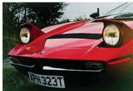
Neat pop-up lamps are powered by Citroën hydraulics
