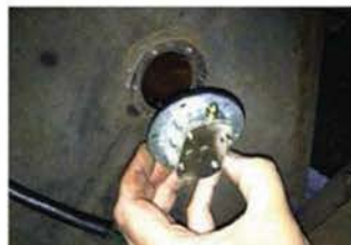
New sender has cured erratic fuel reading
