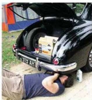
Topping up leaking axle with fresh SAE90
