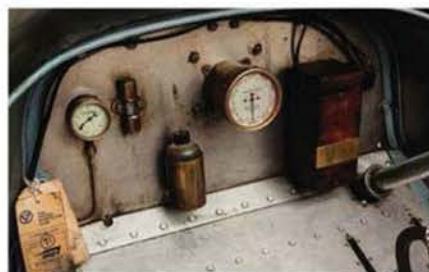
Clockwise: handling is neutral, with a touch of oversteer; wooden box holds coil; minimal gauges for fuel pressure and oil-flow drip-feed meter
