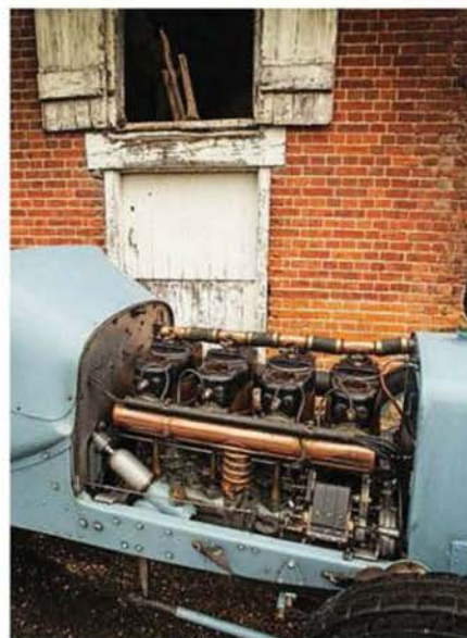
Norfolk could be Dieppe as Walker splashes along – high driving position is key with limited brakes. Right: updraught carb works hard to fuel 12.8-litre 'four'
