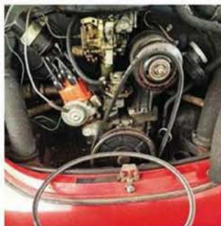
Belt swap cured slipping and squealing
