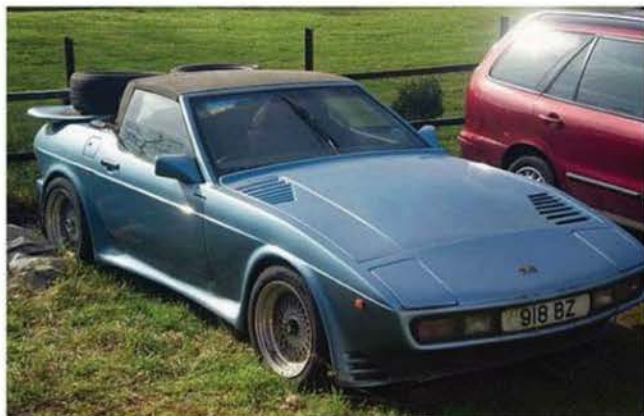
This 420 SEAC not only has the Kevlar bodywork, but also a rare stainless-steel chassis
