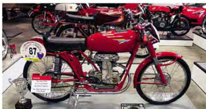
Delightful Ceccato – sole survivor of five made – packs a 75cc Taglioni twin-cam motor
