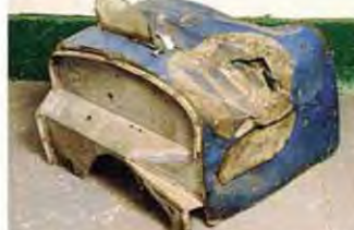
Damaged bulkhead from Delage team car 3
