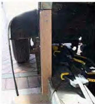
More new wood – repair section on A-post
