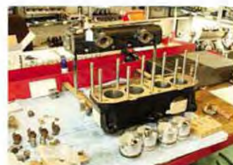
Meticulous reassembly of Meadows engine
