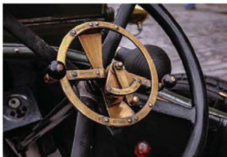
From above: handsome lines with hood raised; steering wheel controls set ignition, mixture and throttle; Zenith carb for the 3969cc 'four', which was rebuilt during post-WW2 restoration
