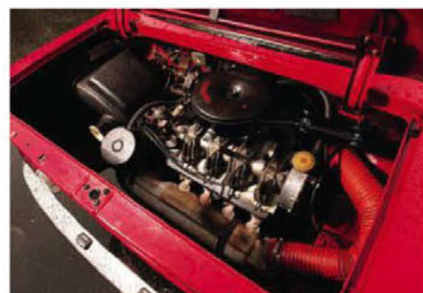
Clockwise: faux grille was intended to give the 1200 a big-car appearance; air-cooled 'four' was bored out from 996cc to 1177cc; seats are from a Metro GTI
