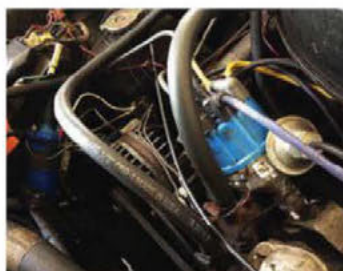
Water hose replaced after checking dizzy!
