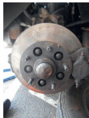
Broken stud was a sign of things to come
