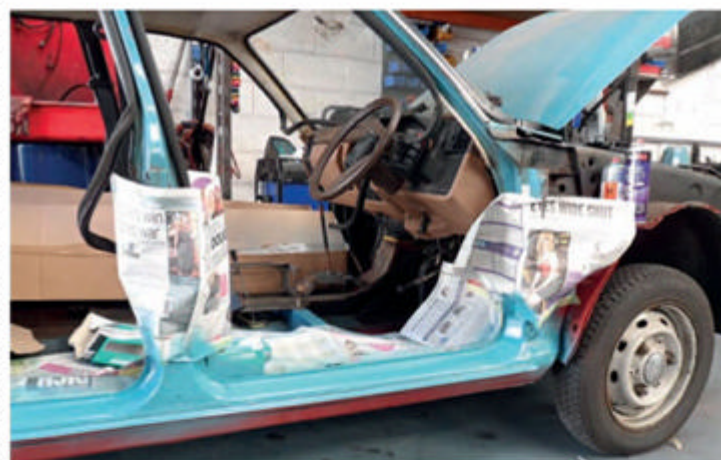
Neatly repaired sill, before colander-like old doors went back on – nice Pallas dash, too
