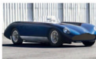
Smooth one-piece body is all glassfibre
