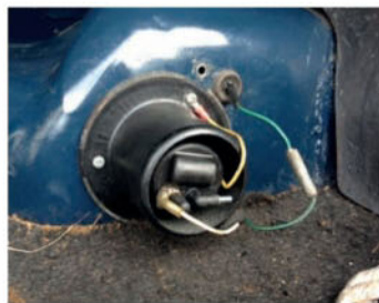
Solid-state fuel pump should aid reliability
