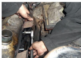
Winding the new manifold studs into head
