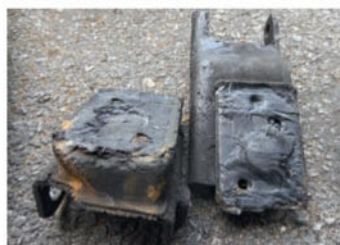
At least engine mount failed before fitting
