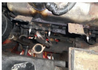
New core plugs (below) a manifold-off job
