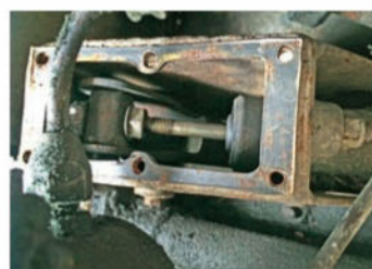
Brake pedal height adjusted at pushrod
