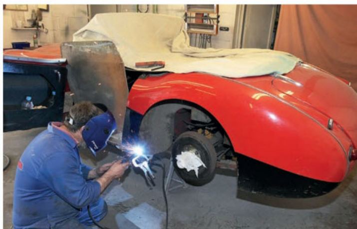
New steel being welded into the Healey's sills, replacing the former gaffer-tape bodge
