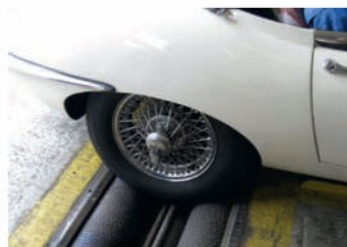
Rolling road is adapted for Powr-Lok diffs
