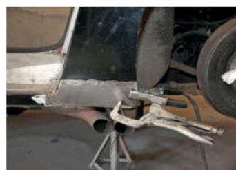
Repair section carefully clamped into place
