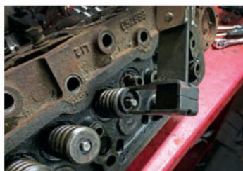
Stripping down the 8:1 CR cylinder head...
