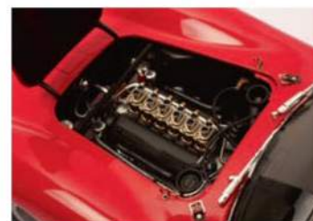
Six twin-choke Webers on Colombo V12
