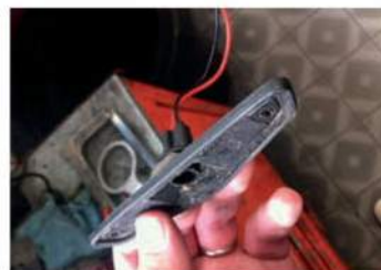
New bulb holder carefully glued in place
