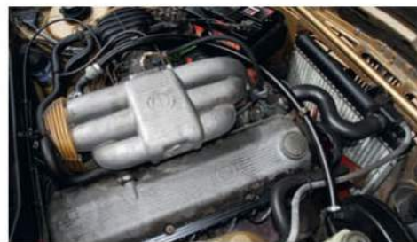
'Six' a bit grubby but no sign of leaks; new plugs and leads
