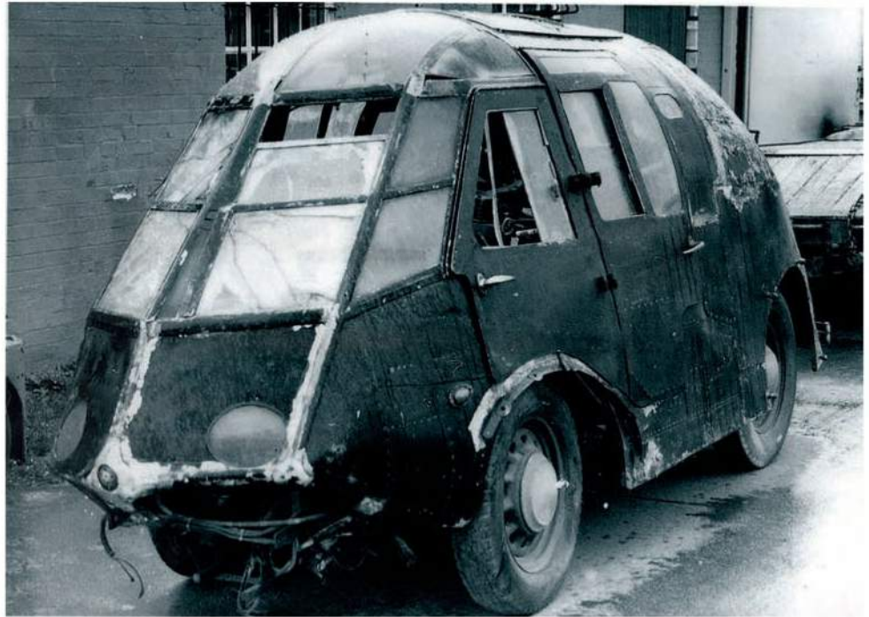
Above: the nose from Blenheim Mk1 L6739 was rescued by Ralph Nelson after WW2 and used on an Austin Seven chassis to form an electric car! It was taken off the road in 1957 before eventually being donated to the rebuild. Left: the Freddie March concurs is a popular Revival attraction
