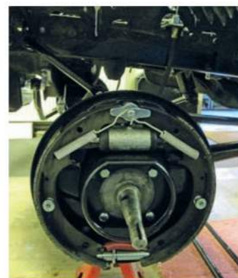
New shoes and cylinders so it stops better
