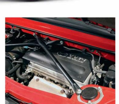
The VVT 16-valve twin-cam **engine** is a classic modern all-aluminium unit: revvy, powerful and remarkably durable if well maintained (many have reached 150k+ miles without problems). Look for a full service history, no warning lights or fault codes, and ideally evidence that pre-cat issues have been addressed
