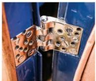
Clockwise from main: Type 575's lines were crafted by English coachbuilder Corsica; unblown 3.2-litre straight-eight has punchy performance; snug cabin, low seat; holes drilled in 57.375's door hinges, in pursuit of lightness
