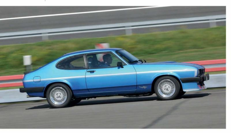
ord called it the 'Capri 78', but the more logical 'Capri III' soon prevailed and many saw the third-generation model as redemption for the disappointing Capri II. The lower bonnet reduced lift over the front axle and underbody protection was improved, although it's far from immune to corrosion.
