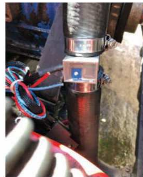
Control sensor was spliced into rad hose
