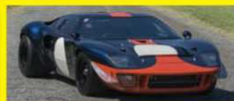
FORD GT40 MK1, Precision constructed to '68 Le Mans winner specs. Stainless steel monocoque, ZF trans axle, BRM magnesium wheels, small block 325 cubic inch, V-8 Dart Windsor. Gurney Weslake cylinder heads, Webbers, A/C. 200 miles since completion.
