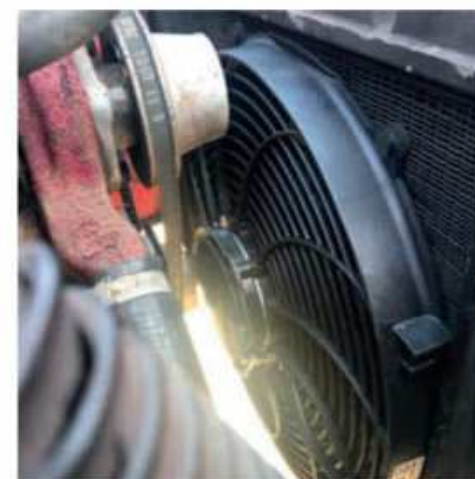
Electric fan replaces ineffective original
