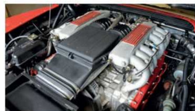
Flat-12's cam covers have been refinished by QV London
