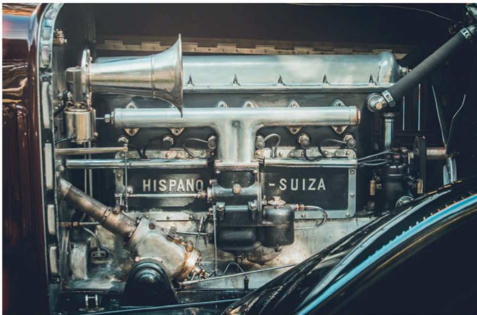
Clockwise from main: you're the one working hard on a rural run; strong overhead-cam 6597cc 'six' has bags of torque; it's all in the details, such as the exquisite gearknob for the three-speed 'box; this car's body shows its regular use
