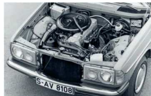
M123 single-cam 'six' had finger rockers and a Solex carb
