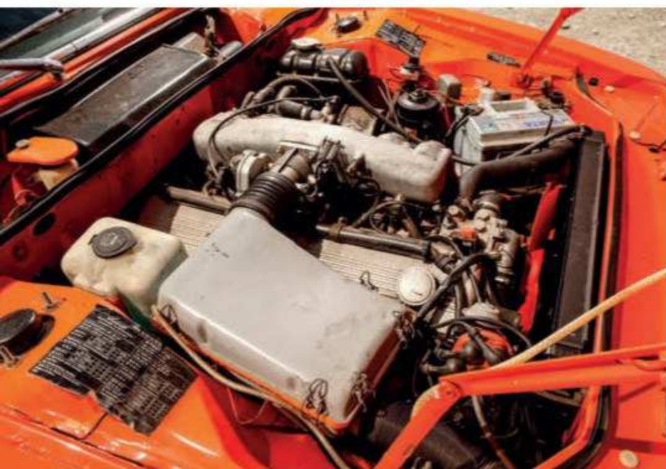
Clockwise from top: great all-round visibility and super driving position; big boot aids practicality; Bosch D-Jetronic injected 'six' leans over at 30°
