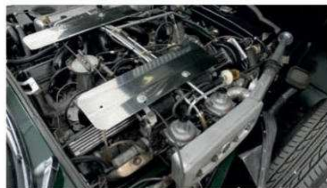
New distributor and high-torque starter, so V12 fires easily
