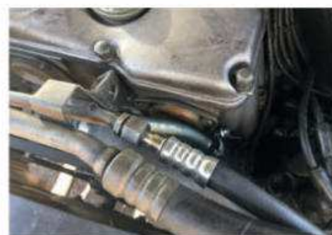
New power-steering hoses cured weeping
