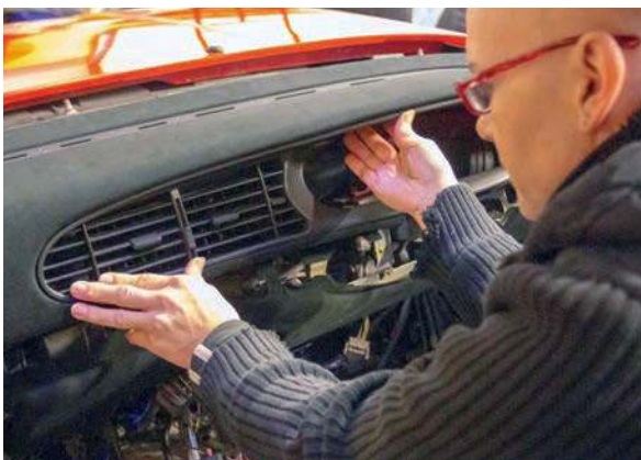
Previous spread Dashboard vent recess insert started out as a plastic part before evolving into steel painted black
