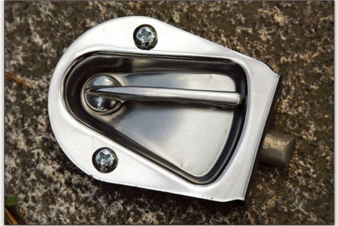
Though most trim components had held up well, the ramp latch had taken more than its fair share of weathering and hard use. The rechromed component shines better than new and operates flawlessly when opening the restored ramp.
