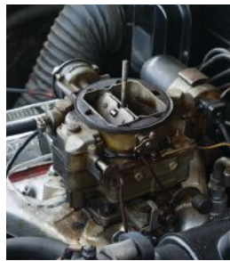
Huge chromed air cleaner atop the De Soto Hemi comes away by twisting a single wing nut. Aluminum sheet fills gap left by Ghia's huge engine setback. Unsurprisingly, Hemi is topped by a Carter AFB. Chrysler generator is backed by a power steering pump; there's no air conditioning.
