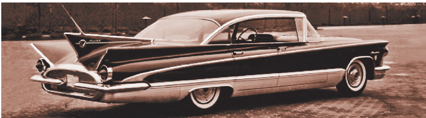
This 1959 Buick concept car sported a large central fin with integral antenna fitted to the top of the trunk lid on a four-door hardtop body.
