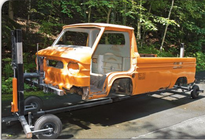
With the Rampside disassembled, it was mounted on a rotisserie so that it could easily be moved around the shop and worked on. The original Omaha orange paint had been the fleet color for the first owner, who had bad luck with the Rampside.
