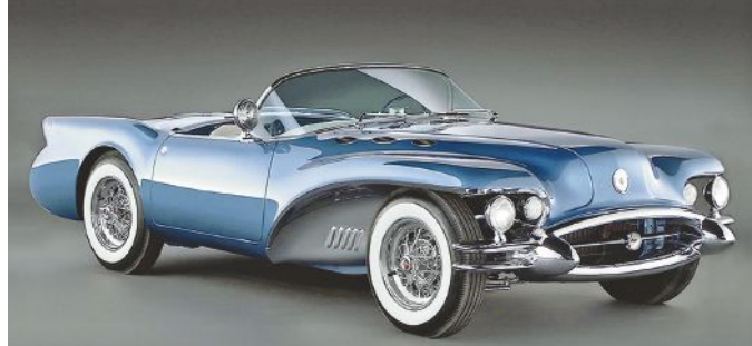
The Buick Wildcat II debuted for 1954 and came closer to the sports-car ideal. Its fiberglass body and four-carburetor V-8 power made this one very fast concept.
