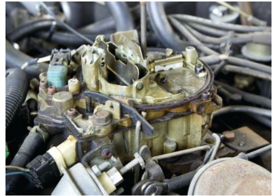
The 307-cu.in. small-block V-8 is entirely original and puts out 140 horsepower, so climbing hills can present a challenge even with the four-barrel carburetor, shown here in factory form.
