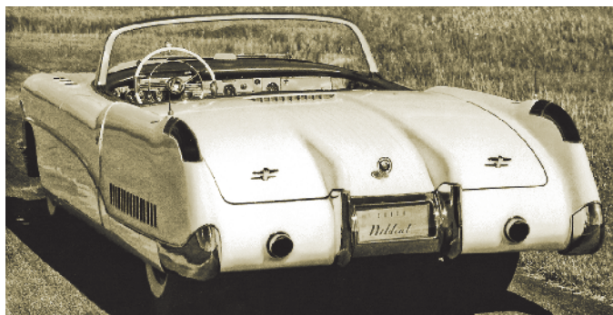
Rear view of the 1953 Buick Wildcat shows sloping rear deck and dual exhausts.
