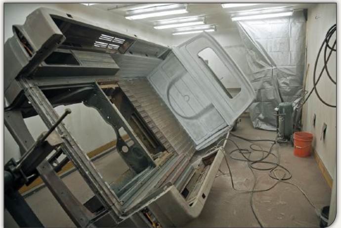
With its 360-degree access, the rotisserie allowed the undercarriage of the Rampside to be painted in a detailed manner, giving the once forgotten pickup a truly top-notch, bottom-up restoration.
