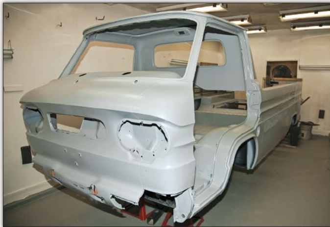
Three coats of Martin Senour 2K Primer Surfacer were each smoothed down with up to 600-grade paper. A final coat of sealer was applied before base colors were laid down. Very little body filler was used, no more than \frac{1}{16} th of an inch at the most.
