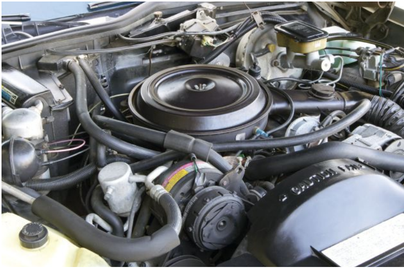
The 307-cu.in. small-block V-8 is entirely original and puts out 140 horsepower, so climbing hills can present a challenge even with the four-barrel carburetor, shown here in factory form.
