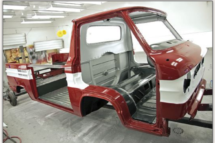
Three coats of Martin Senour Crossfire Platinum base were used for the white-and-Romany Maroon two-tone before they were top-coated with four layers of clear. All were painted at the owner's well-equipped home shop paint booth.
