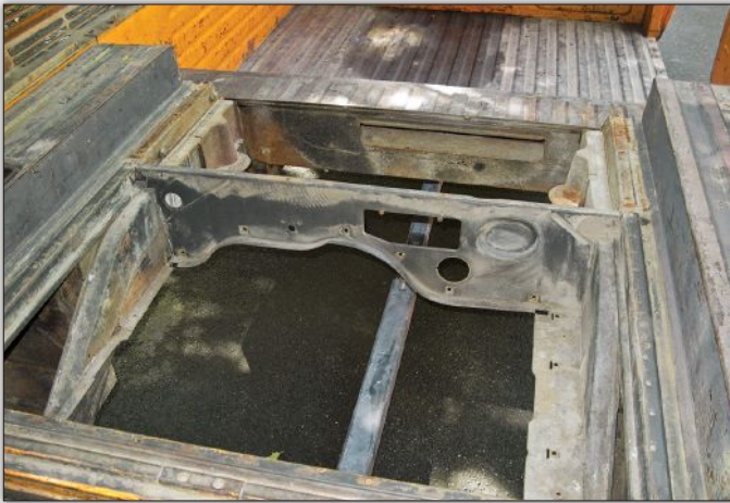
The engine bay, easily visible here with the bolt-in engine covers removed, sits high in the bed and behind the rear axle. It was largely solid, but much like the rest of the lower extremities, did require some work due to so much salt exposure.
