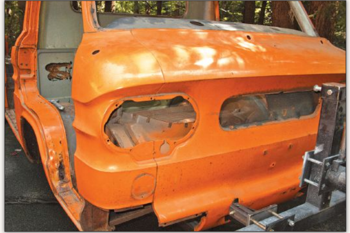
Proper restoration meant removing any and all components from the Corvair's unit-body chassis, including all doors, glass, lighting, wiring, suspension and undercarriage, the entire interior and all decorative trim.
