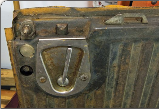
When restoring the ramp, which had to be disassembled, precise alignment of the guiding pin was critical, as the closed ramp provides an important structural component for the bed that would otherwise flex substantially when the pickup was moving.
