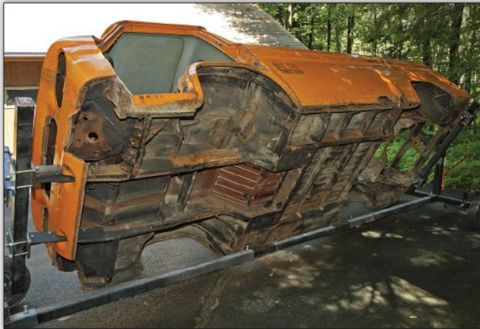
Despite being stored indoors for over 20 years, the Rampside still continued to corrode in some places. Though the rot was largely confined to the lower extremities, it also included the integrated frame pieces.
