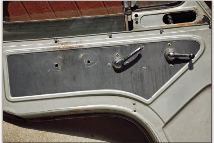
New England winters spare no steel. Even the doors required removal of some surface rust and complete disassembly and re-assembly. After removing all glass, polishing compound was used to brighten up each piece before re-installation.
