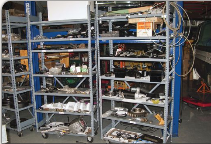
Organization is key to any successful restoration, but particularly one when a car is completely disassembled. Parts were organized onto heavy-duty roll-around shelves with each component labeled and organized accordingly on the appropriate shelf.
