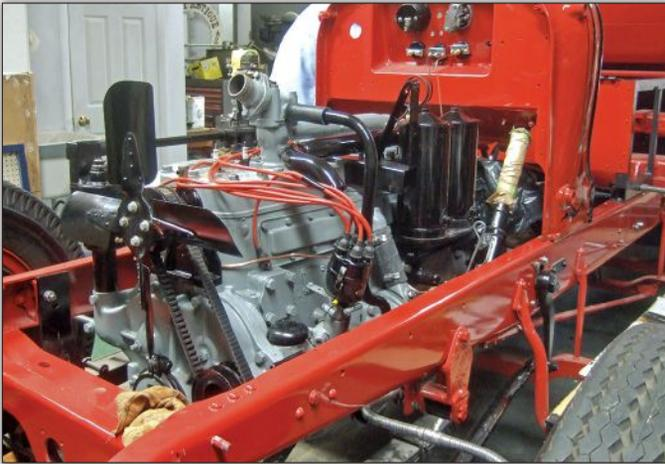
Using reproduction materials, the engine has been wired, as have the rest of the components requiring electricity for operation. Note the two large vacuum tanks near the cowl and the incredibly wide pulley and fan belts.
