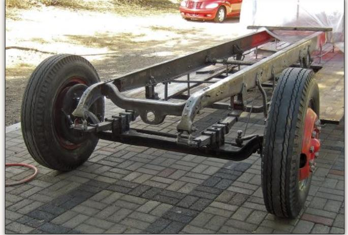
Primer and paint is next on the list for the Seagrave chassis. The back half is already under cover and receiving its treatment. Note that the basic suspension parts have been left in place, done so to assist its mobility to and from the clubhouse confines.
