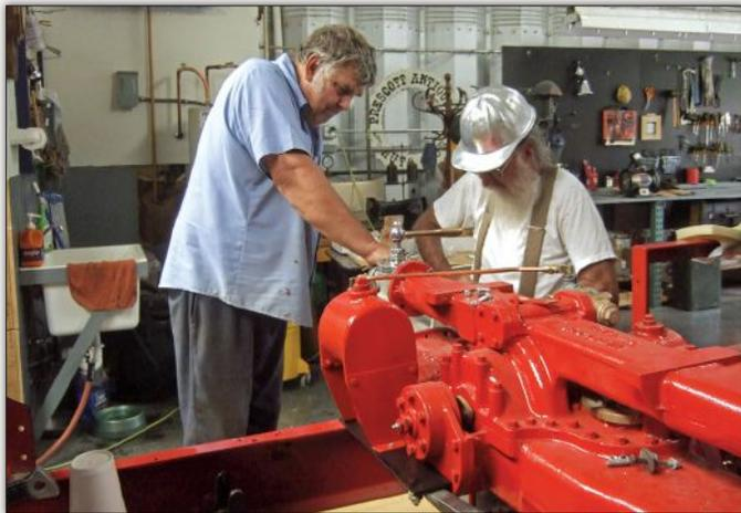
An incredible amount of preliminary work went into locating the replacement water pump, which paid off when it came time to introduce it to the chassis on a more permanent basis. Several details needed to be addressed before its housing could be fabricated.
