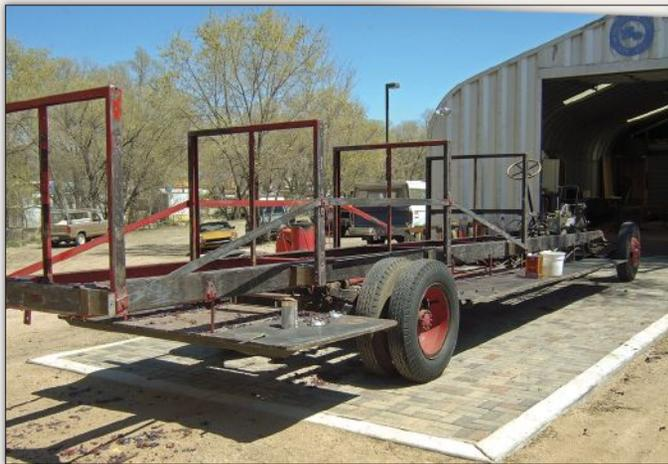
With exception of the suspension systems and the ladder bed framing welded into position at the Seagrave assembly plant, everything has been removed from the chassis, most of which has been painstakingly stripped to bare steel.
