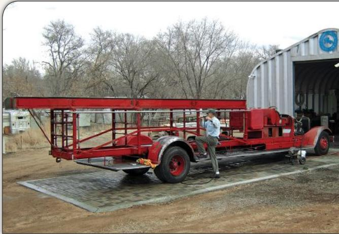
With the truck outside of the clubhouse building, members have already begun the disassembly process by removing hoses, wooden ladders and miscellaneous parts. A thorough power wash removed grime to help expedite the next restoration phase.
