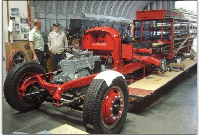
The engine, cowl—now outfitted with its refurbished factory gauges—and water pump have been installed. At the opposite end, the full complement of restored ladders has been carefully loaded into the associated steel framing; running boards are next.
