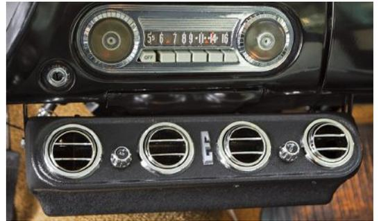
Natural-look carpet warms up an otherwise austere cabin. A brace of conventional instruments flank the floating-drum speedometer. Air-conditioning was dealer-installed. Teletouch shifting was a signature option in 1958, its buttons operating more smoothly than other pushbutton-selected transmissions of the day.
