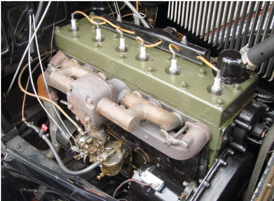
While the Hupp Motor Car Company used parts from other cars in its Hupmobiles, the Century Six engine was of the company's own design: L-head, displacing 211.6 cubic inches, and producing 70 horsepower.
