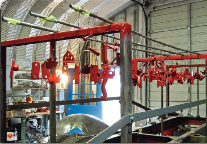
Although the chassis still required some preliminary work, the ladder bed framing became a handy makeshift spray booth for small bolt-on components, which were then left in place to cure before being placed into temporary storage until needed.
