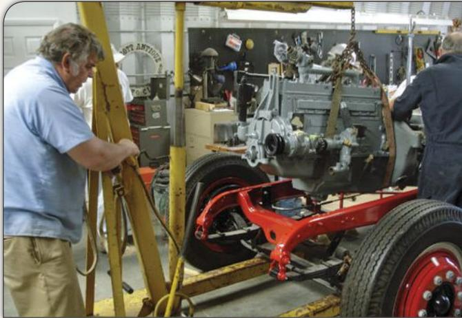
The Hercules engine is being lowered into position. This massive six-cylinder was rated for only 143 hp; however, it was selected by the factory not for speed, but rather its torque—a whopping 488 lb.ft.—to drive the water pump with ease.
