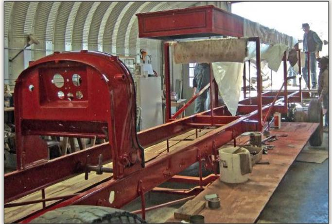
Here the cowl has been reunited with the chassis, while at the opposite end, members are carefully repositioning the upper ladder bed. Look close and you'll note that this upper structure has been carefully pinstriped based on pre-restoration photos.
