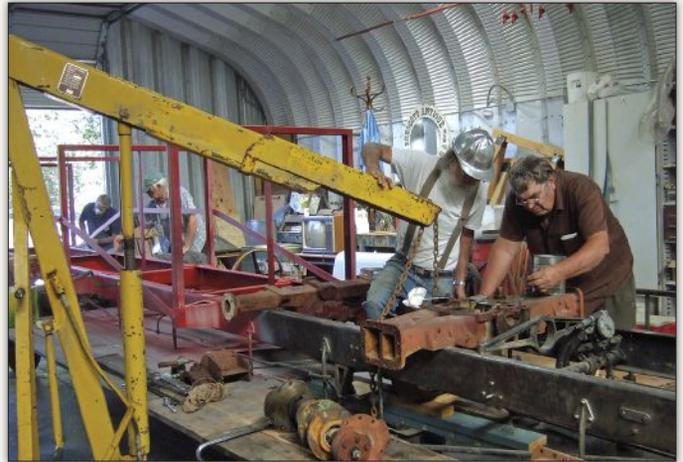
With the front of the chassis stripped of factory paint, club members carefully positioned a new period-correct water pump's mounting points on the frame. This hefty fabrication work done now eliminates the threat of damaging the restoration later.
