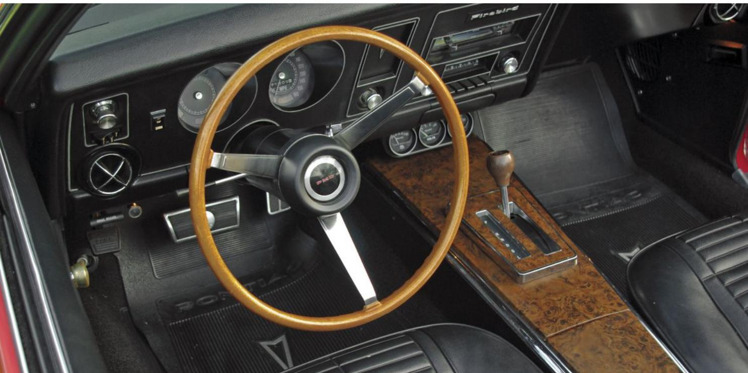
**Geno's standard Firebird interior has an optional console and steering wheel (gauges are aftermarket).**
