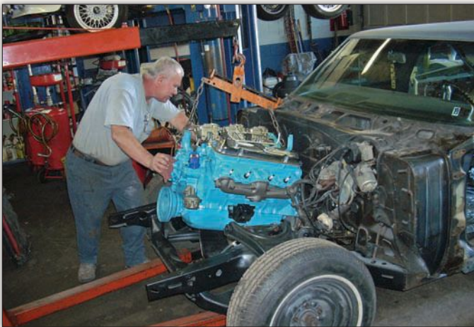
The Tri-Power was added to the engine and the Hydra-Matic was serviced while they were out of the Pontiac. Bill snapped this photo of Terry as he lowered them onto the frame. Before starting the 389, Bill allowed the engine paint to cure for a week.
