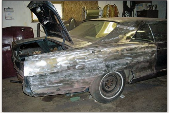
With the shell taken down to bare metal, the absence of rust in the typical areas became obvious and was very encouraging. Unfortunately, various previous war wounds were also discovered. Note the crease in the lower-middle of the quarter panel.
