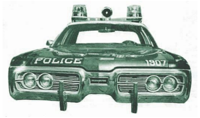
Another warning setup under evaluation was this rack with a pair of rotary beacons and an electronic siren.
