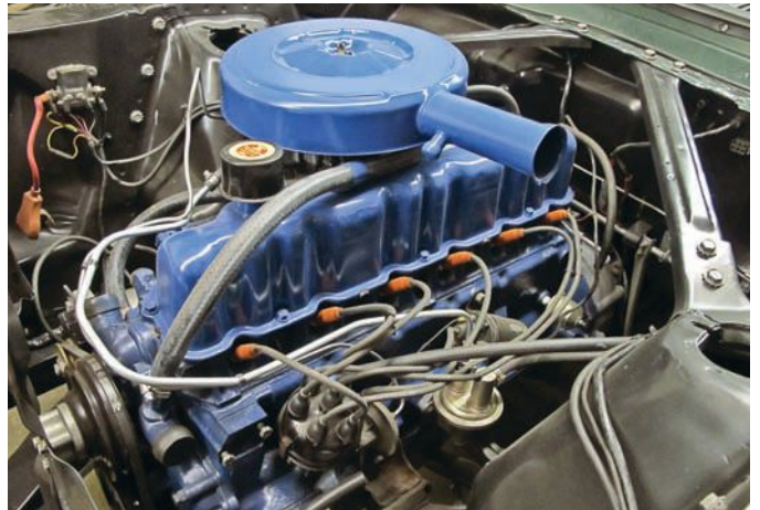
A 429-cu.in. V-8 in Bill's fully restored 1970 Boss Mustang dwarfs a 200-cu.in. six-cylinder in a customer's in-process pony car.
