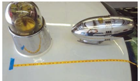
High-mounted Federal beacon with two-colored lamps was standard, like the shrieking Pulsator siren. Each was positioned on the Fury III using measurements from the NYPD shops. Patrol car's number, 1002, comes from the sergeant's badge number of the owner.
