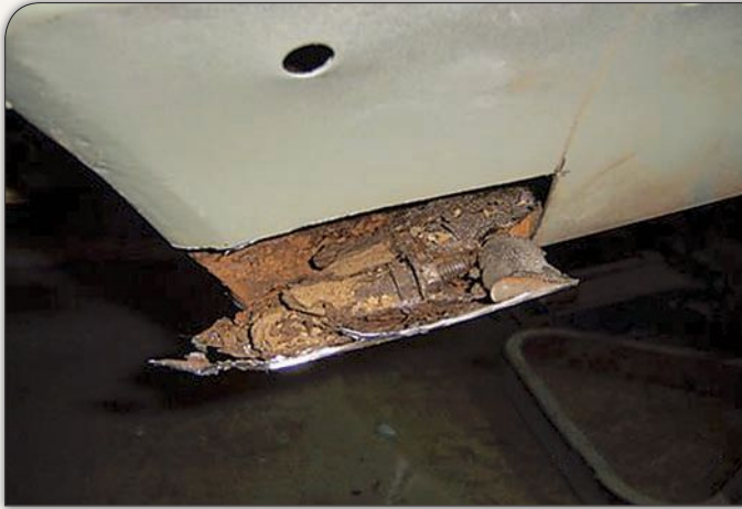
Just behind the driver's-side rear wheel well was a quarter-sized rust hole. When restorer Terry Marsh cut out the section to weld in a new patch, rusty hardware was revealed. Happily, this small area represented the most serious rust in the whole body.
