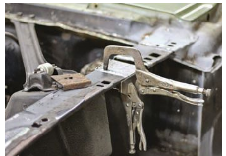
This 1967 Mustang convertible revealed the horrors of rust on closer inspection. Rotten, rusted metal is removed and replaced.
