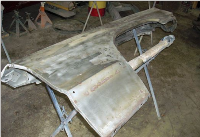
The passenger side front fender was amazingly clean, given its 40-plus years of living in the rust belt. However, like many of the body panels, this original stamping was also very wavy, so a thin coat of filler would be required on certain sections.
