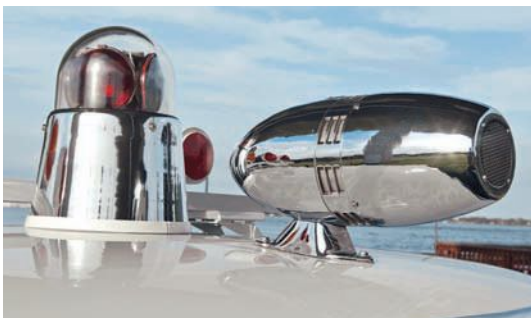
High-mounted Federal beacon with two-colored lamps was standard, like the shrieking Pulsator siren. Each was positioned on the Fury III using measurements from the NYPD shops. Patrol car's number, 1002, comes from the sergeant's badge number of the owner.
