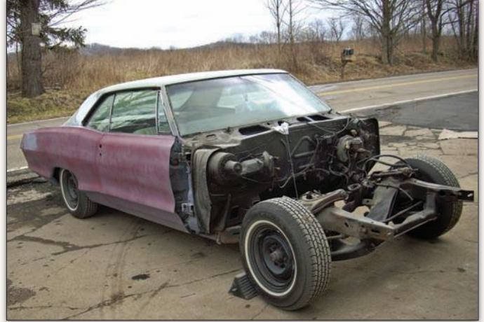
Terry employed various lengths of sanding boards and differently shaped sanding blocks to help better follow the contours of the body. Note the remnants of a red guide coat he applied to reveal high and low spots on the panels during block sanding.
