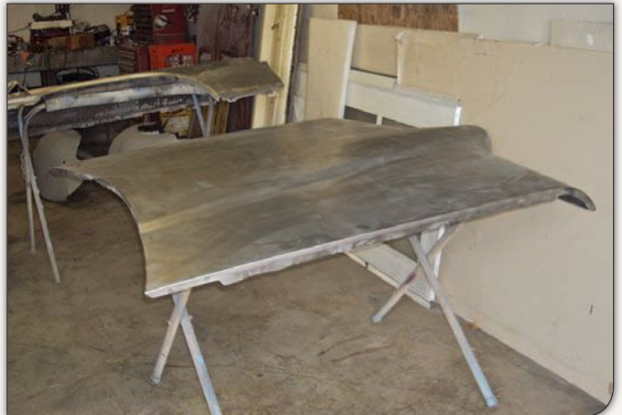
Bill says, "Though the hood was undamaged, the stamping was extremely uneven from the factory. The entire 'nose' area of the hood was sunken-in and needed to be filled to be perfectly flat and straight. It was a Herculean task for any restoration pro!"
