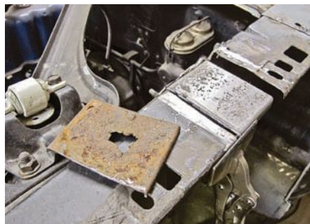
This 1967 Mustang convertible revealed the horrors of rust on closer inspection. Rotten, rusted metal is removed and replaced.
