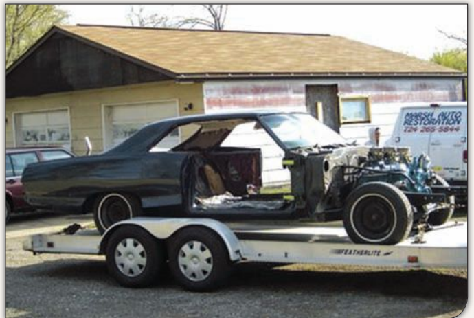
Once Kilkeary's Auto Body finished the paint, the Grand Prix was delivered to Marsh Auto Restoration for reassembly, panel alignment, wet sanding and polishing. Then the bumpers, grilles, lamp bezels, tail panel trim and taillamp lenses could be reinstalled.
