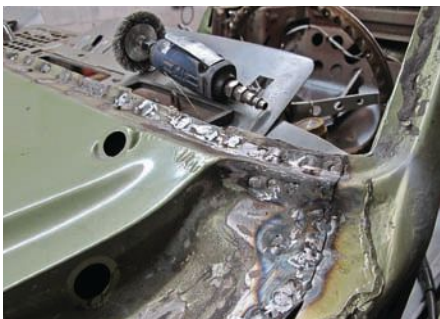
This 1967 Mustang convertible revealed the horrors of rust on closer inspection. Rotten, rusted metal is removed and replaced.
