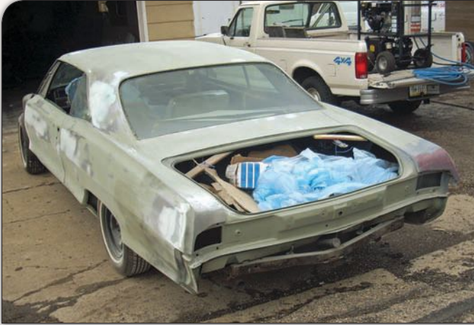
While completing the dent repair on the edges of the rear quarter panels, Terry worked in the end caps that Bill had purchased to replace the heavily damaged ones. Another rear bumper would also be sourced, as the original was too damaged to repair.
