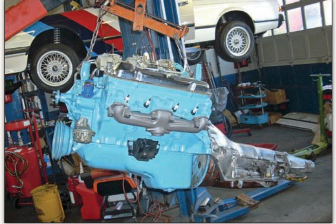
Renting a steam cleaner and employing Gunk Engine Brite to degrease the engine before painting, Bill then applied Bill Hirsch engine enamel over the bare iron. He used Eastwood cast-iron exhaust manifold paint on the manifolds, following sandblasting.
