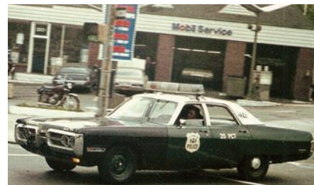
By 1972, the NYPD was experimenting with electronic warning systems. A Federal TwinSonic light bar adorns this Fury I.
