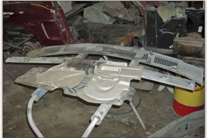
A great deal of time was spent ensuring that all the ancillary components were reworked as-needed to the quality level of the rest of the body. Smaller parts like the cowl grille panel can really detract from a restoration if they are poorly fitted and/or finished.
