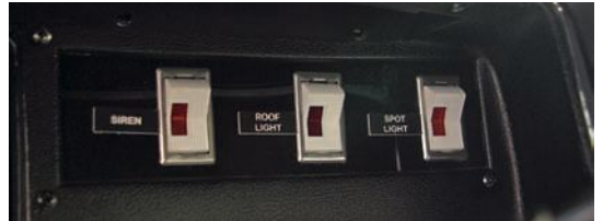
All this gear still exists if you know where to look for it. Telephone handsets were standard for NYPD radios. Switch panel allowed driver to activate siren with the horn buttons. Speedometer was salvaged from a Highway Patrol RMP wrecked during a Parkway pursuit.
