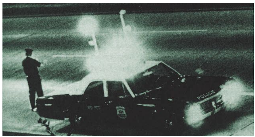
The middle 1960s saw the adoption of high-rise lights, hinged on either side of the roof, which could be swiveled upward for better visibility.
