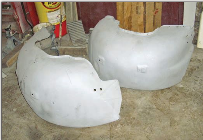
The underhood parts that should have a semi-gloss black finish were epoxy primed with Glasurit (shown) and then painted with Rust-Oleum Satin Black. Terry feels the appearance compares well with more expensive paints, and Bill says it's been durable.
