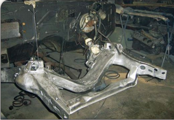
Using Scotch-Brite pads, John stripped down to bare metal the front portion of the frame, the steering box and suspension components. He then epoxy primed the frame and control arms and painted them with Rust-Oleum.
