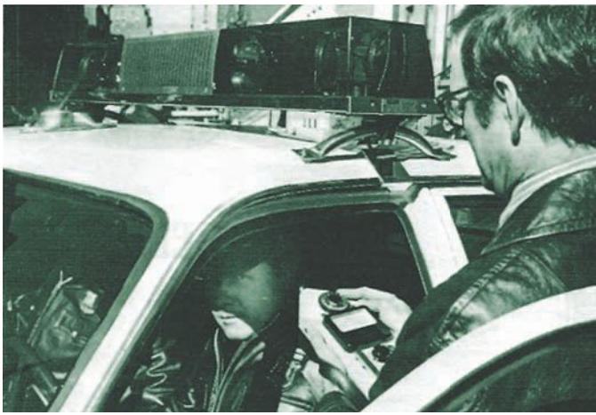
Patrol officers stand by as a 1972 RMP fitted with a TwinSonic warning setup undergoes electronic testing.
