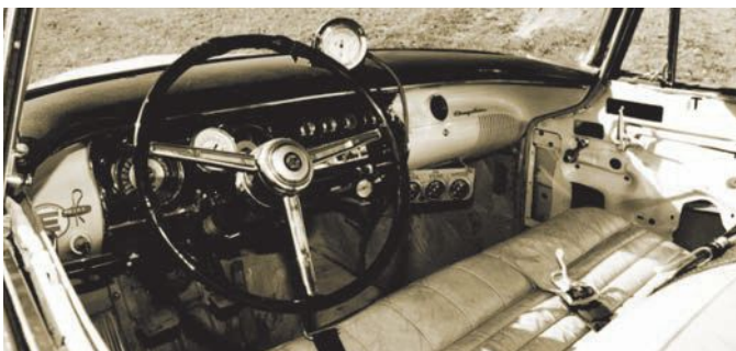
The NASCAR office in 1955. The interior is totally stock other than a few extra gauges and, uniquely, an onboard fire-extinguishing system. No side seat support, either.
