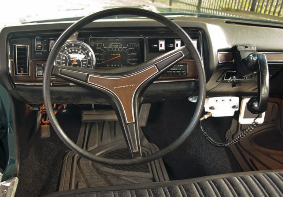
All this gear still exists if you know where to look for it. Telephone handsets were standard for NYPD radios. Switch panel allowed driver to activate siren with the horn buttons. Speedometer was salvaged from a Highway Patrol RMP wrecked during a Parkway pursuit.
