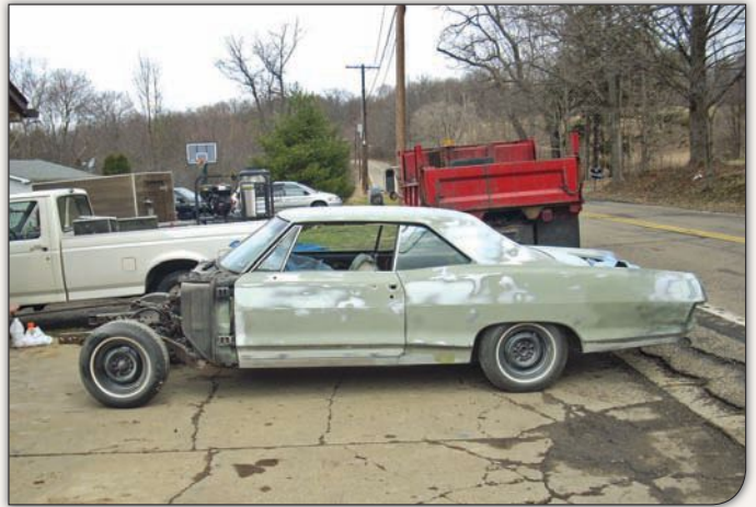
After applying the green-gray epoxy primer over the entire bare metal body, he used a thin coat of filler where needed and block-sanded. Bill Ballon says, "The quarter panel stampings were wavy, and given the prior damage, it made for a lot of work."
