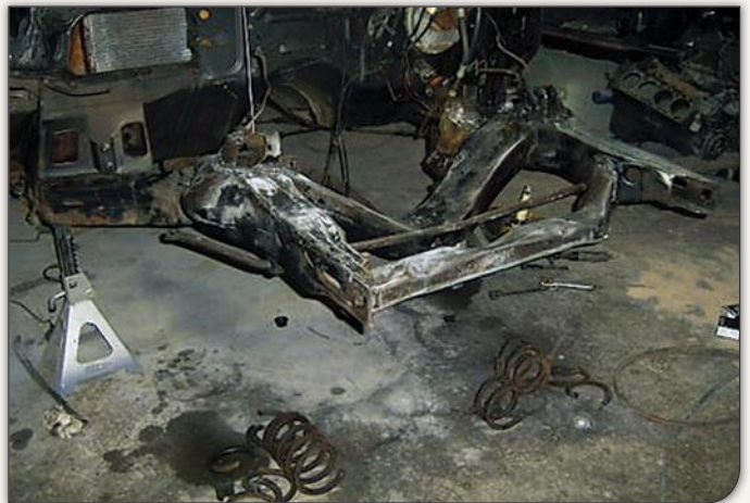
Suspension and steering components were removed and cataloged by John Marsh. The springs were simply cut, since they would be replaced. Bushings were pressed out of the control arms and the ball joints were removed, as the control arms were retained.
