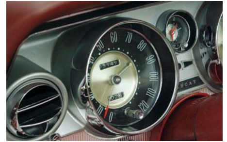
Adjustable ball vent, left of the speedometer, was only fitted to cars equipped with A/C.
