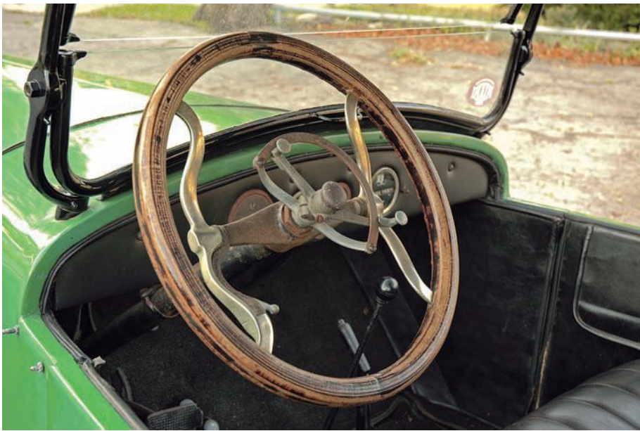
Early tilting wooden steering wheel, a.k.a the "fat man wheel," allowed for easier ingress and egress for the Model 51's driver. Padded instrument panel was a rather simple affair, including a Stewart speedometer/odometer and gauges for amps and oil pressure.
