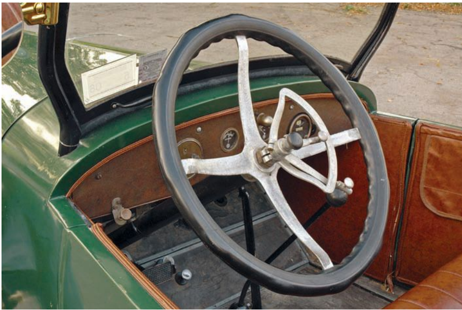
Davis changed little with the instrument panel from 1920 to 1922, with the same gauges available to the driver on the Model 71. Though this 1922 Davis does not have the tilting wheel, it continues to have the hand throttle and spark advance mounted on the steering column.
