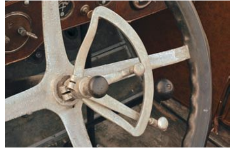
Davis changed little with the instrument panel from 1920 to 1922, with the same gauges available to the driver on the Model 71. Though this 1922 Davis does not have the tilting wheel, it continues to have the hand throttle and spark advance mounted on the steering column.
