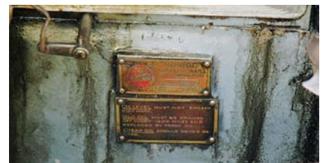
Billing itself as "America's Standard," Continental supplied its 38-hp 7R straight-six engine for use in Davis's 1920 Model 51. The 7R was a workhorse favored by many companies that assembled "component" cars. Engine plate warns that "Cheap oil should never be used."
