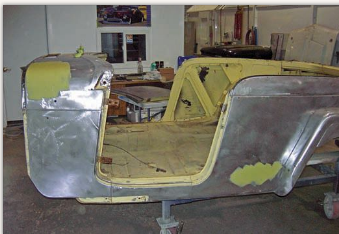
Something fell on the cowl while in storage—the other minor dent's cause is unknown. Once the metal was straightened, a thin coat of Evercoat Rage Gold body filler was applied, worked with a body file and block sanded with grades of paper up to 220.
