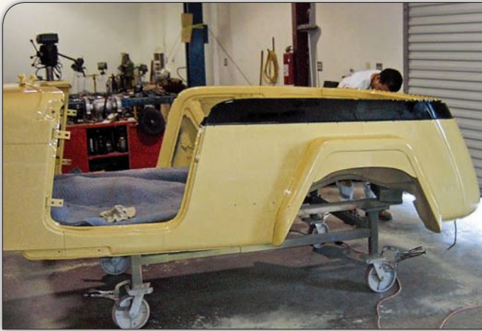
Three coats of Fiesta Yellow, in PPG's Delfleet Essential single-stage urethane enamel system, were applied. The paint was wet sanded using 1200, 1500 and 1800 grades of paper, then thoroughly polished to a mirror-like finish using 3M products.
