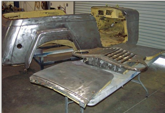
The outer shell and bolt-on body parts were media blasted, but the inner shell and the inner doors would be sanded prior to repainting. Note the overall lack of damage on all the parts—a testament to the care the Jeepster had received since 1949.
