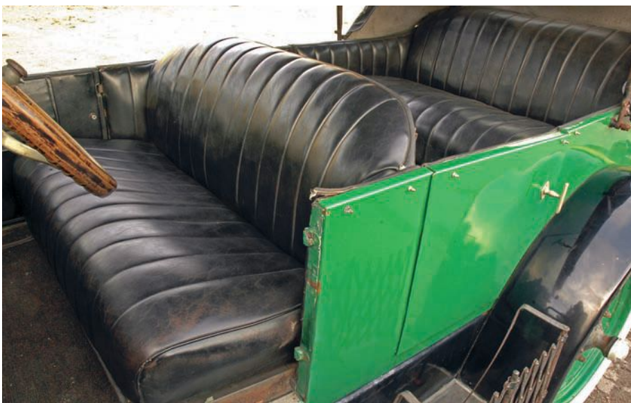
There was nothing unusual about the Model 51's five-passenger touring body, composed of metal panels over a wooden frame, though its Disteel wheels were typically found on more expensive cars; removable, collapsing luggage rack was a common period accessory.
