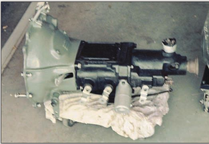
The rebuilt three-speed transmission with overdrive was detailed in black with a gray bell-housing prior to reinstallation. Jim feels that the engine, bell-housing and transmission may have all been painted black at the factory, but he hasn't been able to confirm it.
