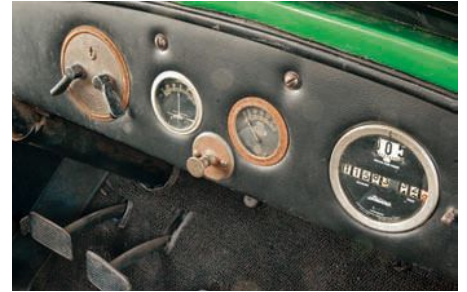
Early tilting wooden steering wheel, a.k.a the "fat man wheel," allowed for easier ingress and egress for the Model 51's driver. Padded instrument panel was a rather simple affair, including a Stewart speedometer/odometer and gauges for amps and oil pressure.
