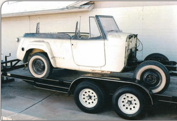
With the bumpers, front body panels, interior, convertible top and frame, engine and transmission removed, the Jeepster was loaded on a trailer for delivery to the body shop. The body and paintwork would take just four months to complete.
