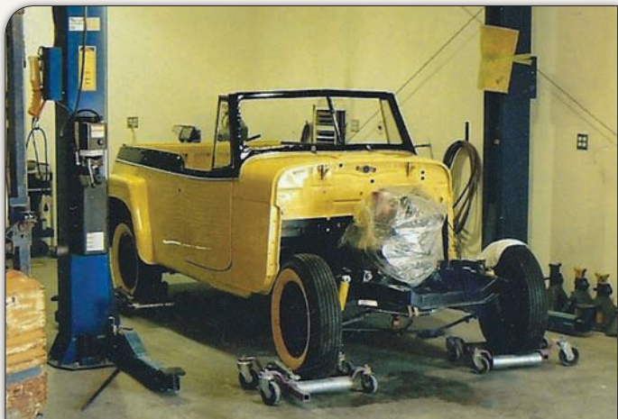
He delivered the chassis with the engine and transmission reinstalled. The body was lowered onto the frame with 24 new rubber mount bushings in place, and most of the body bolts were installed to secure it. He completed the job once the Jeepster was home.
