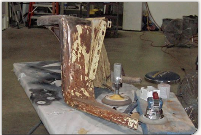
In general, the front fenders, grilles and hoods are mostly interchangeable between the station wagons, trucks and Jeepsters, but body panels from the firewall back are body-style specific. Fortunately, solid steel was under this fender's surface rust.
