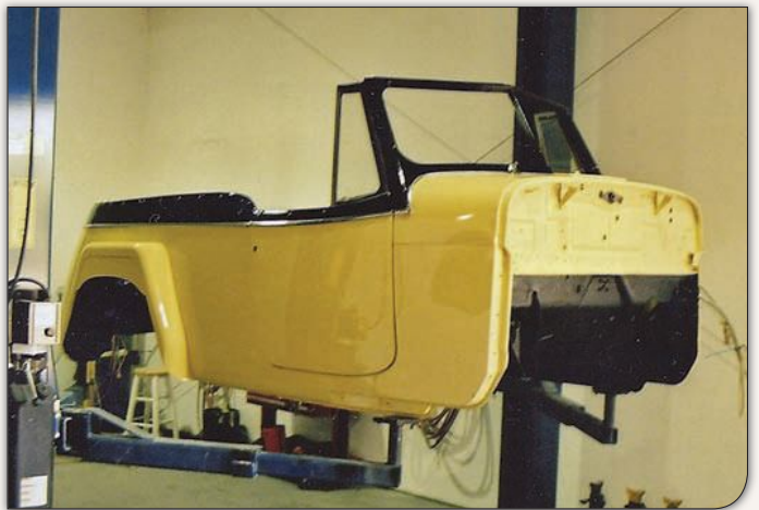
Once the bodywork and paint were completed, the shell was moved to the lift in preparation for being reunited with the chassis. Jim had taken the chassis home to restore it and had sent out the transmission for a rebuild and the engine to be inspected.
