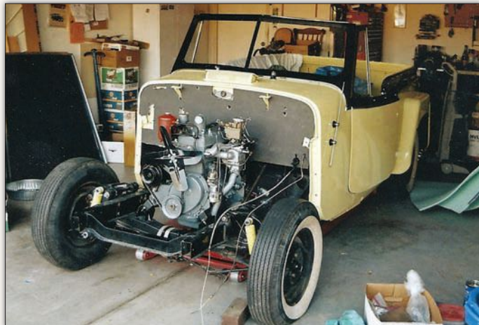
With engine unwrapped, its cosmetic detailing is revealed. The block was painted gray, and the accessories are black. It's possible that black is correct for the engine, however. Jim says that the orange oil filter canister with black top is factory-correct.
