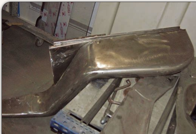
Like the rest of the body, this passenger-side front fender was rust-free. Since few reproduction body parts are available, if this fender had required replacement, Jim would've sourced a used one from one of the other models previously mentioned.
