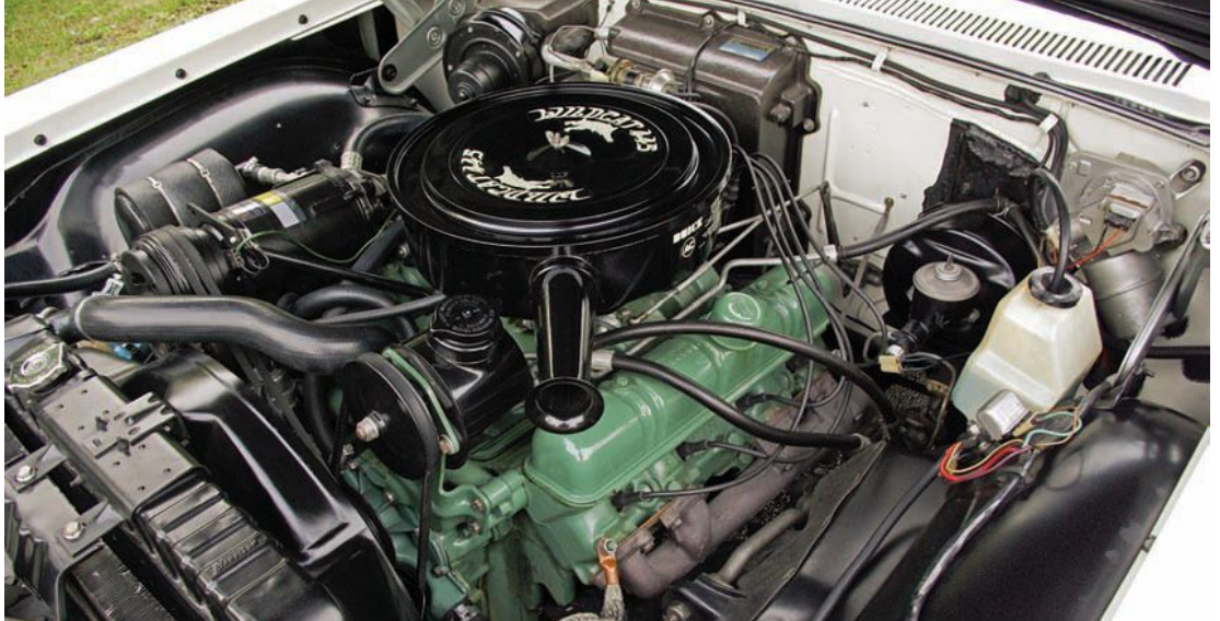
Called the "Wildcat 445" for its torque rating, the 401 nailhead V-8 pushes out a mighty 325 horsepower.
