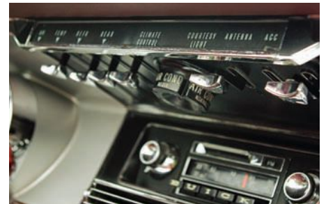
Aviation-style switch panel regulates climate control, courtesy lamps and antenna.
