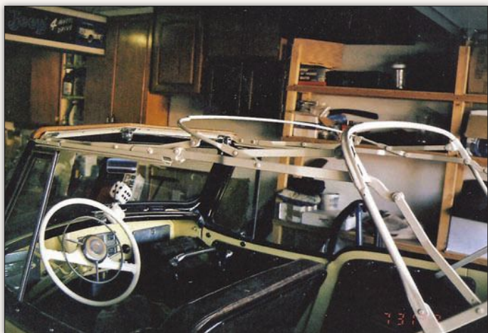
He reinstalled the convertible top frame, featuring oak top bows and a tack strip from Paul Barry at Willys America in Cazadero, California. However, like the body and paintwork, he concluded that making a convertible top from scratch was best left to a pro.
