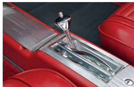
Console-mounted tach isn't in the best location; trunk release button is in the glovebox. The "P-N-D-L-R" alongside the shifter signifies car is fitted with the Twin Turbine transmission.
