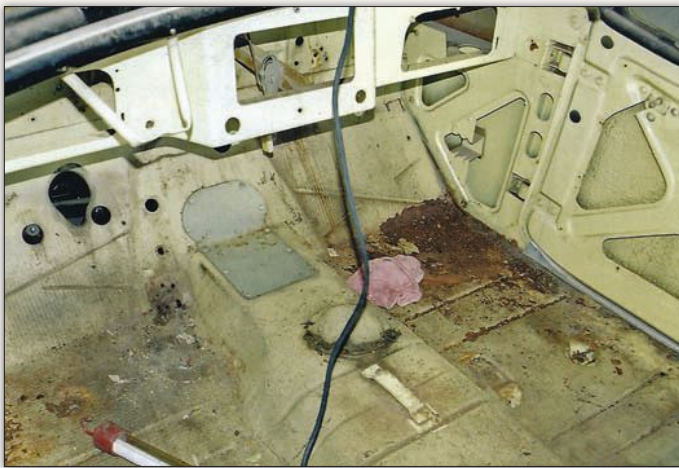
The passenger-side floor is one of precious few areas to reveal rust. Thankfully, it was only minor surface scale that was easily removed when later sanded to bare metal. No holes were found, so the entire area was easily primed and repainted.
