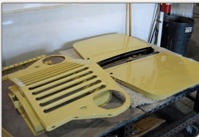
Before the color coats were applied, two coats of PPG ESU461 Epoxy Primer were applied over the body and block sanded with multiple grades up to 220. Then PPG ESU440 High-Build Primer Surfacer was sprayed and block sanded with multiple grades up to 320.
