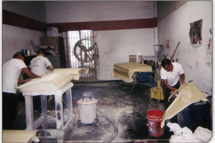
Once the primer dried and cured, it was time for extensive block sanding using progressively finer-grade paper, until everything was ready to return to the paint booth for final finishing.
