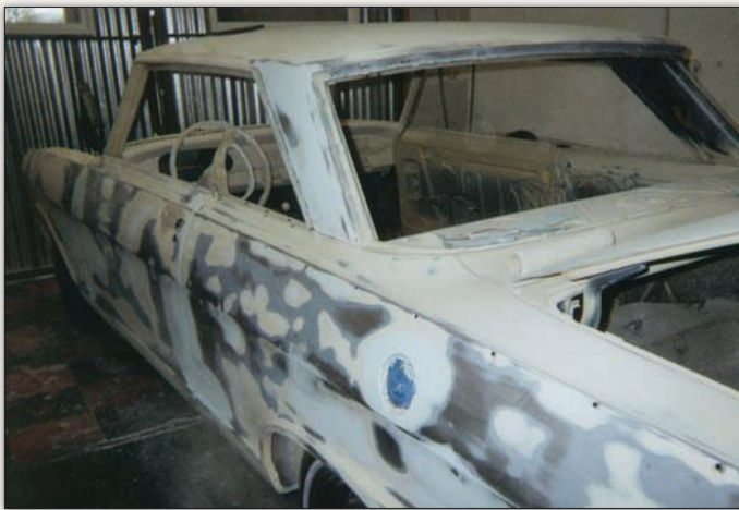
A small amount of body filler was applied and sanded flat prior to the catalyzed epoxy build primer coat; the body filler is light blue, and the build primer is light yellow. Note the extensive masking job on the steering wheel and interior.
