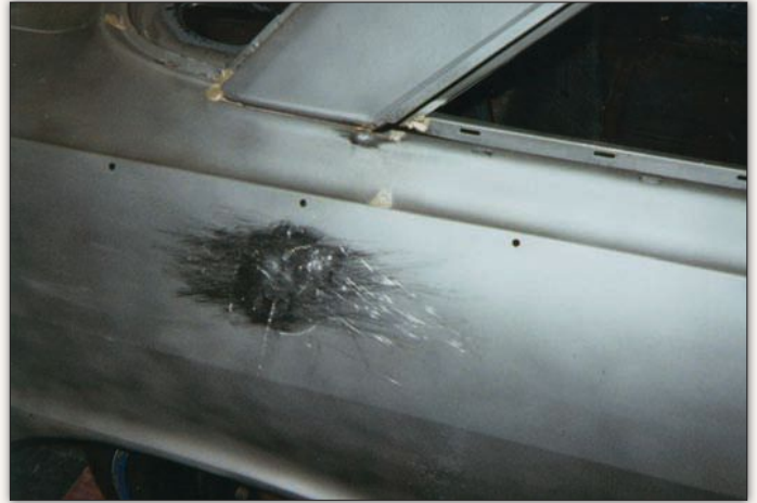
A former shopping cart dent in the sheetmetal was spooned and smoothed back to factory flat before any primer or paint was applied. The repair weld below the C-pillar was made to fix a common spot for stress cracks on 1964 Chevy II Novas.
