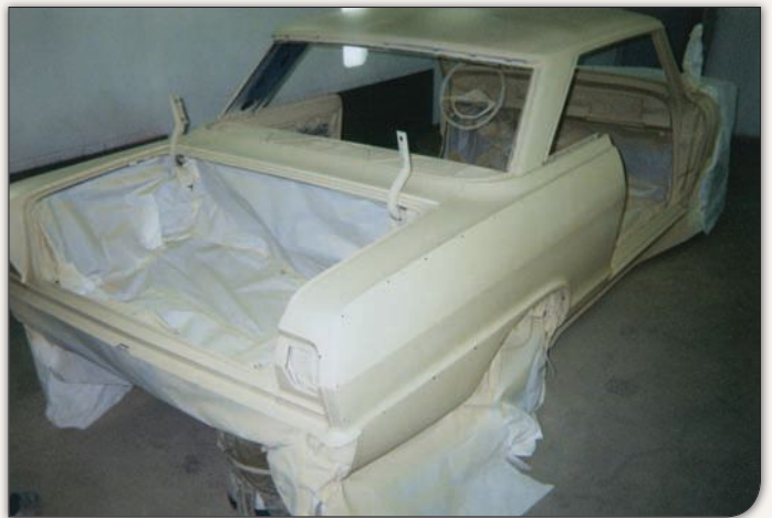
Sanding of the body filler and light coats of primer were followed by a full wipe down with paint prep. A heavier coat of build primer was applied and allowed to cure before block sanding to bring the body panels back to factory perfect.
