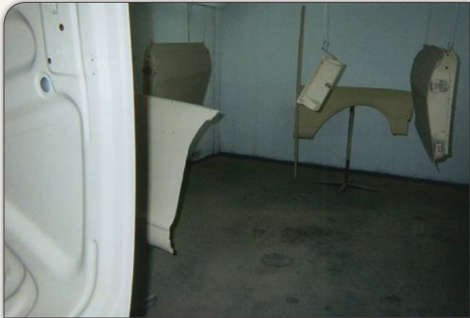
Here, the trunk deck, glovebox, fenders and doors are carefully hung inside the paint booth after getting their own bodywork, filler, sanding and epoxy-build primer coats. Paul wanted the Nova thoroughly painted inside and out.
