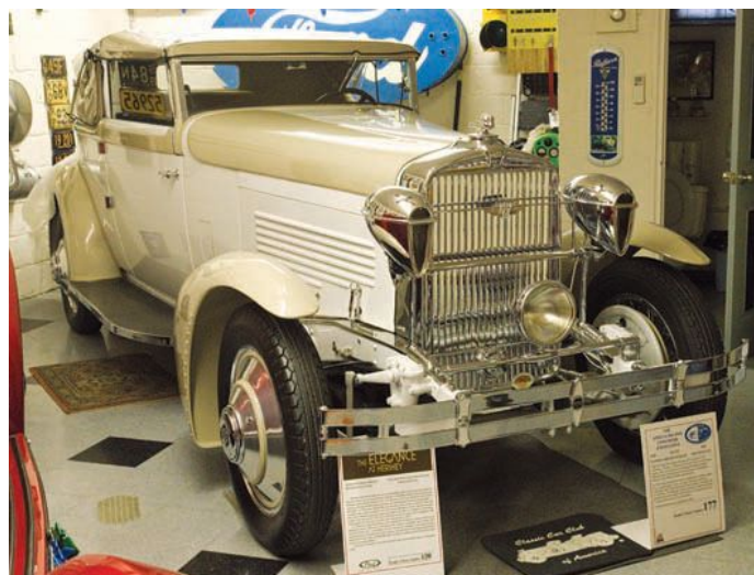
This coachbuilt Stutz represents some of the earliest uses of bobbed fenders as a styling feature on any automobile.
