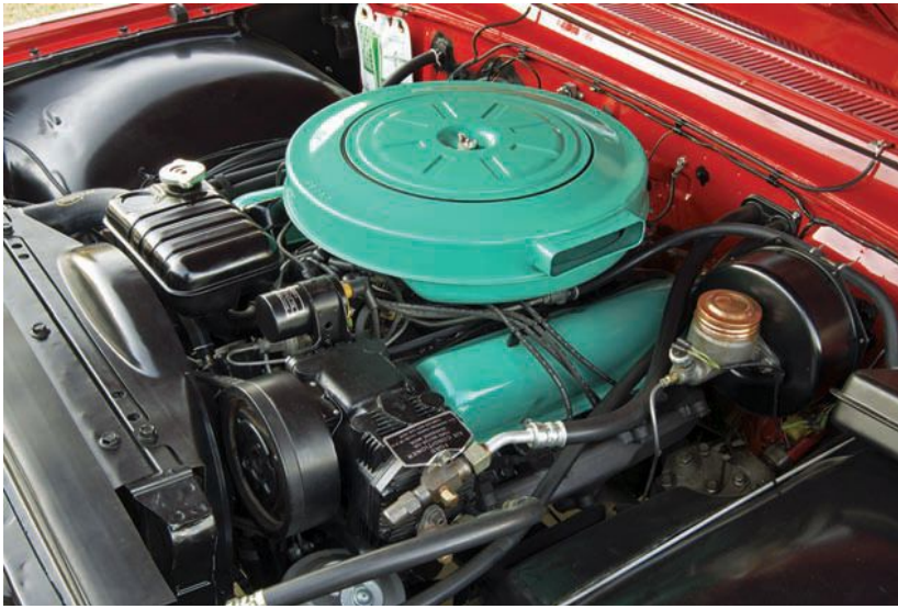
Although an Economy Six was available on other Edsels, the convertible's sole powerplant option was the Super Express V-8, a 352-cu.in. engine with a higher compression ratio than the Ranger V-8, making 300 hp and 381-lb.ft. of torque.
