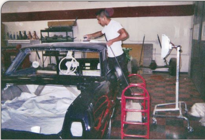
The lead painter is shown here finish-cutting the roof prior to the finish-buffing procedure used to bring back the luster of the Daytona Blue enamel that was lost due to years of California sun and unfriendly environmental elements.
