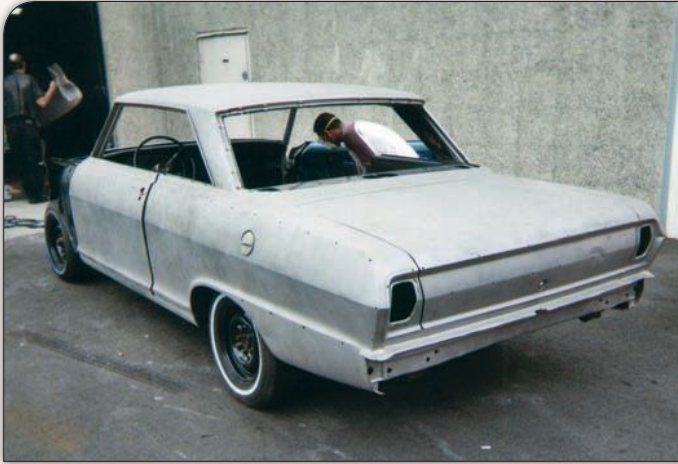
The body was stripped of existing paint and primer using the walnut shell blasting method. All the original sheetmetal miraculously survived well, despite decades of driving, thanks to the old-car-friendly California desert climate.
