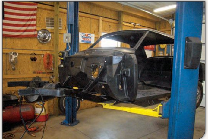
After media blasting, the body shell, panels and frame were given a coat of epoxy sealer to prevent the metal from flash-rusting before final prep, primer and paint could be applied. Note that the front suspension has been removed.
