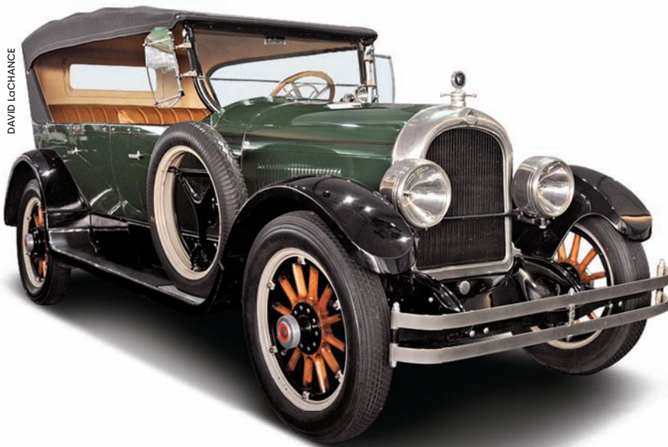
This 1924 Model 34 was one of the last of the series, as consumers began perceiving straight-eight engines as more luxurious than the Model 34's straight-six, despite the Marmon's power and speed.
