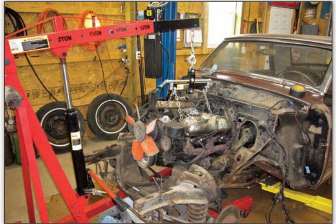
After a second, more thorough assessment of the Gran Turismo, it was determined that a show-quality restoration was the best course of action. Here, the front end has been disassembled, making the task of removing the engine significantly easier.
