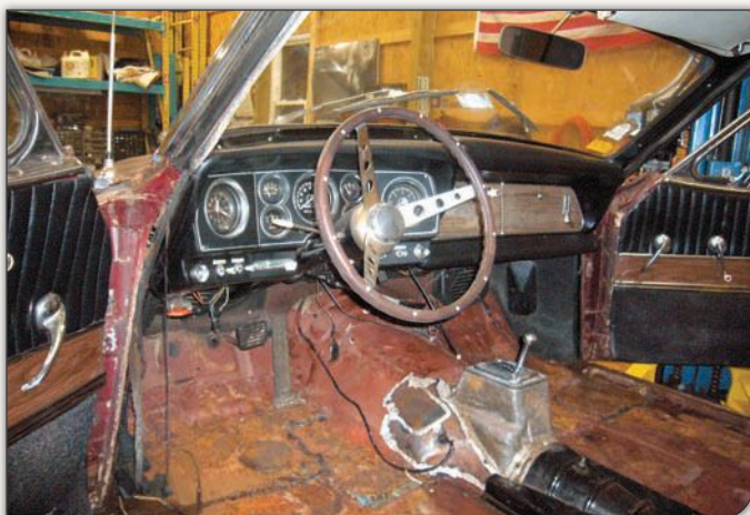
Making repairs to the transmission hump was a difficult process because of the tight fit for the center console and automatic transmission shifter. A parts car in the family inventory of Studebakers donated the necessary metal to expedite the repair.
