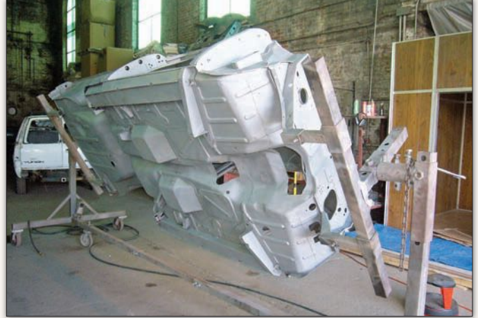
The frame was not the only part subjected to media blasting. All of the removed body panels, and the body shell seen here, received the same careful cleansing, which revealed a few more minor areas of corrosion that would need to be repaired.
