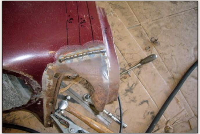
Damage from rust on each fender’s lower extremities was minimal; however, patches still had to be fabricated and butt-welded into position. Lines scribed on the paint are dimensional reference points, and the welds were eventually ground smooth.
