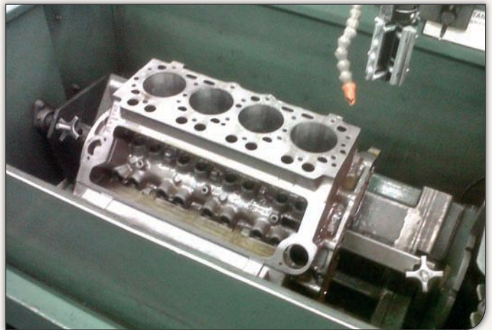
The V-8 was then completely disassembled and brought to a local NAPA outlet that had its own machine shop. Closer inspection by the staff revealed no significant issues, and a .030-inch overbore was performed to ensure that the cylinder bores were perfectly round.
