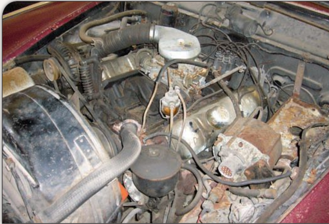
As found, the 289-hp, 289-cu.in. Studebaker R2 engine was complete, though the Paxton supercharger had been removed and stowed in the trunk. The engine's internals would turn; however, it was incapable of running.
