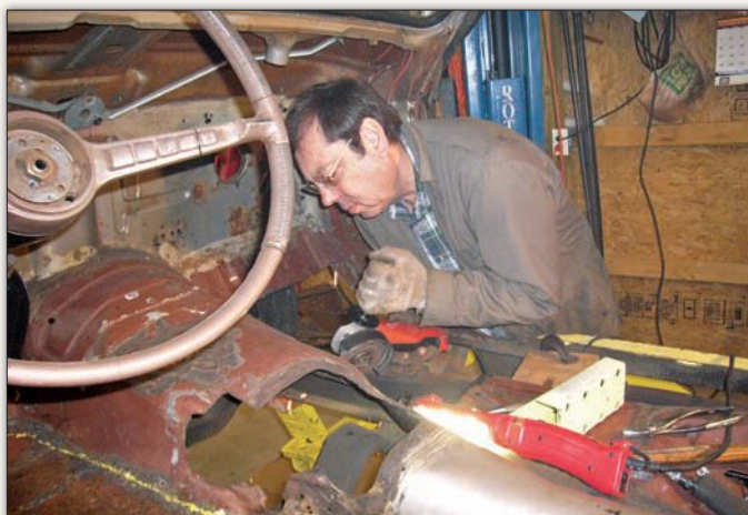
Peter made several visits to assist with many aspects of the restoration project, including metalwork. Here, the passenger side floorpan has been cut from the body, and Peter is using an angle grinder to smooth the rough cuts.
