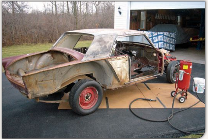
By the time the first round of metalwork was completed, the body had been stripped to its basic shell, which was then separated from the frame for a closer inspection of the mounting points before they were loosely reunited and sent for media blasting.
