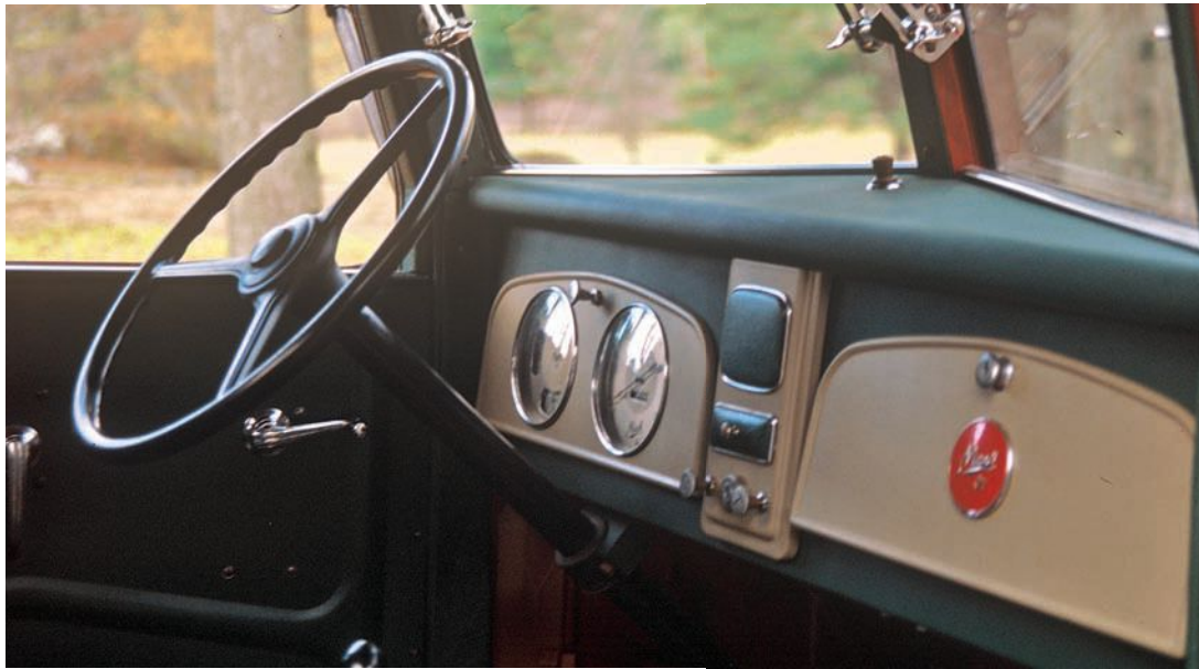
Two large, light gray-faced gauges with their chrome bezels contrast nicely against the green instrument panel.
