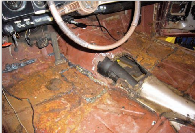
Although the floors seemed solid upon first inspection, when the carpet was removed poorly executed repairs made by a previous owner quickly became apparent. The transmission hump had also been badly cut to permit installation of a three-speed manual.
