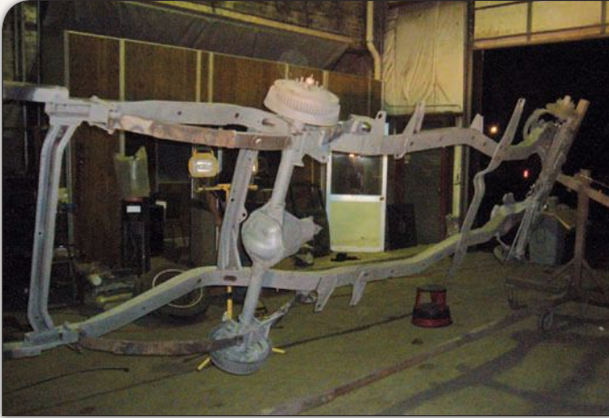
With only the underpinnings required to aid mobility left in place, the Hawk's frame was media blasted, leaving nothing but bare metal behind. In spite of some of the metalwork required to repair the body, the frame was devoid of corrosion damage.
