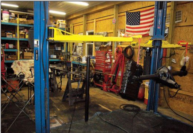
This is an example of how to make the most of the tools available to you during a restoration. Rather than create temporary space, the two-post lift in Matt's garage has been employed to hang and paint many of the chassis and suspension parts.
