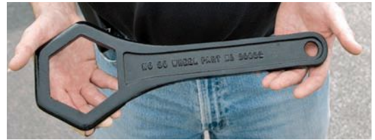
Original—and still intact—tool kit includes this massive lug wrench for the removal of the wire wheels.
