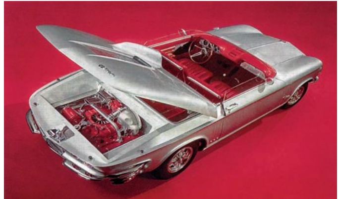
"Exciting" is one way to describe the Corvair Super Spyder concept. Notice the cut-down, frameless windshield and side window glass.
