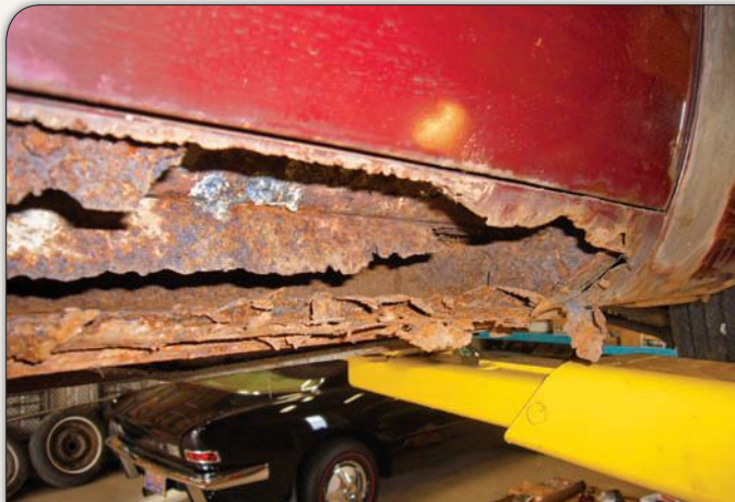
A wide band of brightwork typically covers a Hawk's rocker panels, which then disintegrate while hidden from view—a common plight. The damage here is extensive but manageable when done correctly with reproduction panels.
