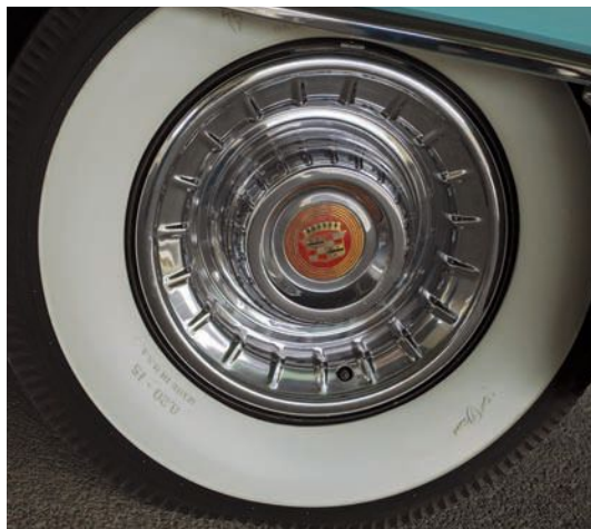
Cadillac's very distinctive Sabre wheelcovers for 1956 had fewer "spokes" than the 1955 version, with a deeper contour between the hub and outer edge.
