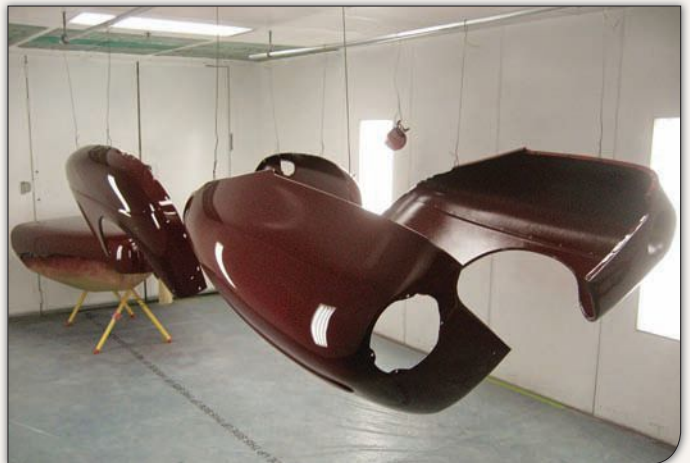
After block sanding, three top coats of Glasurit paint were applied, in this case in the proper shade of Ford Dynamic Maroon, followed by four coats of Glasurit clear. The new paint was eventually wet sanded and buffed thoroughly to bring out the best in the finish.
