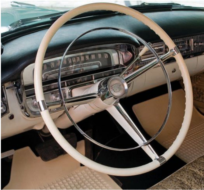
Steering wheel's color matches lower instrument panel and features a large chrome horn ring, with a good view of the speedometer. Glovebox is centrally located, and the Gold Bombay patterned metallic nylon upholstery was combined with white leather.
