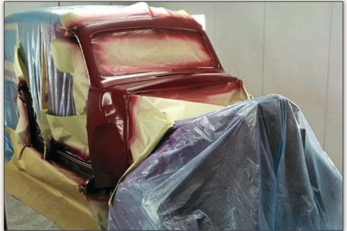
With the radiator installed and some other reassembly complete, the main body was refinished in preparation for final assembly. The wood required little work, owing to its excellent condition and some spot restoration from a few years back.
