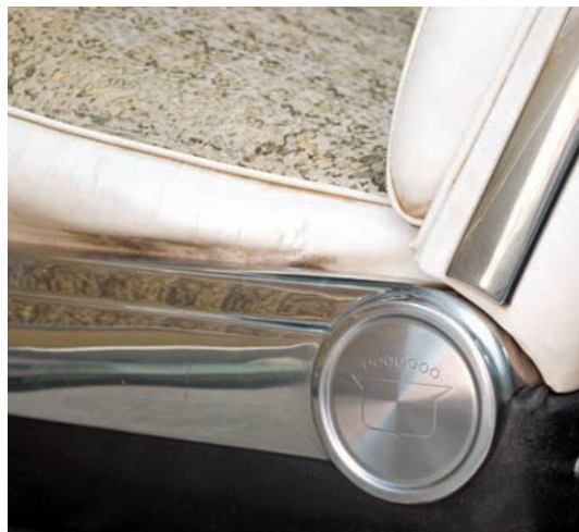
Lots of well-executed quality details can be seen throughout the interior, including the front-seat hinge cover embossed with Cadillac's signature crest.
