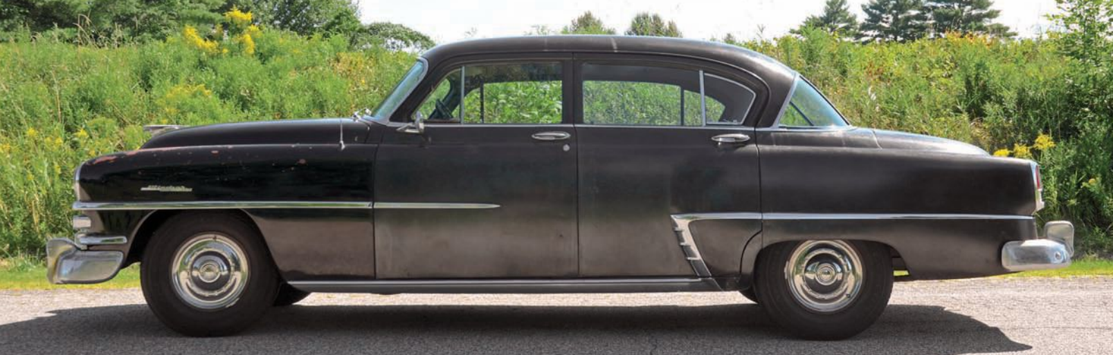
The Windsor DeLuxe shows off its full 211 inches of length in profile. The longer rear fenders for 1953 add to the overall effect.
