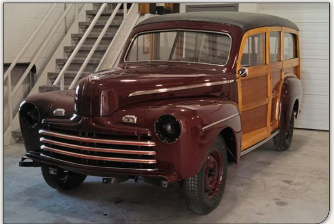
Awaiting the return of the last few chrome bits, the Ford sits ready for final assembly. Note the excellent condition of the unrestored wood, which required only some spot re-staining and re-shellacking, using a pre-mixed shellac.
