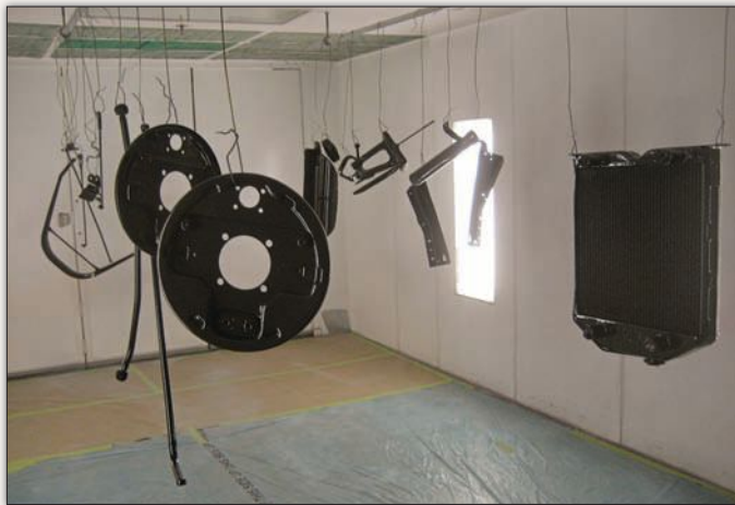
Partial disassembly allowed the restorers to clean and restore chassis and underhood components as necessary, which included the standard semigloss black treatment for those hidden parts.
