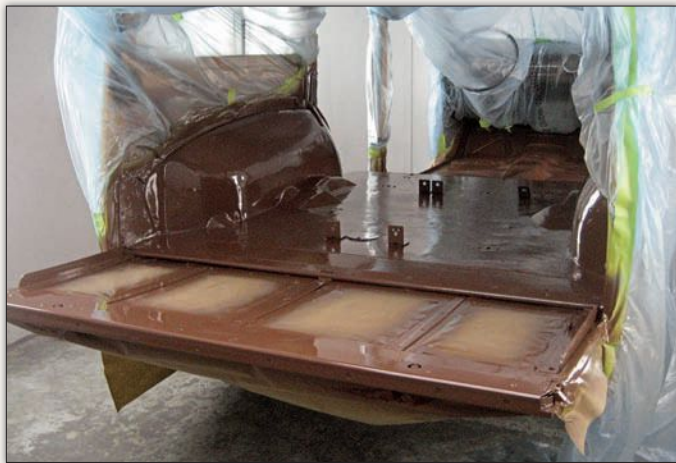
With the seats removed, the interior, too, was treated to a new finish. With the floor pan stripped to bare metal, and after using the PPG DP40 primer, a single-stage enamel was applied, in this case in the correct Ford Maple Leaf Brown color, as original.
