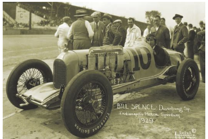
Straight-eight-powered cars were notable for their aerodynamic narrowness in 1929, such as Bill Spence's Duesenberg.
