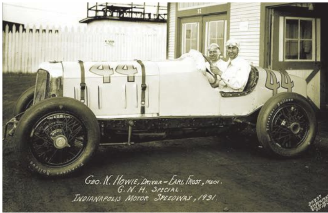
George Howie built this unusual car himself for 1931. It was a Dodge chassis stuffed with an eight-cylinder Chrysler.
