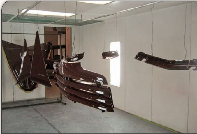
In addition to the removable fenders, the hood, grille and other related body components got the same treatment in removing old paint, filler and surface rust before refinishing with three coats of color and four of clear.
