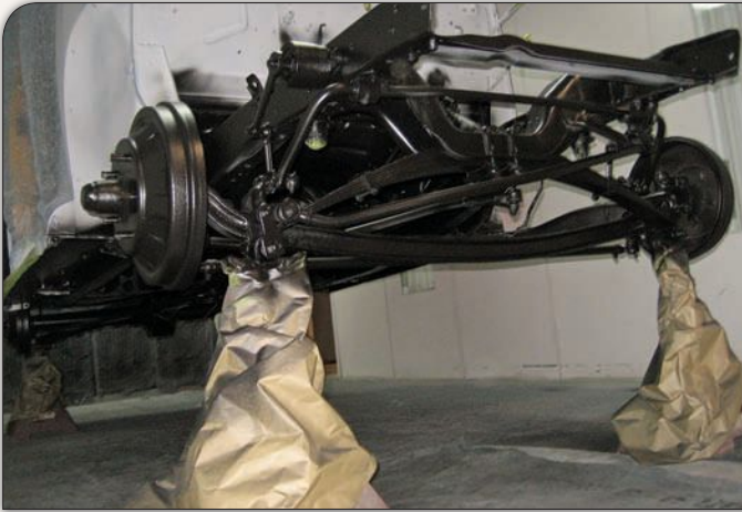
As they do on most frames of this vintage, CB Restorations used one coat of unreduced PPG DP40 epoxy primer and two coats of Sherwin-Williams Polane Semi-Gloss Black to refinish the woodie's frame, completing the job without removing the body.
