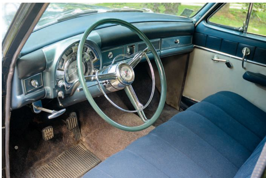
There is no lack of head or legroom up front. The odometer and speedometer are surrounded by amperage, fuel level, oil pressure and coolant temperature gauges. Temperature controls are flanked by fan and defroster knobs.
