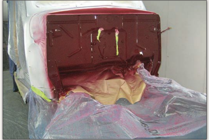
With the chassis complete and body primed, the firewall received the first final coats. After primer, that was three coats of maroon followed by clear. As the firewall would not get the same final wet sanding as the exterior, it got two coats of clear instead of four.
