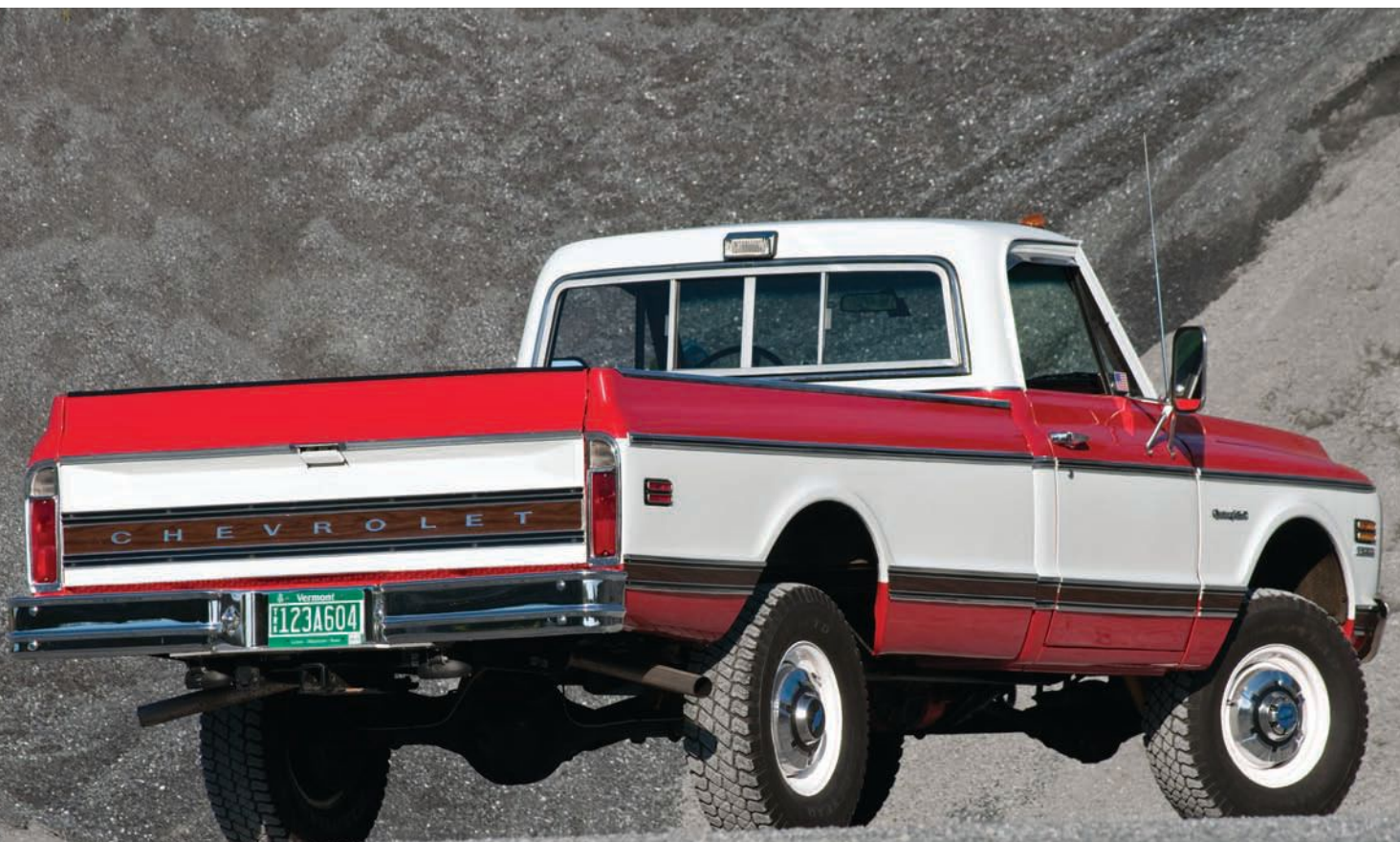
The truck's hubcaps look stock, but they're from a 1973-vintage Chevrolet pickup. The front caps are rear units with the centers removed and the inner lip rolled over for a factory appearance.
