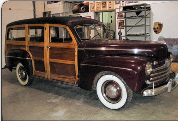
When it arrived at CB Restorations, the Ford was in relatively good shape, a mix of previous work and largely preserved originality. Both the interior and exterior wood required very little work, and none was removed from the car during the restoration.
