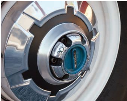
The truck's hubcaps look stock, but they're from a 1973-vintage Chevrolet pickup. The front caps are rear units with the centers removed and the inner lip rolled over for a factory appearance.
