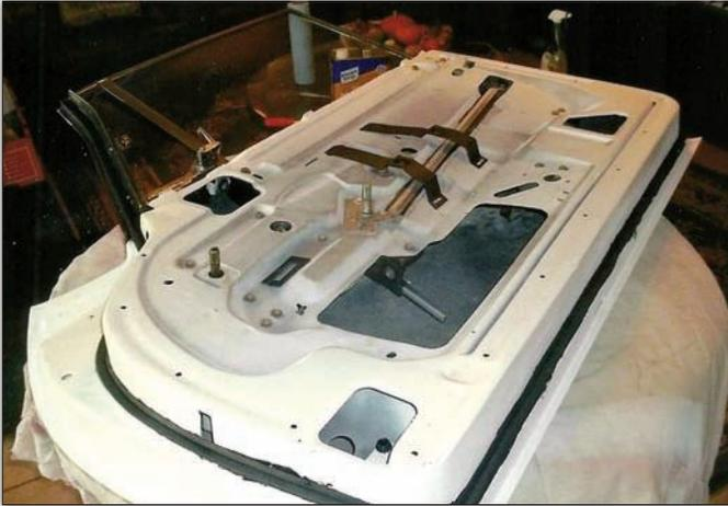
Each door's window operating system was refurbished and then reinstalled with new glass run channels and inner and outer door whiskers. The interior of the doors was sandblasted, wiped with Ospho, sprayed with two coats of epoxy primer and seamsealed.
