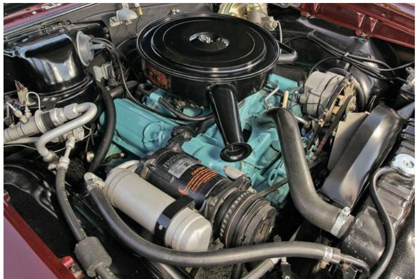
The original 326 H.O. V-8 engine was bored .030 over and upgraded with a longer-duration camshaft and a 650-CFM carb during its rebuild.
