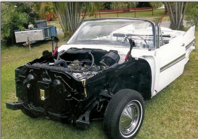
After the body was painted and the engine and transmission installed, the radiator was bolted to the chassis along with both inner fenders. This allowed the radiator to be installed and hoses to be connected to the engine, along with the horns and hood hinges.
