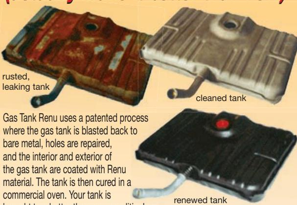
rusted, leaking tank      cleaned tank      renewed tank
