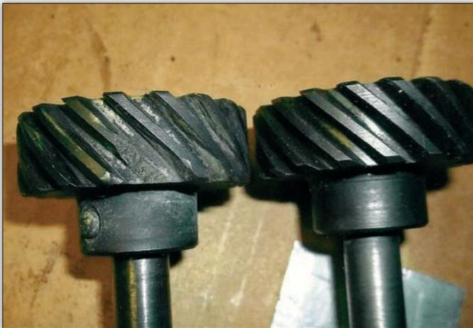
A new oil pump and distributor driveshaft, which is gear-driven by the camshaft, was installed because the original gear had several broken teeth. An NOS shaft and gear assembly was found at Len Dawson's Deception Pass Auto Parts in Washington state.
