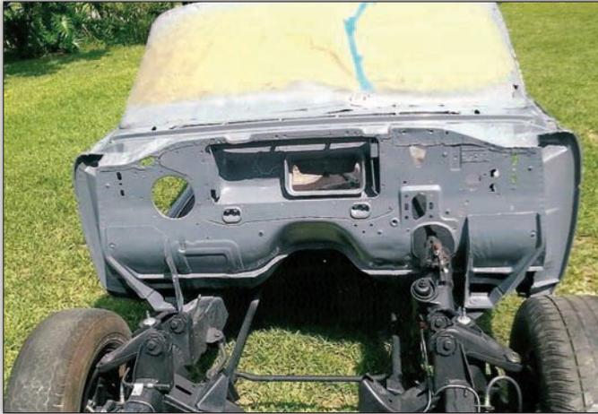
After the body was bolted back on the frame to have the replacement floor pans precisely aligned, it was lifted off again in order to be sprayed with a single coat of Eastwood's Encapsulator Epoxy, followed by two coats of urethane primer/sealer.
