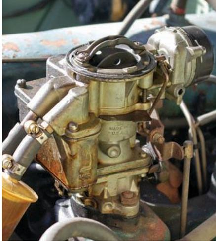
A single one-barrel Carter YF carburetor has proven more than adequate to feed the Gremlin's base inline-six engine.
