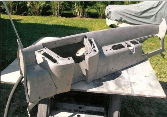
After the instrument panel had been removed and all the knobs, switches and wiring had been taken off, it was sandblasted down to bare metal using 30-grade media abrasive. After a second blast using finer 60-grade media, it was primed and painted.
