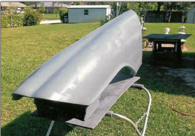
Both front fenders, doors and hoods were refinished separately. Just a few small spots required a thin layer of lightweight body filler, followed by a coat of light gray epoxy primer, then two coats of primer/sealer. All the painting was done by Richard.
