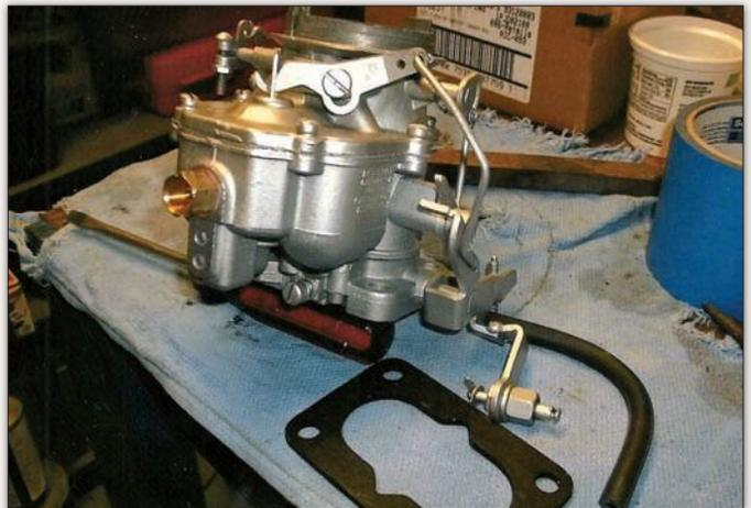
The replacement engine had a two-barrel intake, so Richard decided to keep it and buy a used two-barrel carb instead of switching to a four-barrel set-up. He now regrets that, due to the two-barrel's poor gas mileage. It was rebuilt prior to installation.
