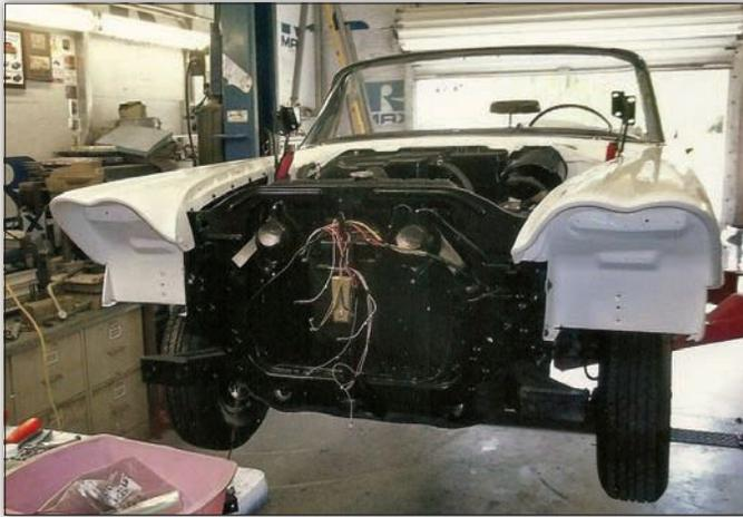
This is the period during a restoration when progress slows down, because you need to take extra care in bolting the restored components back in place without damaging them or chipping the new paint. With the fenders on, next came the headlamps and grille.
