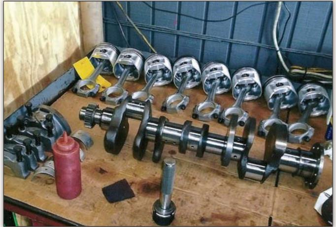
The replacement 318-cu.in. V-8 engine was sent to Lake Park Auto Machine Shop in nearby Lake Park to be machined and rebuilt. The block was bored .030-over and fitted with new pistons; the crankshaft was cut .010, polished and balanced for smooth operation.
