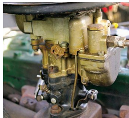
Oldsmobile's 238-cu.in. straight-six was standard in the Special 66 series. With a Carter single-barrel carburetor, it was rated for 100hp in stock configuration.
