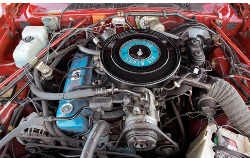
Optional two-barrel, 145-horsepower, 225-cu.in. Slant Six engine is one step up from the standard one-barrel version; fender tag is full.
