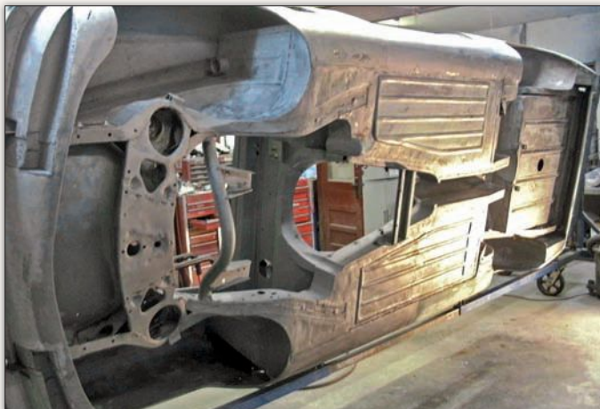
Once the entire body was media blasted—and also chemically and mechanically stripped—it was put onto the rotisserie for metal and bodywork. This view clearly shows the hybrid nature of the Dual-Ghia's body components welded to the modified Dodge frame.
