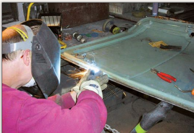
Unlike the original, which was gas welded, a new outer skin gets MIG welded to the inner skin and structure of the decklid, repairing rust and fixing some inferior work done decades ago after collision damage.
