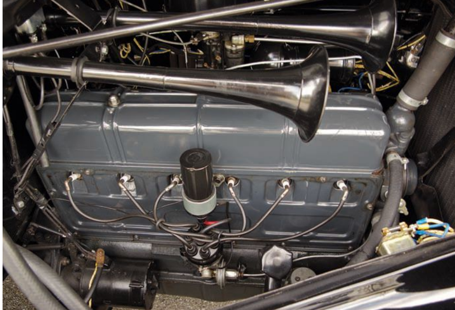
Ken rebuilt the 216.5-cu.in. six-cylinder engine and detailed the engine bay. Note the prominent placement of the City and Country horns.
