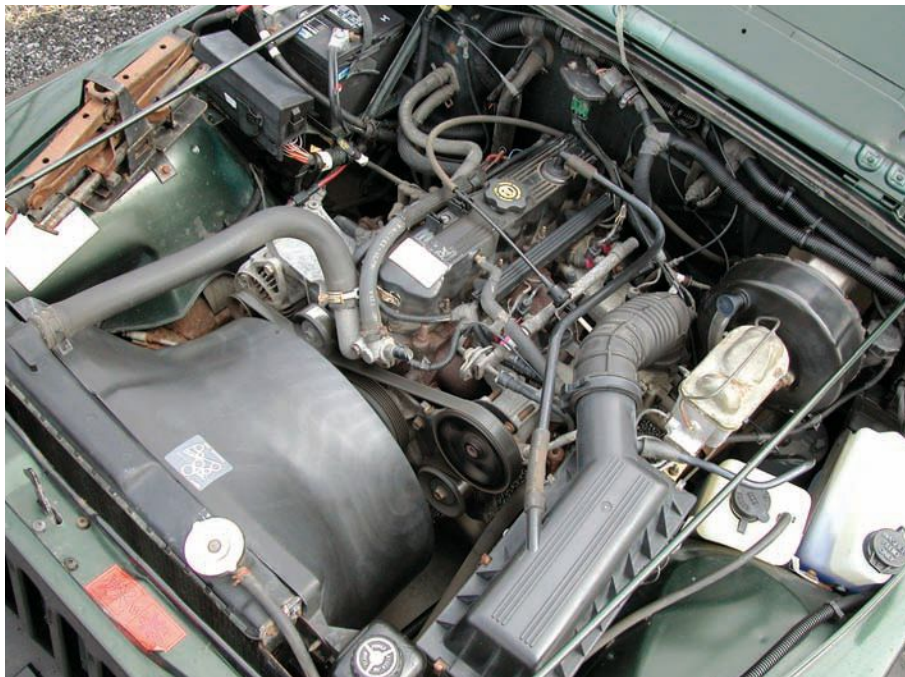
This Jeep was built under the corporate umbrella of the Chrysler Corporation, but its 150-cu.in. inline four-cylinder is an AMC design. With multi-point injection, it made 123hp.
