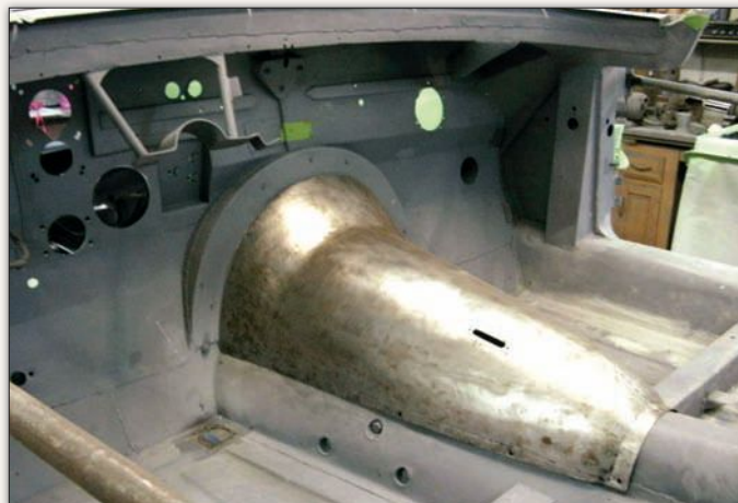
Like every other existing metal component, the transmission tunnel was also stripped of its previous finishes. Note the slot in the panel where the PowerFlite automatic transmission's shift lever attaches to the transmission.
