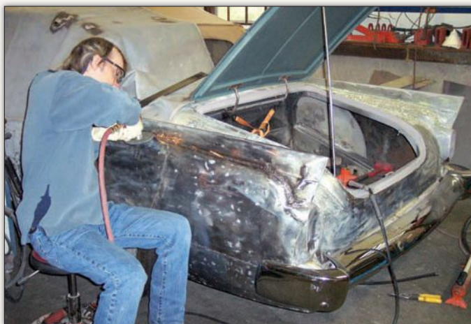
With the back bumper in place for fitment and guidance, a large, new piece of steel was welded into place in the quarter panel; here, the welds are being smoothed out before the first treatment of body filler to replace the factory's lead work.
