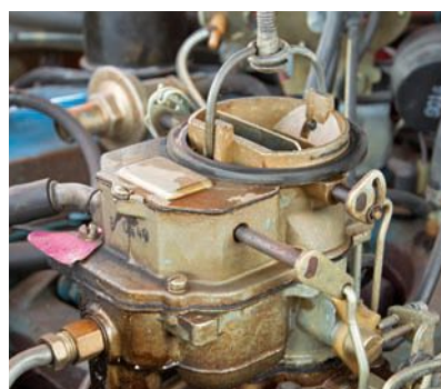
Optional two-barrel, 145-horsepower, 225-cu.in. Slant Six engine is one step up from the standard one-barrel version; fender tag is full.
