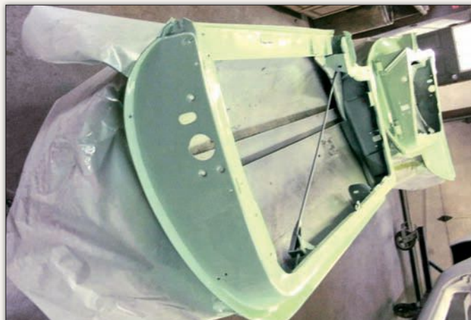
Note the threaded rod inside the door. Those rods were installed by the workers at Ghia, nearly 60 years ago. With every panel for every car handmade, those skilled coachbuilders would make fine adjustments by twisting the rod to get the doors to fit right.
