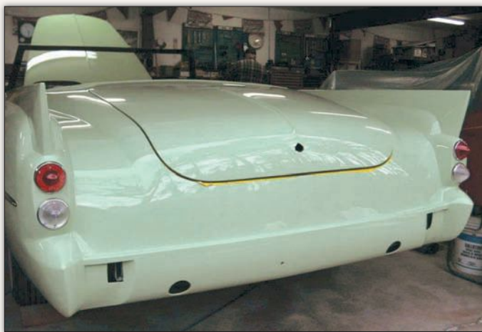
Here is the repaired and finished deck-lid and rear of the car before the complete trim and hardware has been installed. The intersecting curves and lines of the Dual-Ghia's fins and quarter panels would have been impossible to create on an assembly line.
