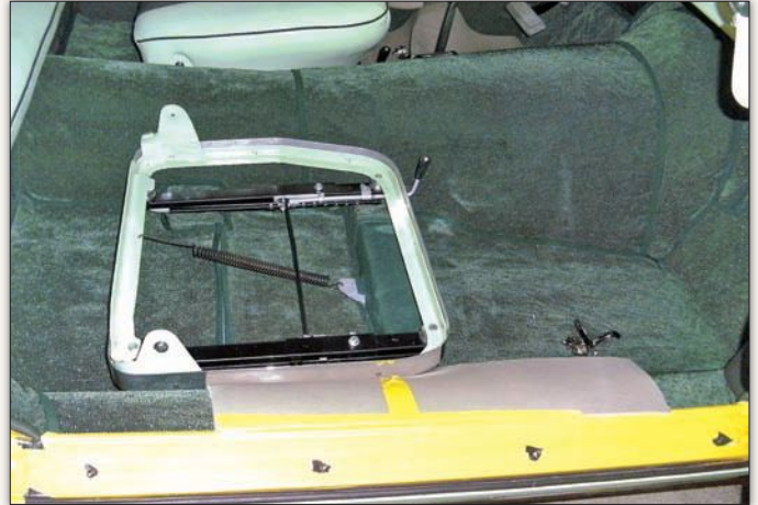
Before rebuilding the seats, Whitehall also painted the stripped-down frames in the same shade of Vermont Green. The carpet, with its unique pattern and color, was from a supply of 1956 NOS Chrysler material, making the entire color scheme complete.
