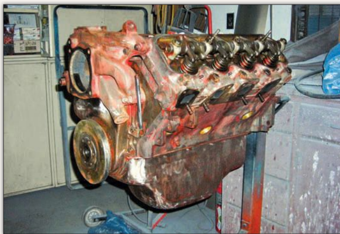
Though roughly half of all Dual-Ghias were equipped with Hemi V-8s, this car still features its original polyspheric combustion-chambered Dodge 315-cu.in. engine, rebuilt by the technicians at Whitehall before it was reinstalled in the restored car.
