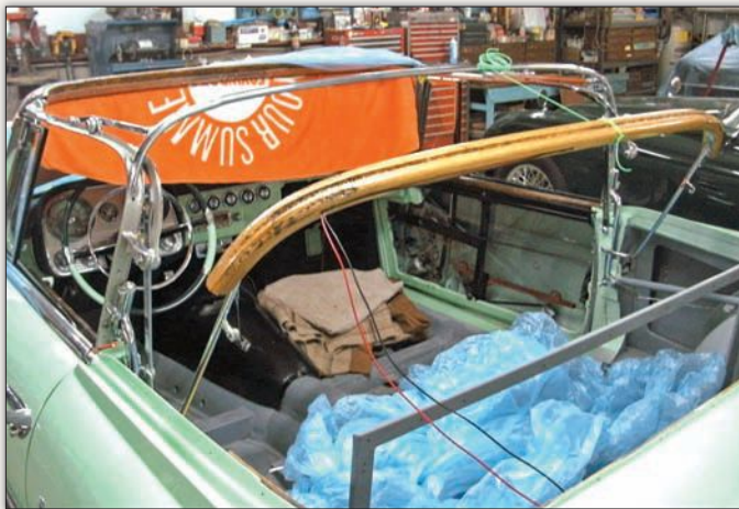
In addition to sourcing the correct top fabric, Whitehall had to carefully reassemble the top's internal frame and structure, after sending it out to have it rechromed. Additional work was needed to get the top to fit and the structure to properly operate.
