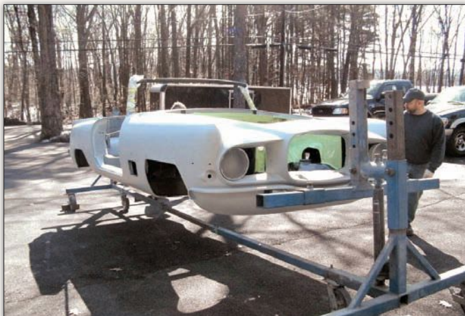
Mounted on a rolling rotisserie, the fully prepped Dual-Ghia body was moved to the paint shop, where several coats of primer were followed by four coats of color and several more coats of clear, for a stellar finish.
