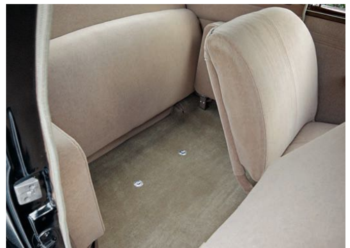
A pair of folding rear seats provides four-passenger capacity in this coupe when down and increased cargo area when up.
