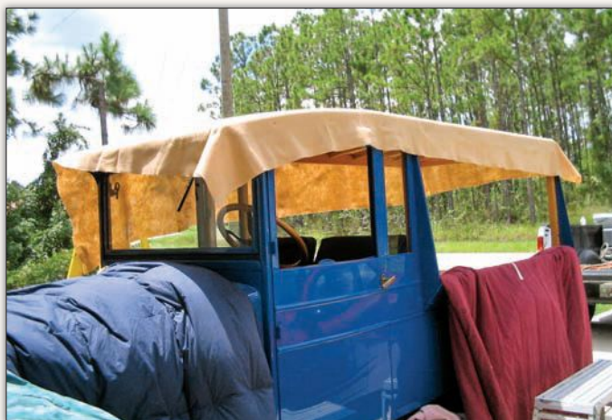
Before the top vinyl layer was installed, a proper fabric sheet was attached to the large wood roof structure by the upholsterer as part of the process.
