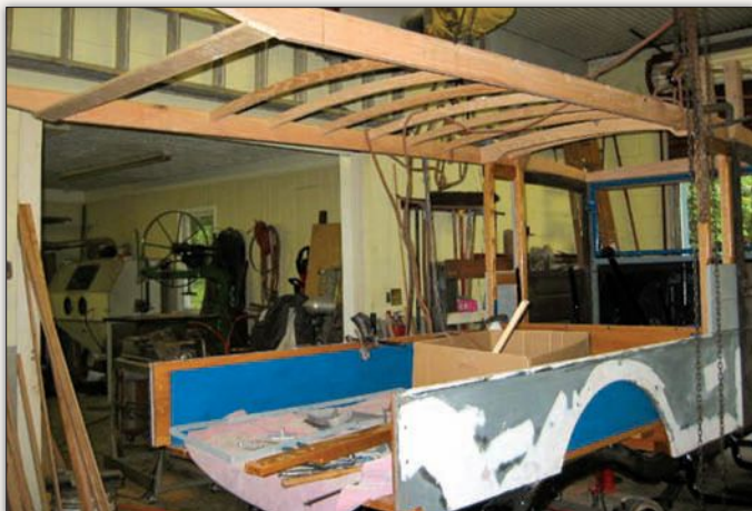
The top frame is shown here being test-fitted into place before final assembly. Note the extensive use of wood throughout the body and frame. From the door jambs back, wood is used extensively throughout this Graham truck.
