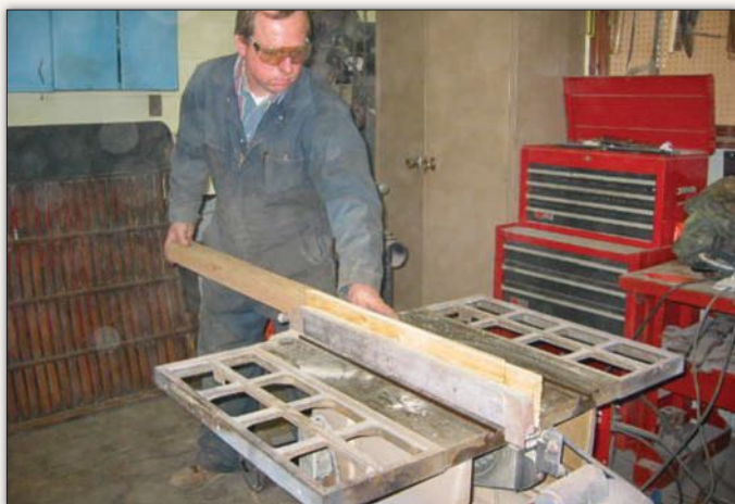
Restoring a wood-framed vehicle requires an entirely different set of tools than when working solely in steel or other metals. From the table saw shown here to the jointer to the shaper, having the right tools makes the job far easier to complete.
