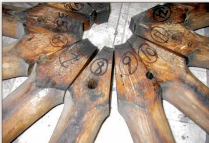
In disassembling the vehicle, the couple carefully documented and marked every part that came off the car. The wood spokes were in good enough shape to be refinished, but were marked in sequence for proper reassembly.
