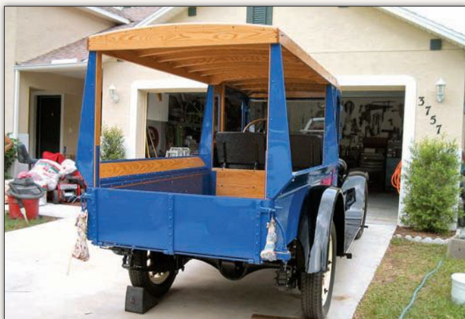
With the body and paint complete, here is an image that shows, again, how extensively wood is used throughout the truck, the main roof extending from the windshield all the way back through the canopied section.
