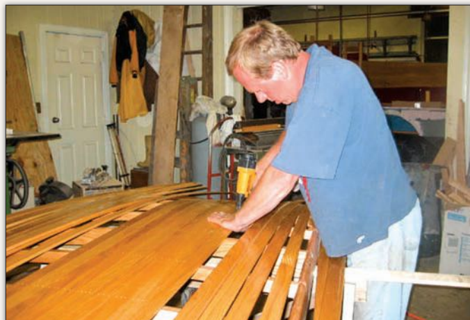
Here Ed is shown attaching the many long runners that complete the wooden roof structure. Given the repetitive nature of the task and the size of the boards—long and narrow—Ed had a local mill fabricate the individual pieces to his specifications.
