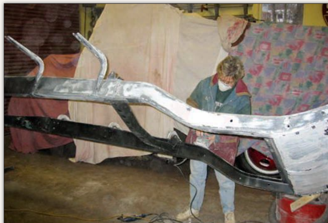
Having likely been stored inside for decades, the Graham's steel frame was relatively free of rust. Here, Barb continues the job of smoothing the surface before any final coats of protective paint are applied to the frame.
