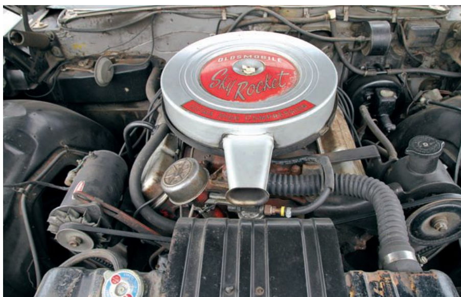
This 330-hp, 394-cu.in. "Skyrocket" V-8 is still factory-fresh, having traveled fewer than 60,000 miles in 53 years. It got new hoses and belts as a precaution against dry rot.
