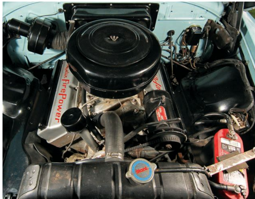
The 331-cu.in. Hemi V-8 gained 55 horsepower via induction and exhaust enhancements for 1954. This example has yet to require a rebuild.
