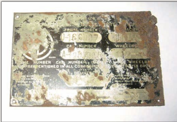
Working from a corroded and rusted chassis tag, Ed and Barb Joyce had new, blank tags exactly recreated, making sure to match fonts, color and spacing as best as possible, in order to complete the restoration as thoroughly and correctly as they could.
