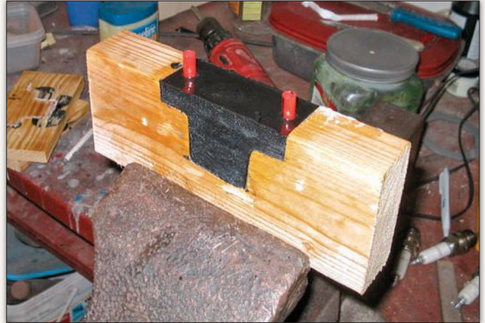
Graham Brothers trucks have largely been lost to history, so with so few spares available, beyond the Dodge running gear, the Joyces went so far as to mold rubber pieces in their home shop by creating molds from wood.
