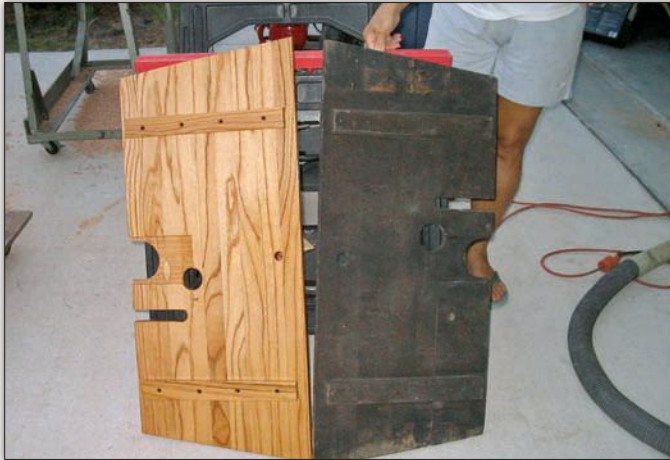
Shown here next to the original piece that came out of the car, the floor recreated by Ed was made from solid red oak. For the wooden pieces, Ed measured carefully and machined and worked each piece until the fit was perfect.
