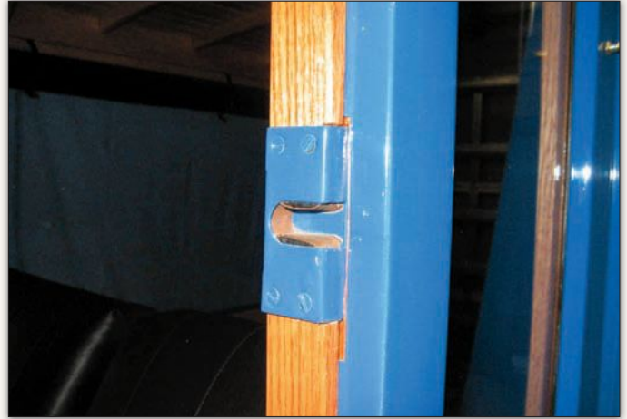
This closeup of the door jamb shows in detail the techniques used by Graham Brothers and now Barb and Ed: sheetmetal formed to fit over a hardwood frame and attached via small nails.
