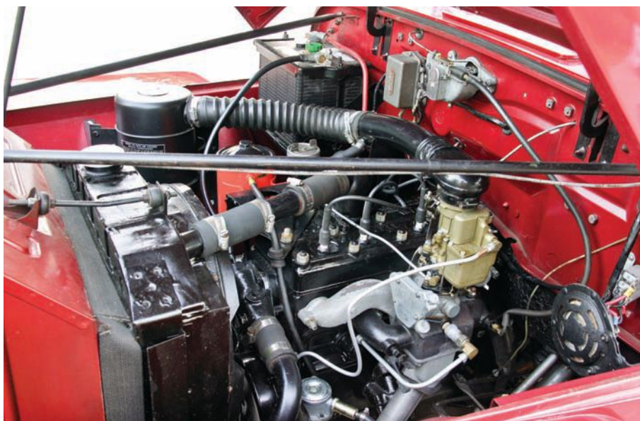
The 60hp Go Devil four-cylinder was standard issue on the truck, a transplant from the Willys CJ and military Jeeps. A deep 5.38:1 axle ratio helped when the hauling was heavy.
