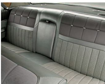
Seat upholstery is two fabrics and Moroccan vinyl, and all have proven durable. The front bench seat has power controls, and the rear has an armrest and cigarette lighter.
