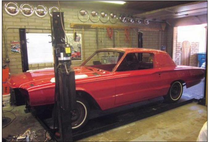
At this stage, most of the disassembly has occurred. To help expedite delivery to a local facility for media blasting, many of the major body panels have been reunited with the chassis, while the entire suspension system remains bolted into position.
