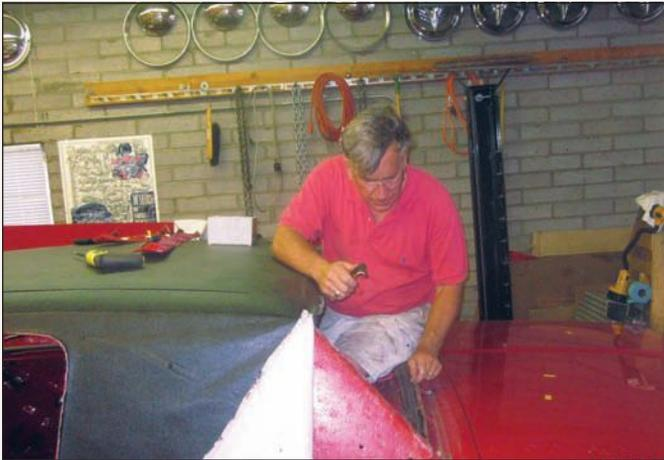
With the interior gone, it was possible for the team to remove the vinyl top without putting stress on their lower backs. As that process gets under way, the last bits of the original weatherstripping are being eliminated from its channel.
