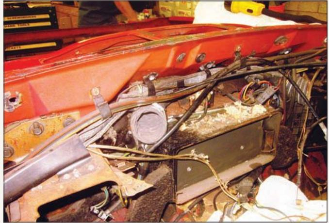
As the instrument panel and padded dash are removed, it becomes clear that small vermin had occupied its recesses. The remains of a mouse nest were uncovered; however, damage had been surprisingly minimal, in spite of the reputation of rodents for mayhem.
