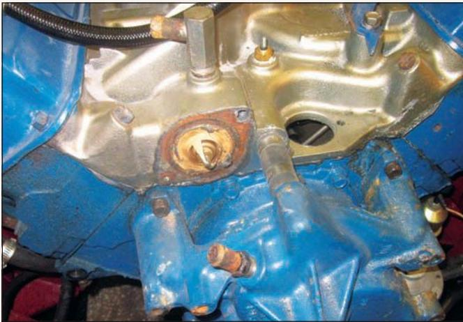
In spite of earlier work by previous owners, the original FE-Series 390-cu.in. engine had been retained and repainted, which meant that when its bolt-on components had been removed to facilitate its extraction, expected minor corrosion was uncovered.
