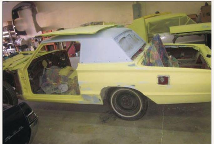
In order to prevent the bare metal of the body panels and shell from flash-rusting, even in the dry desert climate, a protective layer of epoxy primer was applied, at which point exterior surfaces could be smoothed with a skim coat of body filler.
