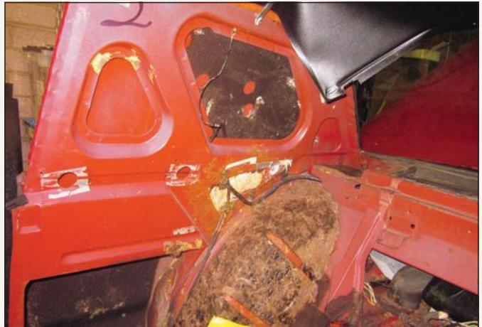
At this point, a significant portion of the interior has been removed, exposing the vast C-pillar substructure. To the relief of the team, none of the metal in this area had been compromised by rust, nor had vermin destroyed the original insulation.
