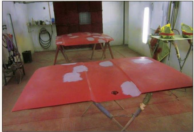
Now five months into the process, yet another application of primer revealed that not all surfaces were as smooth as they should have been. More filler in select areas was applied and continuously sanded smooth before paint could at last be shot.
