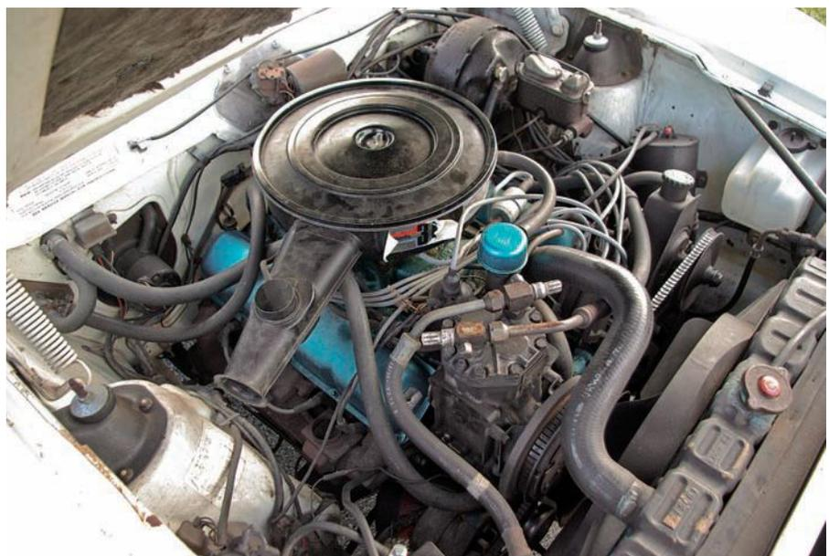
**While the less-powerful 360-cu.in. V-8 in the white Javelin doesn't quite have the get-up-and-go of the orange car, it still has enough torque to keep up with today's traffic.**
