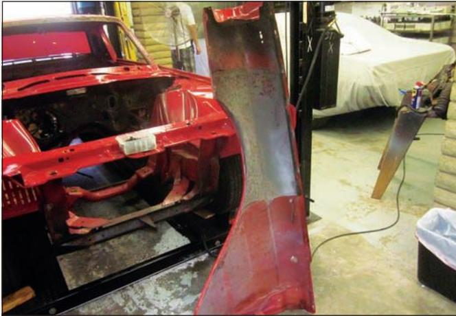
Both sides of each body panel were carefully removed and inspected. Here, it's the right-front fender that's being inspected, and upon closer examination, only a trace of surface rust can be seen. Holes for fender trim are apparent near the leading edge.
