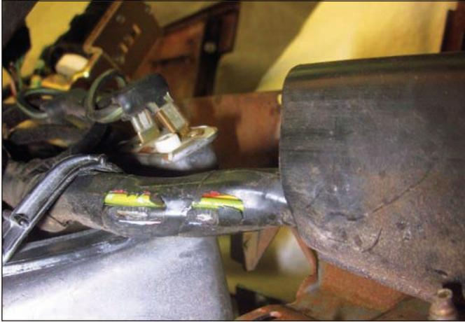
Although the Thunderbird had been able to ward off rust through the decades, the first hint of potential trouble due to rodents was discovered when the wiring harness was being removed from the body: Mice have chewed through the wiring's insulation.
