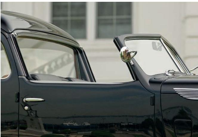
Matching rake of chauffeur and passenger windshields is an elegant touch by the LeBaron styling staff. In foul weather, a roof insert covers the chauffeur's compartment.
