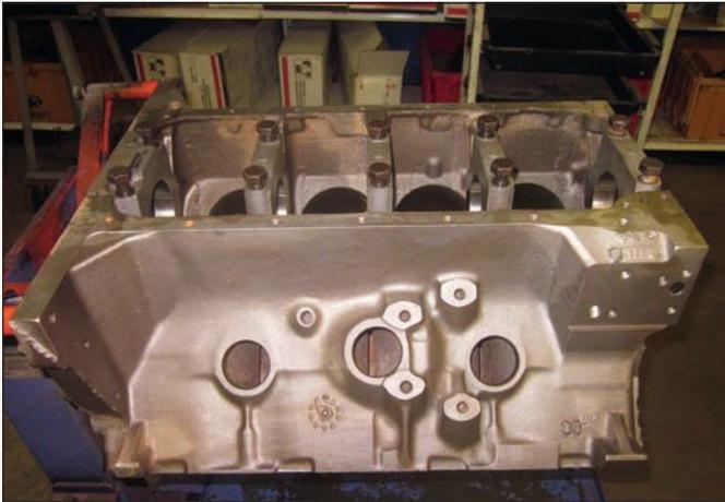
After the engine was removed from the Thunderbird, it was sent to an engine specialist. There, it was completely stripped, evaluated for hairline cracks and fully cleaned before the cylinder bores were subjected to a standard .030 overbore.
