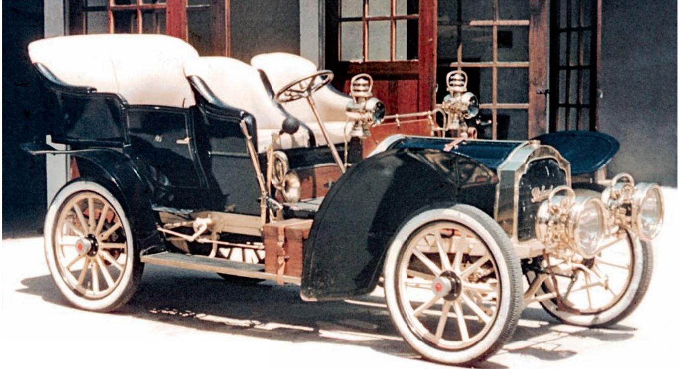
**This fine-looking 1905 Packard Model N touring car features, like all Packards of the time as well as many other American cars, a right-hand-mounted steering wheel. It would be a few more years before American automakers would settle on left-hand steering.**
