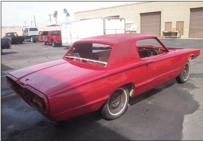
Single-stage urethane, matched to the original factory red hue, was finally applied to the body shell and other exterior body panels. Although exact details of the process are not known, it was permitted to cure before being returned to the restorer.
