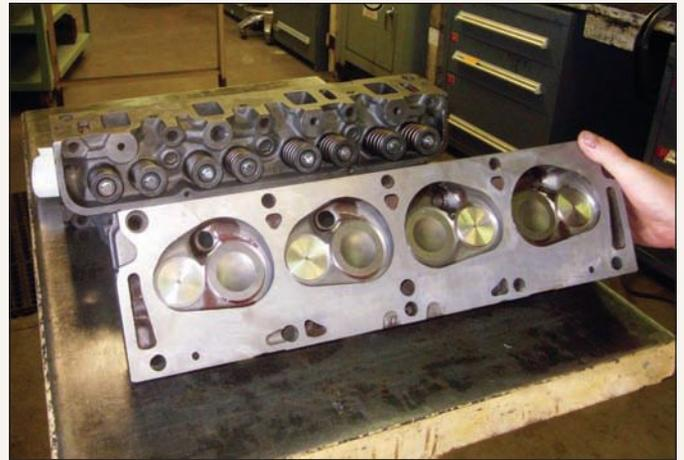
Each of the cast-iron cylinder heads was also cleaned, stripped and evaluated before it was rebuilt. The face of each was milled to true so it would mate with the block's surface, and then OE 2.02/1.57-inch intake/exhaust valves and OE springs were installed.
