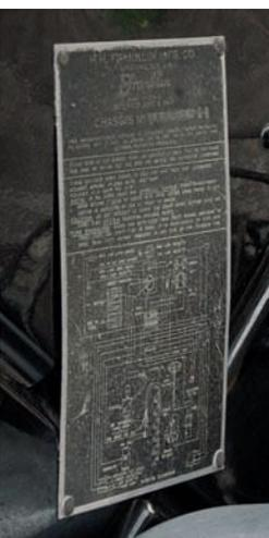
The 10B ducted its engine-driven fan to cool the air-cooled cylinders; maintenance information and electrical schematic were included with chassis plate.
