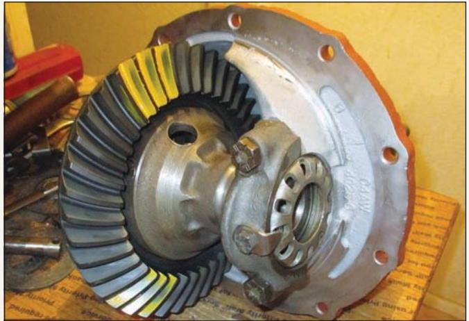
Seal concerns aside, careful examination of the differential revealed unwanted gear wear, forcing a total rebuild. Marking compound on select teeth of the ring gear helped determine an acceptable amount of lash. If not set properly, the gearset could fail.
