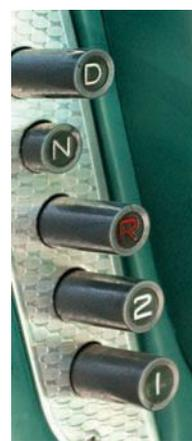
The Sport Fury for 1959 was outfitted with several distinct features, including the unique upswept exterior side trim and the half-padded steering wheel. Besides the Deluxe radio, pushbuttons were also used to engage the three-speed TorqueFlite automatic transmission.
