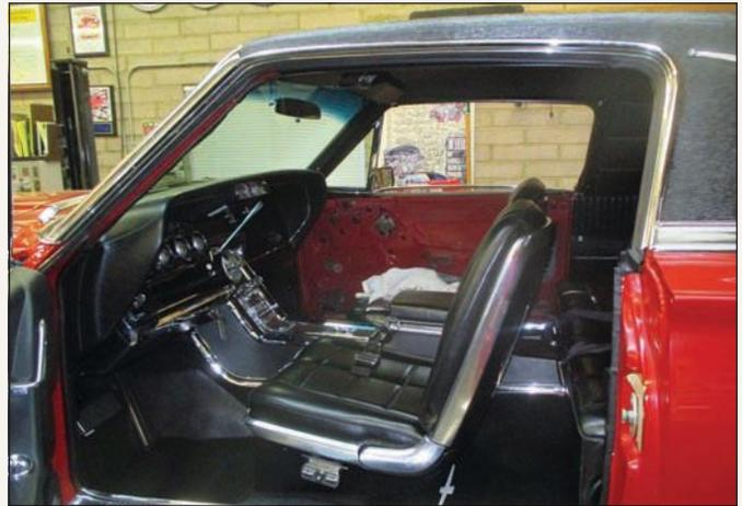
Look closely and you'll note that, along with the front bucket seats, most of the interior has been completed, including the C-pillar trim, rear seats, restored center console and steering column. Note the exterior top trim has also been returned.
