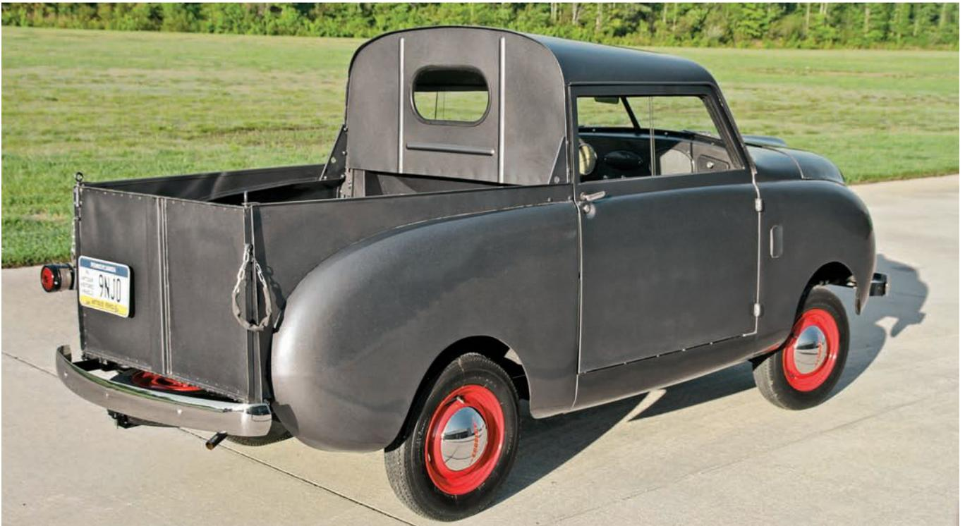
Crosley had to keep it simple in order to offer a diverse model lineup, so the "round side" pickup was derived directly from the sedan. The back half of the car body was cut off, then bedsides and a gate were added. Even the fuel tank filler pipe (above) remained in the original location.
