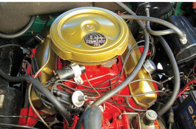
Equipped with the Golden Commando 395, this 360.8-cu.in. V-8, with its wedge-shaped combustion chambers, produces 305hp.
