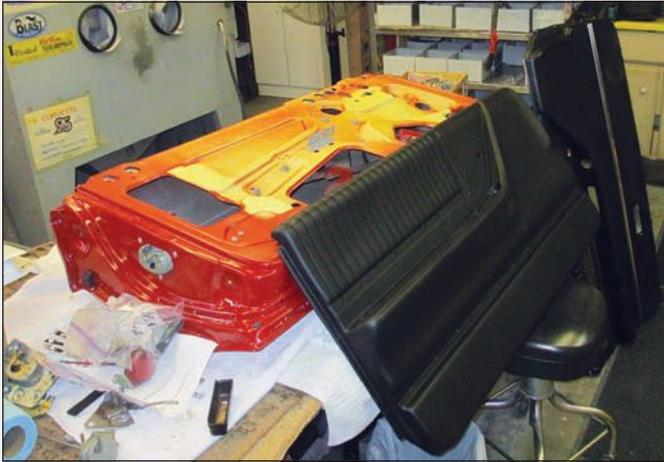
To prevent a restoration project from getting bogged down, it's helpful to stay one step ahead. Here, new door panels are in the process of being test-fitted, as the other body panels and main shell receive a second corrective coat of PPG single-stage urethane.
