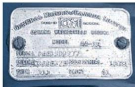
**The 248-cu.in., two-barrel-carbureted, 107-hp straight-eight starts instantly and offers lots of hill-pulling torque. The data plate reveals its GM of Canada Ltd. origins.**
