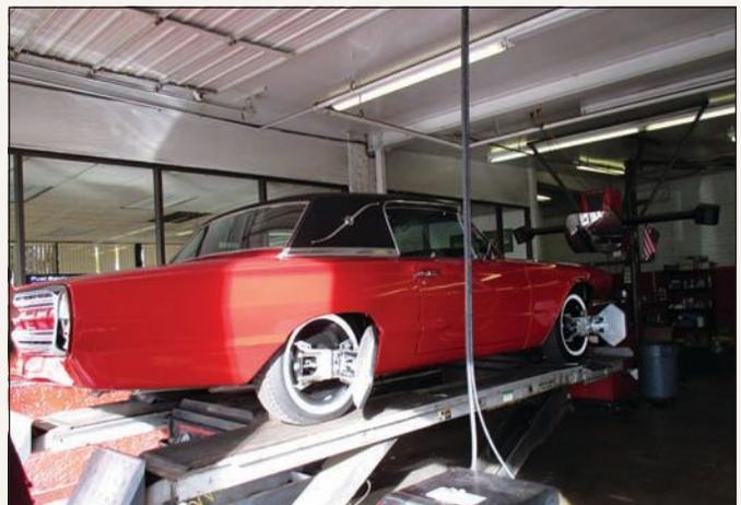
An important step in most restorations that's rarely discussed is the proper alignment being performed here. Regardless of how carefully the steering geometry is set during reassembly, a few degrees of error can lead to poor handling and premature tire wear.
