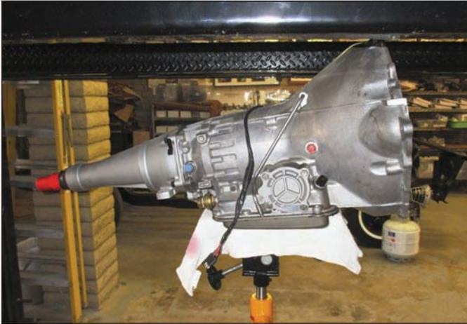
Before turning the restored Thunderbird over to the owner, the restorer subjected the car to a couple of shakedown runs. After some adjustments, a fairly serious vibration developed during another test drive; the transmission had to be removed to investigate its cause.
