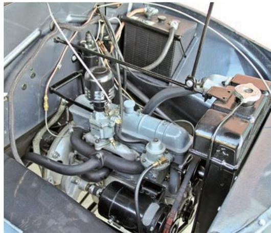
The Crosley pickup's interior is spartan, but boasts a full compliment of gauges and a speedometer. Power comes from Crosley's 44-cu.in. cast-iron four-cylinder, backed by a T-92 Warner three-speed gearbox.
