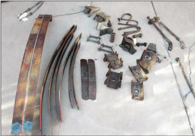
After the second repaint had been accomplished, restorer Ward Gappa and his team stripped the suspension from the chassis, including the rear semi-elliptic leaf springs, both of which have been separated to get them ready for media blasting.
