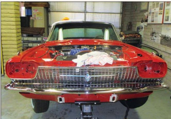
In spite of the installation of the front fenders and the related bumper and grille, there was still a long list of tasks that needed to be accomplished, including adjusting panel gaps, refitting the hood and finishing the electrical system and remaining trim.
