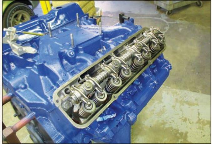
Earlier, an engine specialist stripped the Ford's 390-cu.in. block in preparation for its rebuild. With the cylinders bored .030-over, new pistons and other critical internals were installed. The FE-Series V-8 was also balanced to ensure smoother operation.
