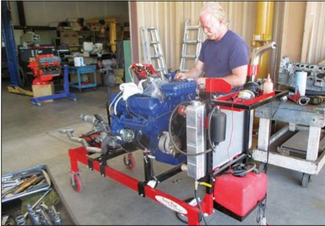
Rather than break in the rebuilt V-8 while it's bolted in the chassis, it was done on a special engine stand. In this setup, it would be easier to correct any problems that might arise without having to remove it from the chassis, risking damage to the new finish.
