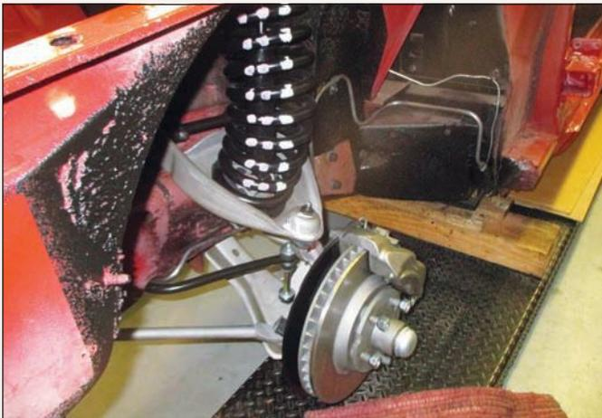
Accompanied by new bushings and ball joints, the suspension and brake systems were rebuilt and reinstalled; the two-piston calipers had also been rebuilt. Note that the front coil springs were refinished to factory color, including paint dab markings.
