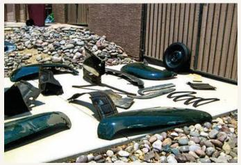
After sitting in post-purchase storage for a period of time, the car finally began to be restored in earnest with the removal of several key body panels, select trim and the front inner fender panels, each carefully laid out for evaluation and documentation.
