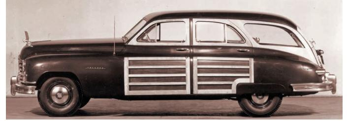
Postwar Packard station wagons used steel bodies, with wood employed to form the wagons' rear section, as well as the side trim. This 1949 Packard Eight "station sedan" rode on a 120-inch wheelbase and had a list price of \$3,449. Note how squared-off the wood paneling was.
