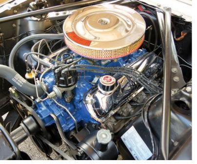
Karl's father negotiated the two-barrel 289 V-8 engine's appealing chrome dress-up kit as part of the car's initial purchase. The engine was preemptively rebuilt at 100,000-miles - after the restoration was finishedbut the original pistons were reused.
