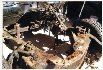
Both the engine and three-speed manual transmission were removed, allowing easy access to the rest of the electrical and brake systems, as well as the front suspension. A thick layer of undercoating had preserved most of the frame and control arms.
