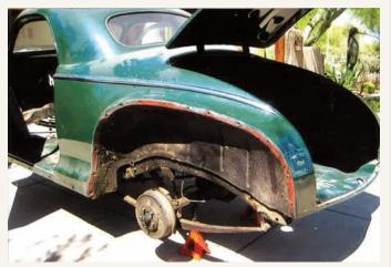
Focus shifted to the disassembly of the rear portion of the brake system. To help make moving the Business Coupe easier during much of the remainder of the restoration, the differential, axles and rear suspension systems were left intact, yet were carefully evaluated.
