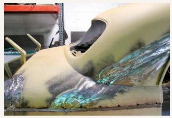
To fill the void in the body seams after the lead was removed, strips of 18-gauge metal were MIG welded in place. This also served to reinforce the panel junctions. Here the welds have already been ground smooth using a rotary sander.
