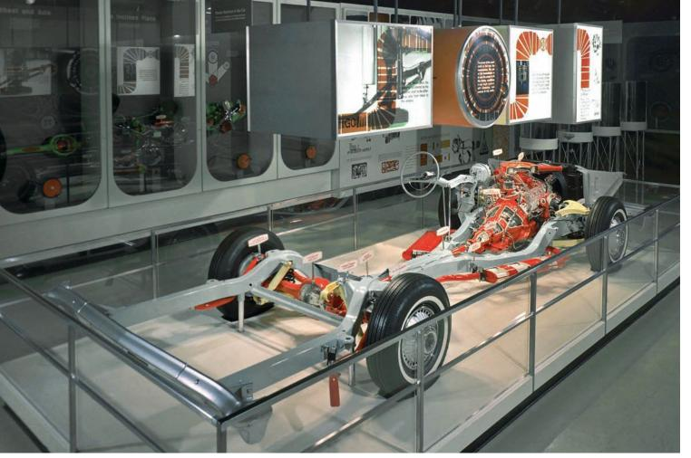
This chassis was built for show and features a cutaway small-block V-8, Powerglide transmission, rear end and muffler and small I.D. signs.
