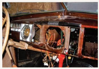
Inside the cabin, the bench seat has already been removed, permitting greater work space to tackle the disassembly of the woodgrained instrument panel and the rest of the wiring harness. Fortunately, there was nary a trace of rodent infestation within.
