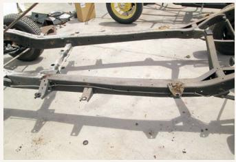
As the body began to receive its restoration treatment, the Dodge's frame was further stripped and carefully scrutinized. Against all odds, nary a spec of invasive corrosion was discovered compromising its structural integrity, a fact that made the restoration task easier.
