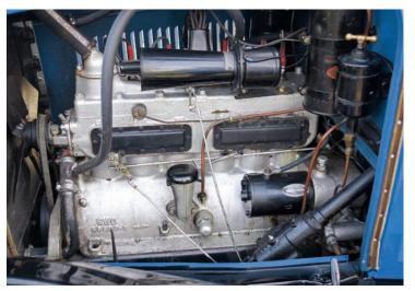
Single one-barrel updraft Stromberg carburetor provides fuel to the 180.2-cubicinch straight-six flathead engine, which develops 54 horsepower at 3,000 RPM. The Chrysler's ride is very smooth and comfortable, thanks to the Weed Levelizer friction cable "shocks."
