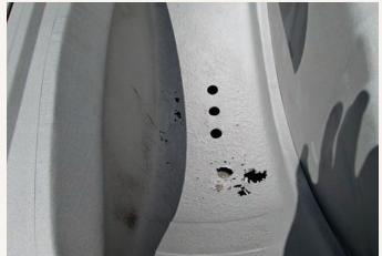
Considering the Dodge's eastern origins, the level of exposed corrosion seemed minimal; however, in typical fashion, the spare wheel well in the trunk floor would require careful patch work before moving forward with the project.
