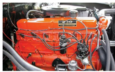
Uninformed enthusiasts are always taken aback when they see the 230 Turbo-Thrift 140hp straight-six under the hood. With so few six-cylinder-powered SS models remaining, it's a credit to the owner for keeping the car as-built.
