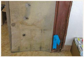
Although it was complete, the original cloth/leather interior showed water stains and other damage from decades of use. The upholstery, including the door panels, was retained in order to duplicate the colors and pattern when the time came later in the restoration.
