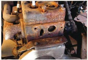
Although it was functional, the Dodge's 230.2-cu.in. straight-six engine exhibited some corrosion, especially the water distribution tube (within the oval opening), a critical passage that maintains proper cooling. The L-head engine would need to be rebuilt.
