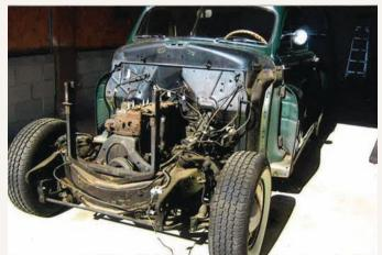
Once the front body panels were unbolted from the Dodge, the removal of various parts that surrounded the engine began, including the radiator and some of the electrical wiring. Each wire and connector was carefully tagged for future reassembly.
