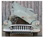
The Buick's hood is hinged on either side for easy access to the sosmooth-you-don'tknow-it's-idling 248-cubic-inch, 6.3-compression, 110-hp straighteight engine.
