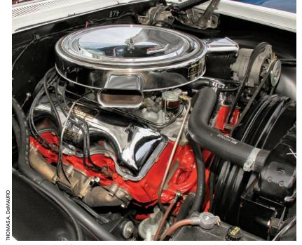
The 425hp, dual four-barrel 409 was the top Impala SS engine for the street.
