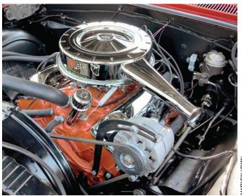
With its mild hydraulic cam, the new 340hp version of the 409 was a smooth and torquey street engine with 420-lb.ft. at 3,200 RPM.
