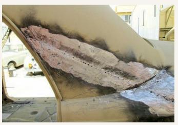
Manufacturers hid stitched body seams with lead, adding weight to the body and, over time, contributing to the discoloration of paint applied over the soft metal. A common step today is to eliminate as much of the lead as possible on the roof pillars.
