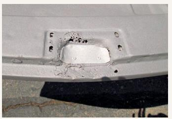
After dismantling, the body was separated from the frame and subjected to media blasting. The process exposed original bare metal, small pockets of corrosion and previous attempts at repairs, such as this riveted patch along the trunk lip.
