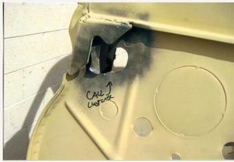
Shortly after the condition of the body was evaluated and the extent of its needs was determined, every surface was given a coat of epoxy primer to further ward off corrosion. Areas needing work, or that required consulting with a marque expert, were marked.
