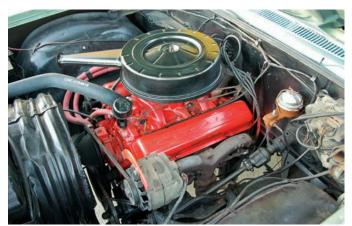
Compact in size yet quite responsive, the 283-cu.in. V-8 provides 195hp while returning 22 miles per gallon. It has never been rebuilt.
