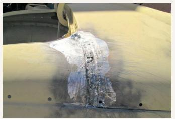
Another leaded seam was exposed, this time covering the junction between the rear section and the main coupe cabin. The lead, in all cases, was carefully melted out in small sections to prevent the main panels from warping; the rest was ground out.
