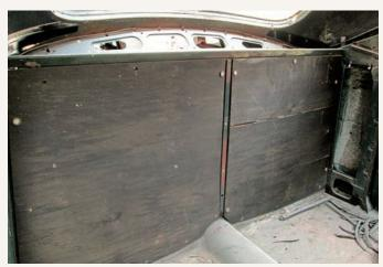
It may seem surprising, however Dodge still used thick slabs of wood to separate the cavernous trunk from the coupe's spacious interior. As fortune would have it, neither piece had rot, although deep cracks would eventually force the replacement of one.
