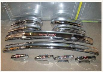
Chris managed several aspects of the restoration project. Both the front and rear bumpers and corresponding guards were removed and documented before being delivered to Kerr West Plating in Phoenix, Arizona, for proper refinishing.
