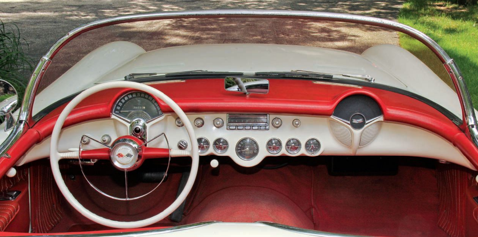
A 140MPH speedometer and a full complement of instruments were standard. These gauges are original, as is the signal-seeking AM radio.
