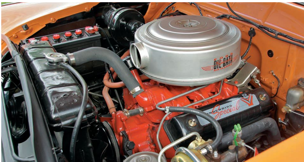
Ford's Thunderbird Special V-8 displaces 312-cubic-inches while making 225 horsepower and a mean 324-ft.lb. of torque at just 2,600 RPM. Oil Bath air cleaner sits atop a Holley 4000 four-barrel carburetor.
