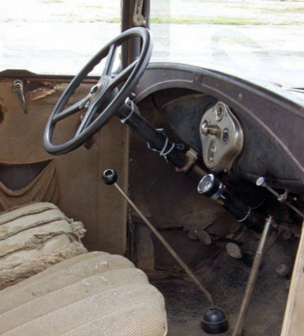
Little remains of the factory-installed wool cloth upholstery on the driver's seat, although its blue hairline stripe is still visible under close inspection. The rest of the interior fabrics—plus the rubber floor mat—have held up quite well for 85 years.
