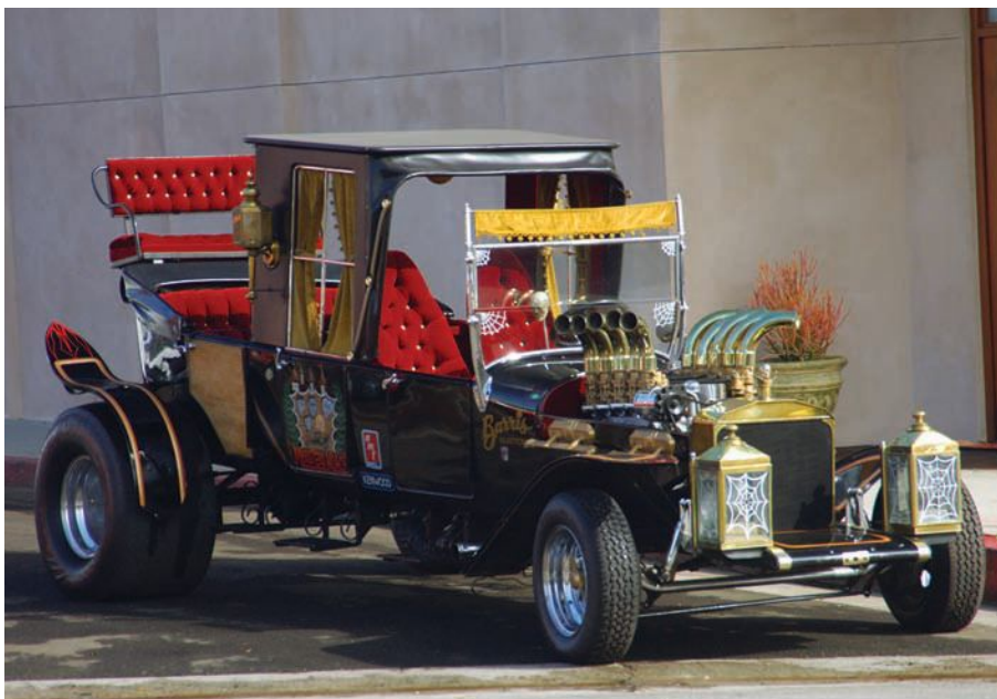
Dice up three Model T bodies, meld them together, add a Ford 289-cubic-inch V-8 and you have the Munster Coach , which had to accommodate the series' towering star, Fred Gwynne.
