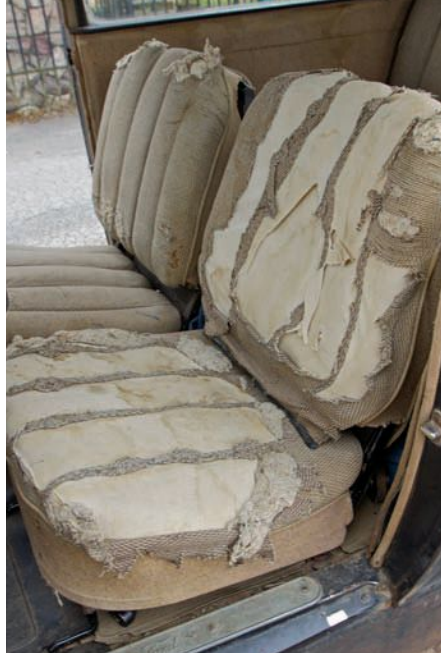
Little remains of the factory-installed wool cloth upholstery on the driver's seat, although its blue hairline stripe is still visible under close inspection. The rest of the interior fabrics—plus the rubber floor mat—have held up quite well for 85 years.
