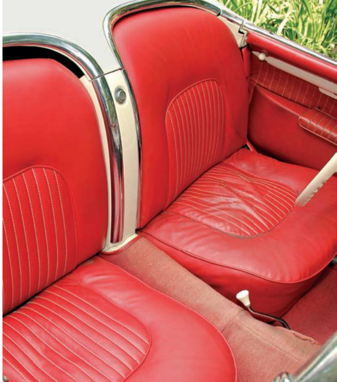
The body-colored “waterfall” element between the seats unified the exterior and interior design themes of the Corvette.
