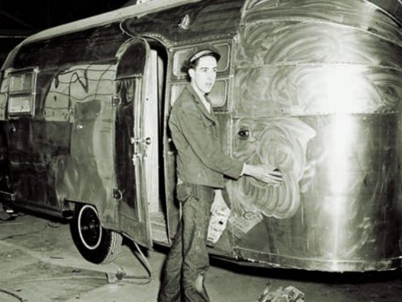
One important job at the plant was to polish out the aluminum skin prior to shipping the new trailer to its owner.
