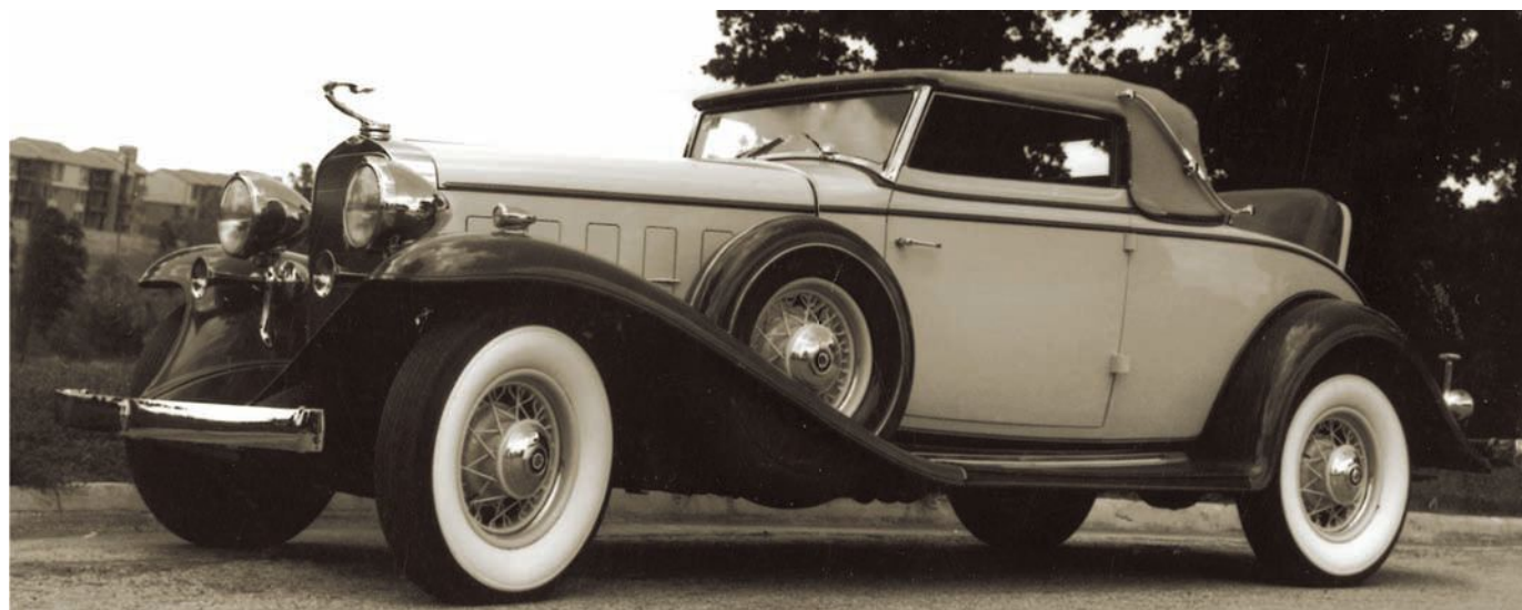
For 1932, the Art and Colour Section purposely styled the Chevrolet line to resemble the Cadillac. Grille shape and texture, hood vents, fenders and other key elements were similar, leading to the popular-priced Chevrolet being fondly called the “Baby Cadillac.”
