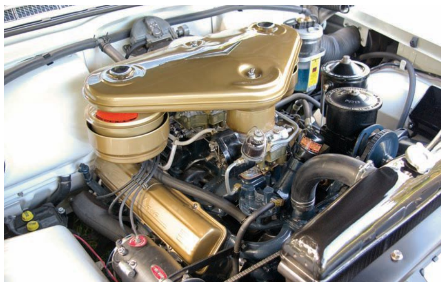
The pair of Carter WFCB carbs has been professionally rebuilt, allowing the Eldorado's original matching-numbers 365-cu.in. V-8 to produce 305 horsepower once again.
