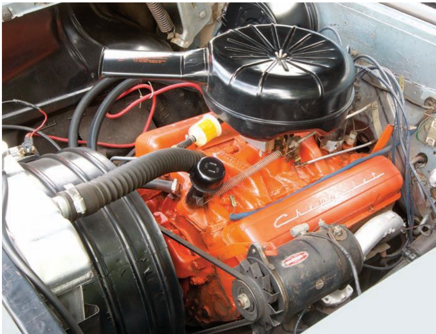
The repainted original 283-cu.in. V-8 engine has yet to require a rebuild; with its two-barrel carburetor, it produces 185hp.
