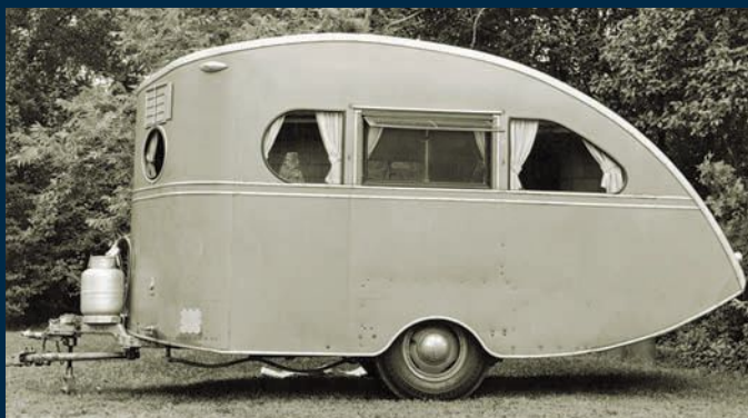
Another Airstream trailer, this one circa 1935. The uplifted tail was designed to provide ground clearance when exiting driveways, or coming off steep hills.
