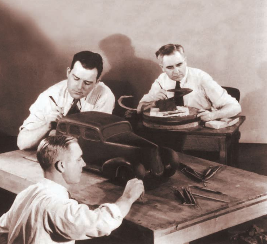
Detailed quarter-scale clay models were used to ensure correct proportions between body elements, and even tested for streamlining in a wind tunnel.
