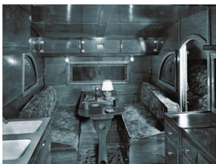
The interior of an early teardrop shows the efficient use of space, and nice wood paneling. The dinette converts into a bed.
