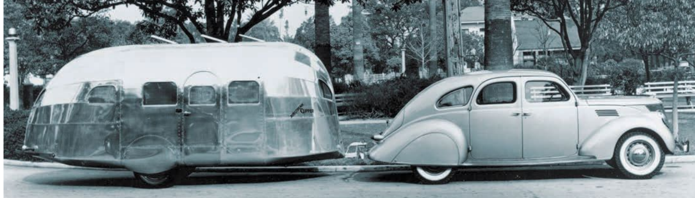
The 1936 Airstream Clipper introduced the classic aluminum construction and aero shape that became Airstream's hallmark.
