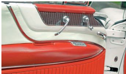
Acres of new red and white leather hides cover the restored seats and door panels, along with all re-chromed trim pieces, which cost a small fortune to have re-plated.
