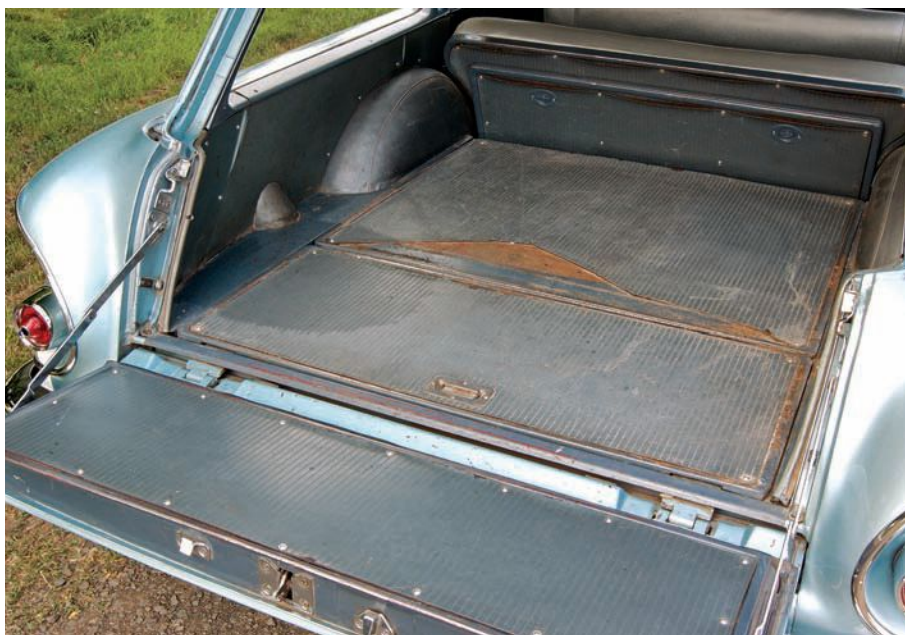
A linoleum covering made for easy cleanup of the cargo area floor. The blue dot in each tail lamp and the chrome headlamp covers are not stock but period-correct custom add-ons.
