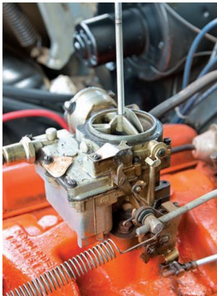
The repainted original 283-cu.in. V-8 engine has yet to require a rebuild; with its two-barrel carburetor, it produces 185hp.
