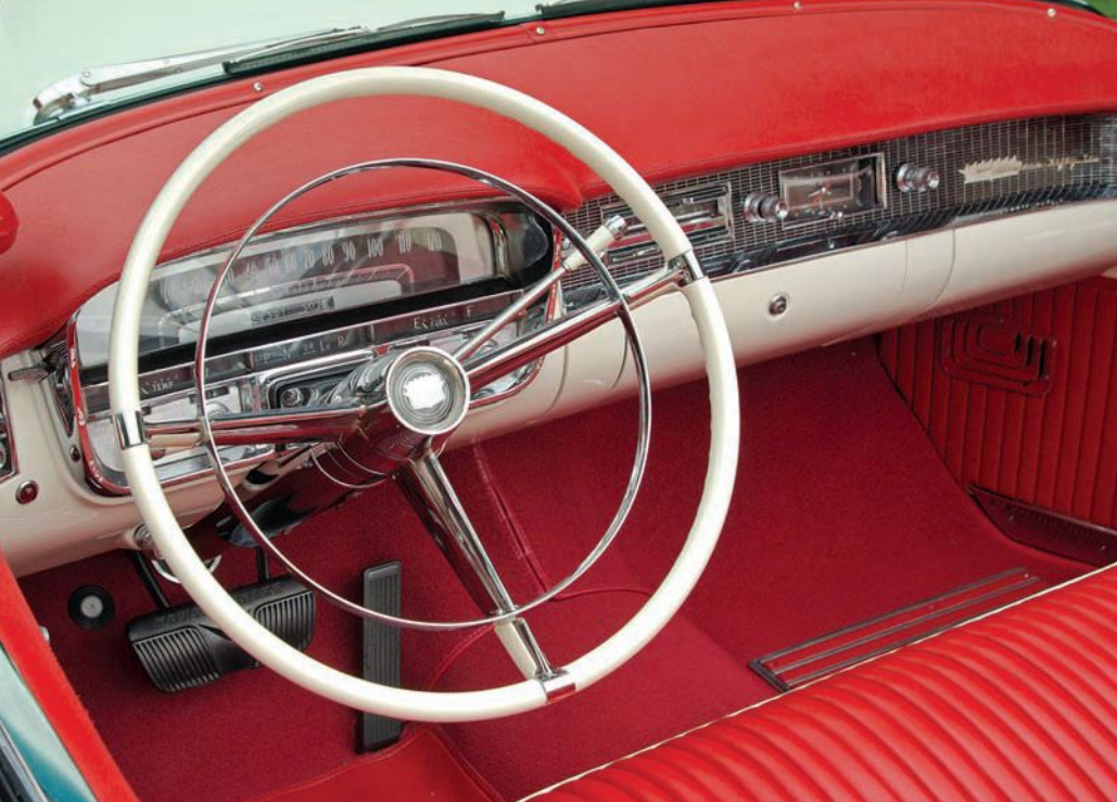
Every component on the Cadillac looks brand new, including the glovebox's interior. All the instrument-panel brightwork has been either polished or re-plated.
