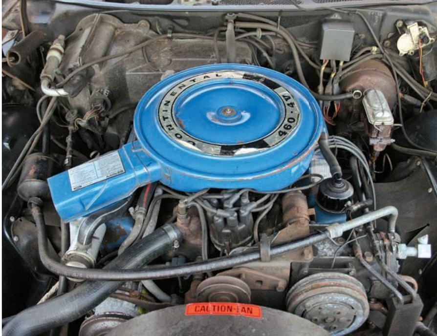
**This four-barrel-carbureted, 365hp V-8 has powered the Continental Coupe for more than 132,000 miles, and despite sitting inactive for 16 years, has never been rebuilt.**
