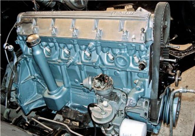
A cosmetic restoration of the original overhead-cam six engine included stripping its exterior, then priming and painting the block with several coats of the correct Pontiac Blue Metallic. The engine was not removed; rather, it was refinished in place.
