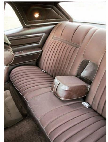
**The B-pillar-less body offered an elegant window line and made the large interior feel airy, despite thick C-pillars. The man-made nylon fibers used in the carpet and seat upholstery have proved unappealing to mice, which have left those materials intact.**
