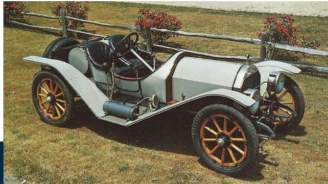
**1912** The 1912 Moon Model 30 roadster was a sharp machine, with sleek lines on a 116-inch wheelbase, and a 32hp T-head four-cylinder engine under the hood.
