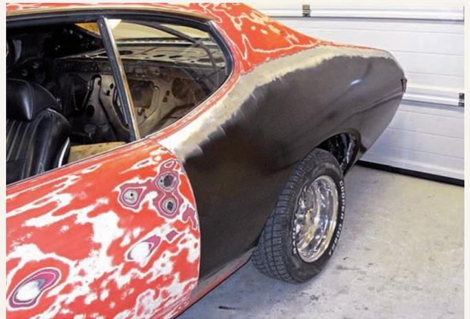
The Le Mans's body was in good shape, but ultimately, new reproduction quarter panels were installed on both sides because there was corrosion all around the rear fender lips. It cost the owner \$3,000 for the parts and labor to have them installed.
