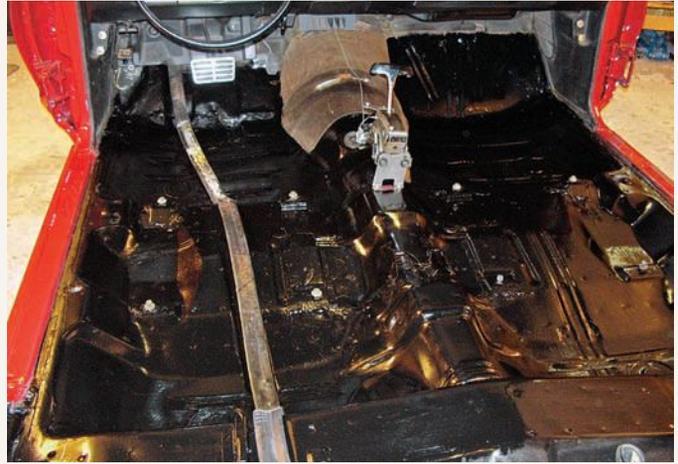
Thanks to northern Sweden's use of sand instead of salt, the entire floor pan was solid and free of any corrosion. After everything was removed, the floor was degreased, then sanded smooth before a coat of primer and a thick coat of POR-15 were applied.
