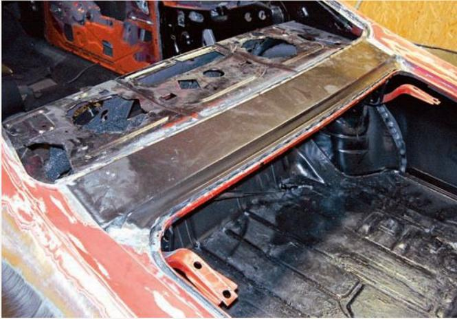
The replacement rear filler panel, which stretches between the quarter panels, was carefully trimmed to fit, then slowly MIG welded in place by a local autobody metal specialist. Fortunately, the water damage did not extend into the trunk area.
