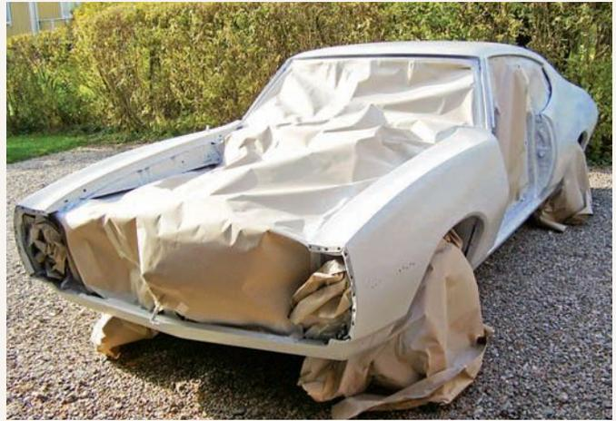
After taping off the interior and engine bay, two coats of a high-build epoxy primer were applied, followed by a double wet-coat of primer sealer. Roger did all the priming work in his home garage in order to save money on the final refinishing process.
