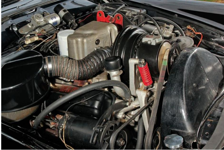
One of the unique aspects of the Hawk's 289-cu.in. V-8 engine is its induction system. On the cast-iron intake manifold, a Stromberg two-barrel carburetor contained in a cast-aluminum housing is fed compressed air from a McCulloch supercharger at a maximum of 5psi of boost. The exhaust then exits through a two-inch stainless steel dual system with twin mufflers and aftermarket chrome tips.
