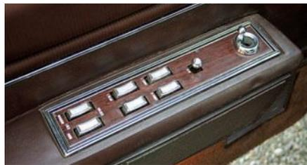
**Power controls for the exterior mirror, two-way seat, four windows and door locks were grouped by the driver's elbow.**
