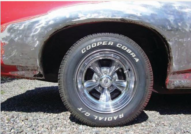
During the stripping of the right side quarter panel to remove rust bubbles that were showing through, it was discovered that the corrosion was far worse than originally thought. This is why the quarter panels and inner wheel wells had to be replaced.
