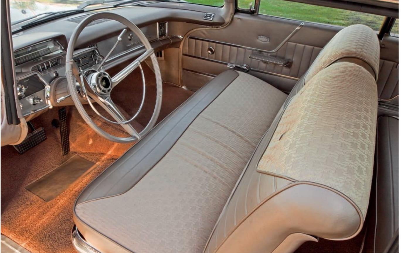
“Space planned for a new kind of comfort,” opines the 1959 Mercury brochure. Indeed, the clearance hump for the transmission was reduced 45 percent, thanks to the engineers tilting the engine back and to the rear slightly; seating for six was rarely so comfortable.
