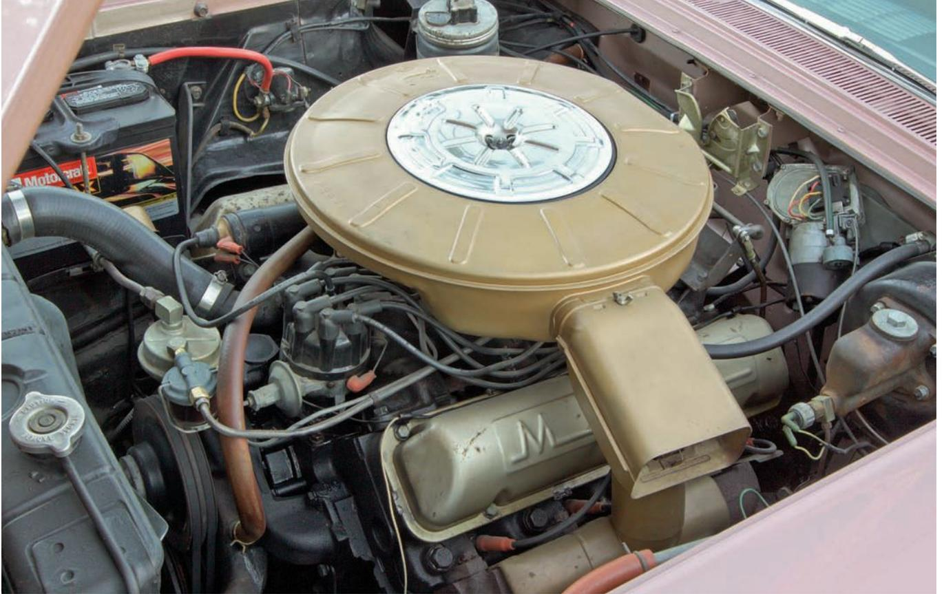
**“Here is performance that says, with quiet confidence, ‘Find the road, hill or curve that Mercury cannot master!’” Indeed, with 345 horsepower under foot (and, more crucially, 480-lb.ft. of torque) the Park Lane has performance that belies its external dimensions.**
