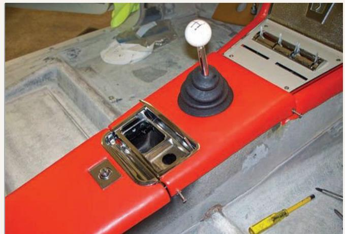
From a healthy supply of NOS parts collected over the years, the restorers were able to craft a near-perfect, factory-correct Avanti. Included in that stash were the new-old-stock ashtray and a roll of the correct orange Naugahyde for the console.
