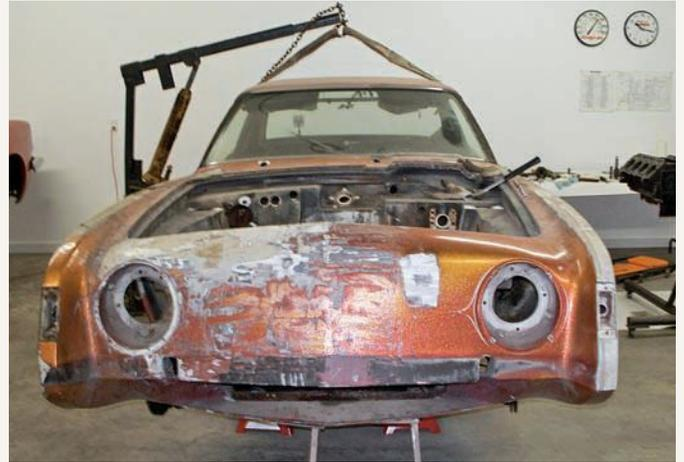
With the goal of the project to return the car to its factory-original condition, the restorer had the body removed from the chassis as part of the process of tearing the car down to its elemental components and almost starting from scratch.
