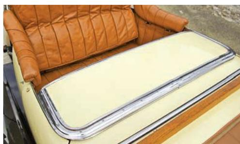
Here's what the semi-clamshell looks like with the forward portion lowered. The seat will fold forward.
