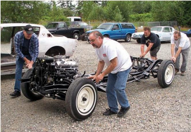
Ready to reunite the body with the frame, the crew at Avanti Northwest rolled the finished chassis, complete with engine and transmission, across the yard. Along with the powder coating, all wear items were replaced on the suspension.
