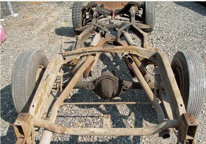
Though the chassis exhibited some surface corrosion beneath the fiberglass body, it was largely solid and intact. With its extra-strength center X-brace, the Studebaker Lark convertible chassis proved to be an ideal platform for the Avanti.
