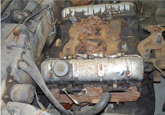
Despite the rough-looking condition of the engine, the powerplant was complete and salvageable. After minimal machining, the robust, supercharged Studebaker 289 cubic-inch V-8 was fitted with new pistons, valves, plugs, seals and bearings during the rebuild process.
