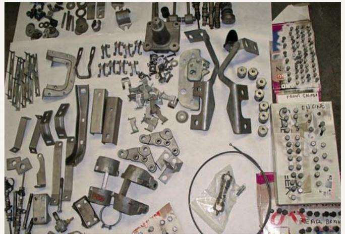
When it came to doing a “nuts and bolts” restoration, the restorers meant that literally, removing, cleaning and refinishing, or replacing when necessary, any and all fasteners, brackets and related hardware—and then carefully organizing it all.
