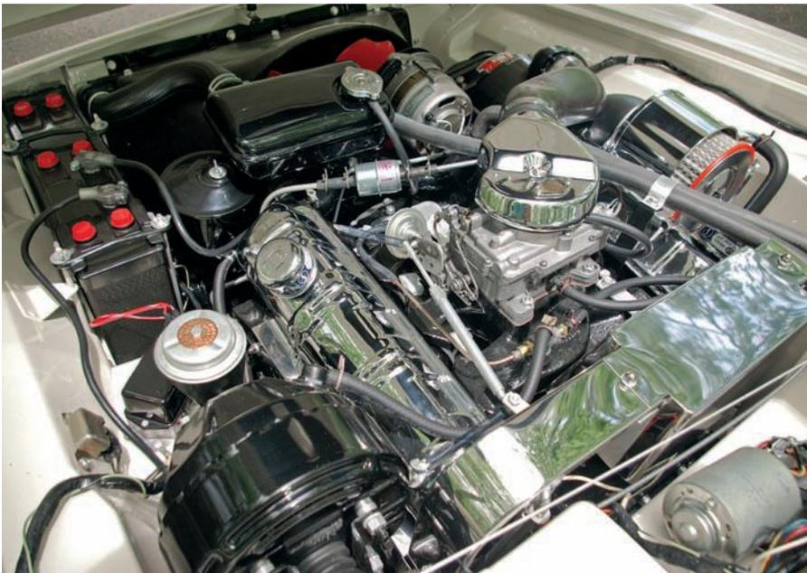
Studebaker's 280-horsepower supercharged "Jet Thrust" 289-cu.in. V-8 provided plenty of oomph for Studebaker's flagship, four-passenger GT car.
