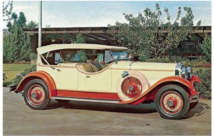
The 1929 Model M four-passenger speedster (aka dual-cowl phaeton) was a pretty car, powered by a 322-cu.in. single-overhead camshaft straight-eight with 115hp. This body was built by LeBaron.
