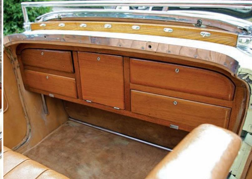
Rear seat forms half of a clamshell when lowered for the Brooklands' two-passenger version, with another panel forming a semi-tonneau. Cabinetry in the front bulkhead is fully functional and all original. So is the rear upholstery. This is the epitome of Twenties elegance.
