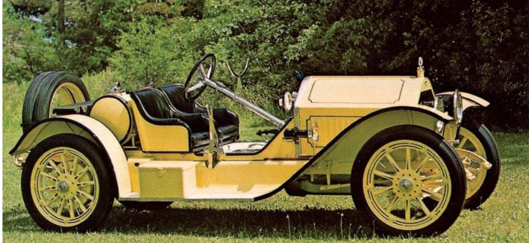
The sporty two-seat 1914 Bearcat was powered by a T-head four-cylinder, 50-horsepower engine. Stutz automobiles were targeted mainly to driving enthusiasts looking for a fast, good-looking car of distinction. It appealed to these buyers because of its outstanding racing record.
