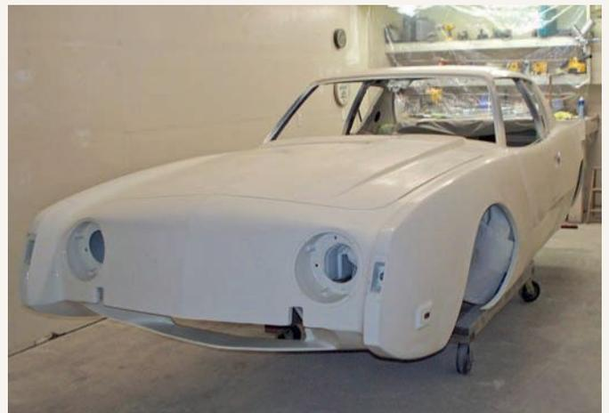
Bringing number two back to original meant a return to the factory Avanti White exterior, a process that included five coats of primer, five coats of white base color and finally four more of clear, with plenty of progressively finer hand sanding at every stage.
