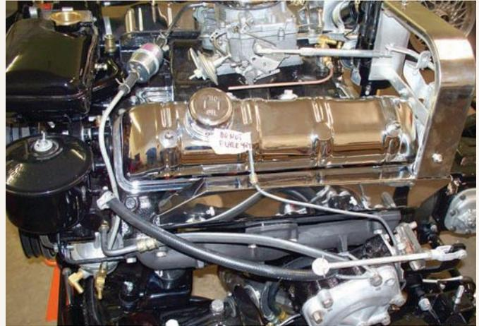
After the rebuild, the engine was almost unrecognizable as compared to when it first came into the shop. From the factory, Avanti engines had chrome-plated rocker covers, lifter cover, oil filler cap, air cleaner and voltage regulator.
