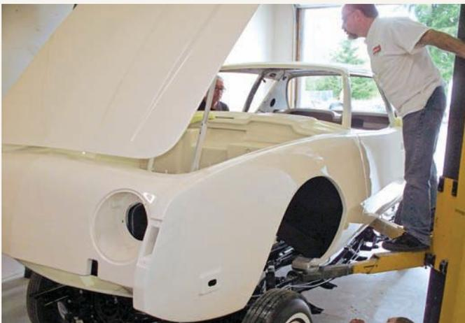
Slow and careful is the only right way to get an Avanti body back on its frame. Rubber grommets must be properly fitted between the chassis and the fiberglass body before bolting it all together, and the appropriate shims must be used for fine-tuning the fitment.
