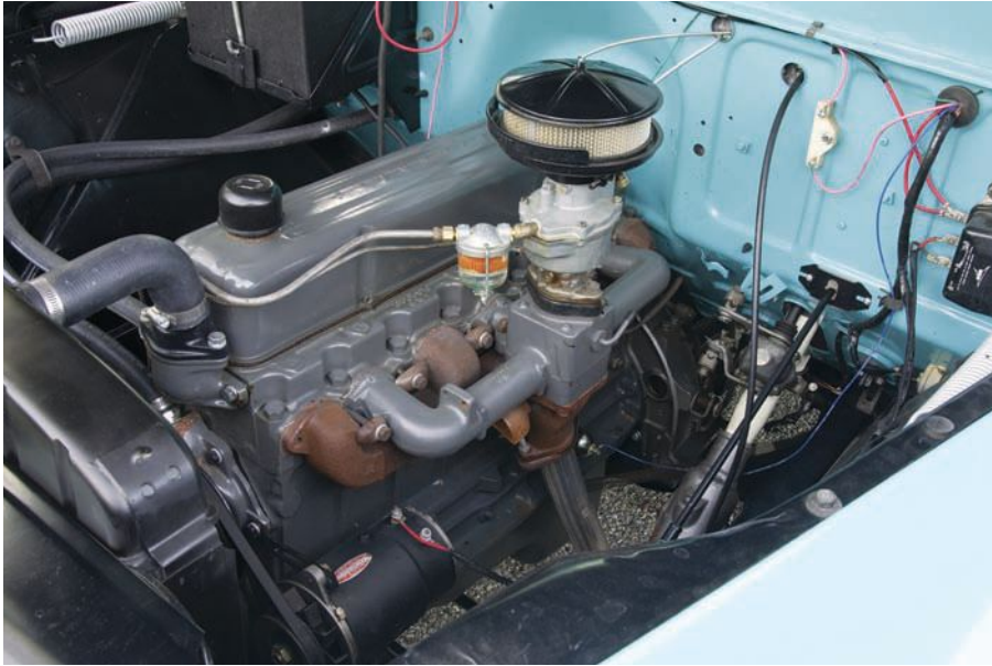
The 283 was available in '58, but this truck left the factory powered by a 235.5-cu.in. six. With a one-barrel Rochester carburetor and 8.5:1 compression, the 235 was rated (gross) at 145hp and 215-lb.ft. of torque.
