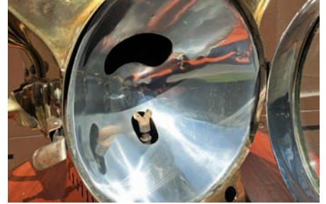
The burner inside the headlamp was accessed by opening the headlamp door that was hinged to the body of the lamp.
