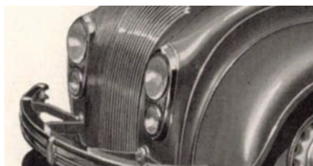
"That's Streamlining" was the way in 1934 that Chrysler described its new look in the data book issued to its sales staff. The styling of the Airflow, with its headlamps flush with the front of the body, represented a dramatic change.
