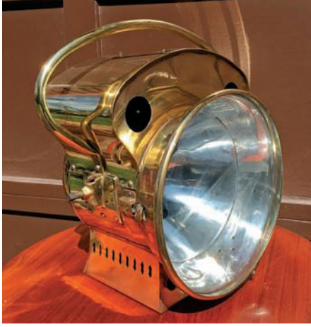
This Dietz No. 3 headlamp was fueled by acetylene gas sent from a separate tank usually mounted on the running board or next to the chassis near the cowl.
