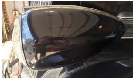
The huge headlamp on this 1936 Packard is an example of slipstream styling; all that metal to hold a small bulb for night vision.
