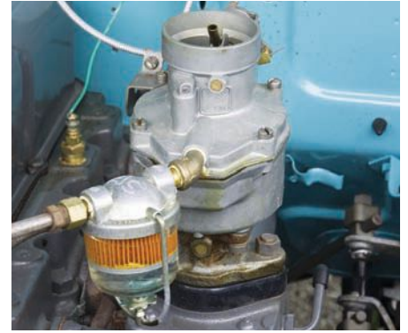
The 283 was available in '58, but this truck left the factory powered by a 235.5-cu.in. six. With a one-barrel Rochester carburetor and 8.5:1 compression, the 235 was rated (gross) at 145hp and 215-lb.ft. of torque.
