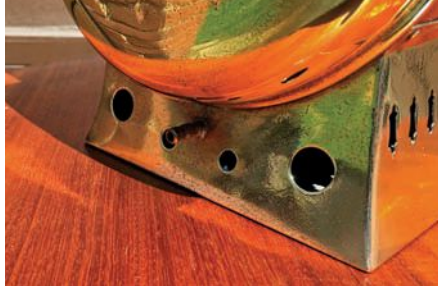
The inlet at the back of the Dietz headlamp is shown here; this is where the rubber hose attached to supply the gas to the headlight.
