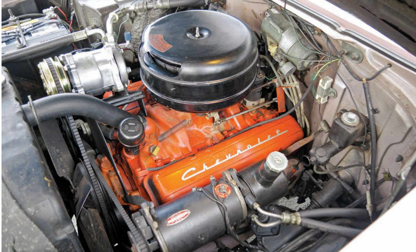
The 283-cu.in. Turbo-Fire V-8 is mated to a Powerglide, and its 185hp easily runs this car's factory-optional air conditioning.
