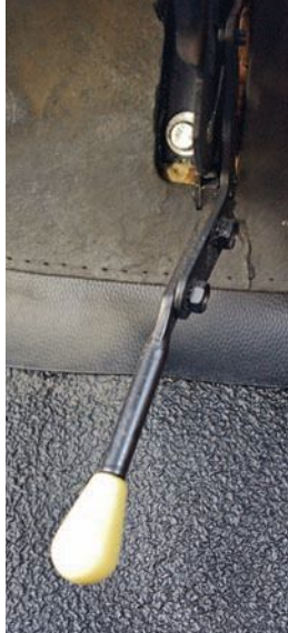
Ivory-knob-tipped lever controls the cowl vent. The recirculating heater was the cheapest accessory heater available and was a subsequent addition by the original owner—it may be more effective than the DeLuxe fresh-air heater.
