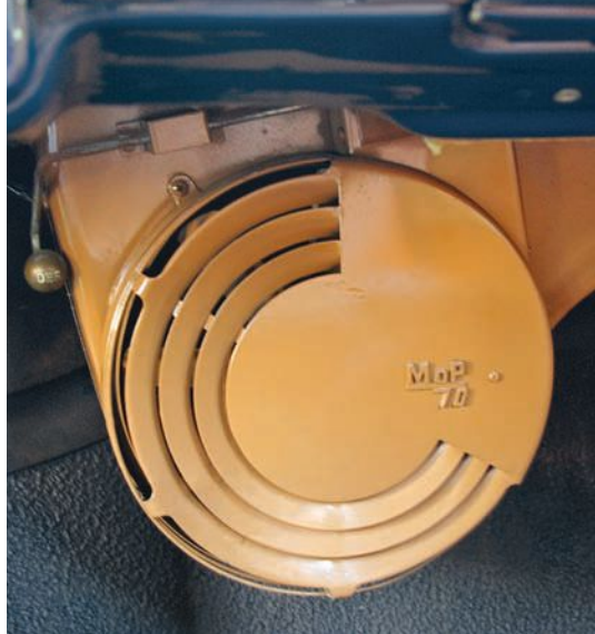
Ivory-knob-tipped lever controls the cowl vent. The recirculating heater was the cheapest accessory heater available and was a subsequent addition by the original owner—it may be more effective than the DeLuxe fresh-air heater.
