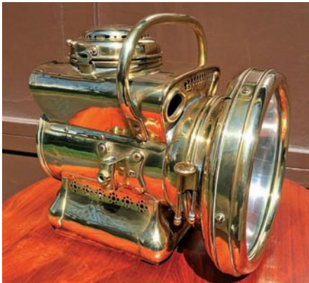
A self-generating headlamp made by Powell & Hamner in England and imported into the United States would have been a fairly costly accessory. It weighs about 6 pounds.
