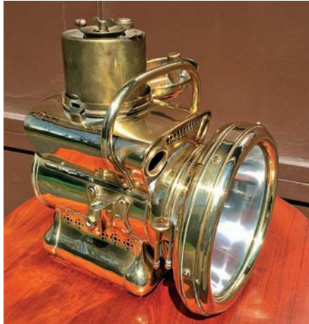
The fuel tank to hold the mixture of carbide crystals and water for the gas for fuel for a self-generating headlamp was contained inside the lamp itself, as seen here.
