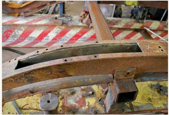
At several key positions, the frame's contours were too significant for the previously described bending method; it was determined that the metal would fracture. To prevent this from happening, they cut sections out of the bottom plate, exposing the channel within.
