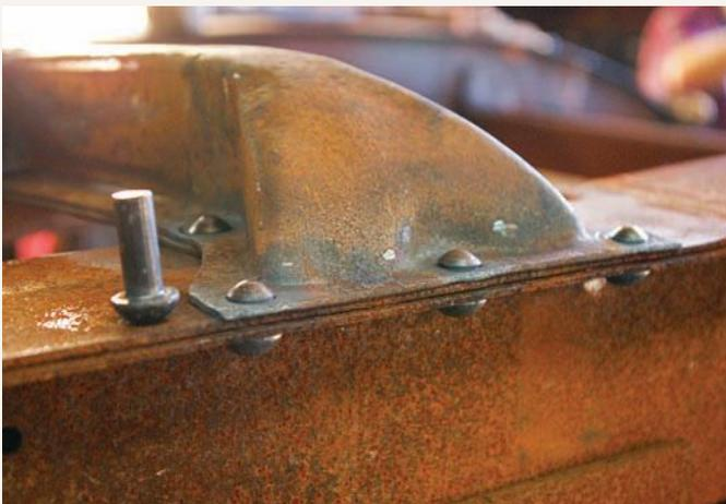
Creating enough pressure ensures that the heated rivets conform to their iconic conical domes, as well as create incredibly tight junctions as demonstrated here. This painstaking system was used for every connecting point along the length of the frame.
