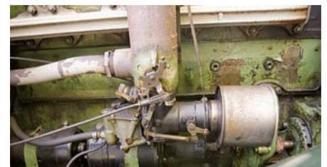
F-head engine is the star of the Super Six. It displaces 288-cu.in., produces 92 horsepower and features a balanced crankshaft for smoothness and high-speed capability.
