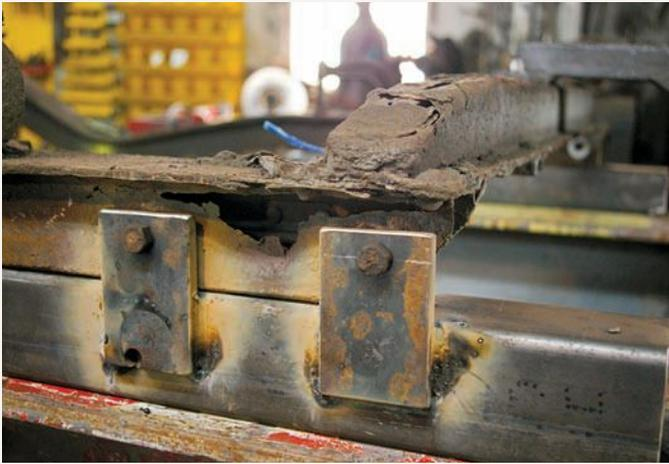
Here is a detail photograph of the kind of damage André found throughout the original frame. Continued stress at this and other points would have the potential to cause catastrophic damage to the Pontiac and serious injuries to its occupants.
