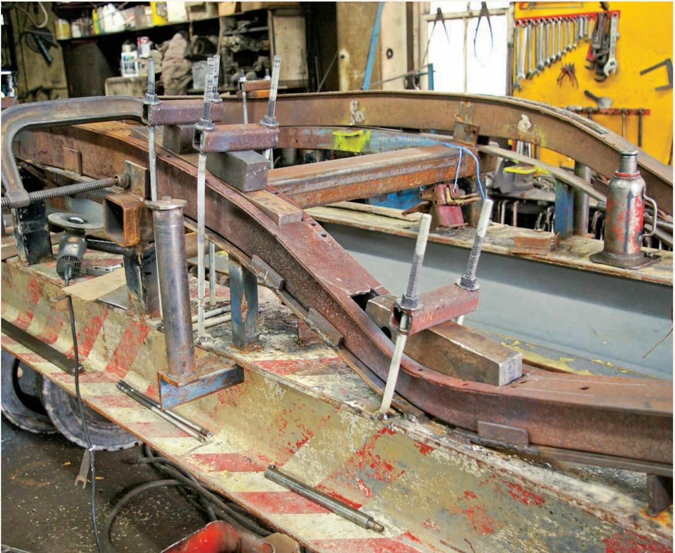
With less metal to bend, both the interior and exterior surfaces of the frame were evenly heated. Using blocks, threaded clamps, time and a lot of patience, the frame began to conform to the jig—note the difference between the rails.
