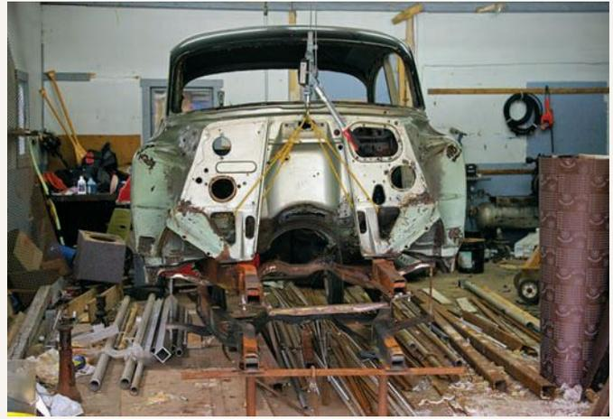
In spite of the misfortune that befell the body shell earlier in the restoration, its removal from the first shop proved to have some benefit, as it was conveniently on hand to serve as a second pattern for comparing with the reworked replacement frame.
