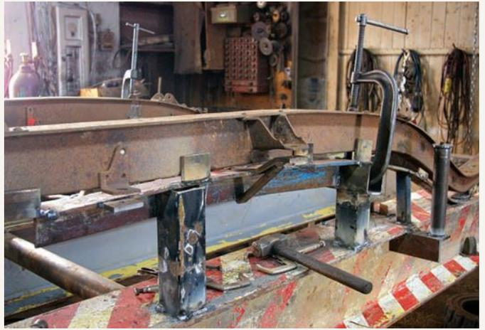
With the frame jig completed, it was time to drop the replacement frame into position and secure it using C-clamps. Initially, it was thought that the rails could be manipulated simultaneously, so each of the crossmembers remained riveted to the side rails.
