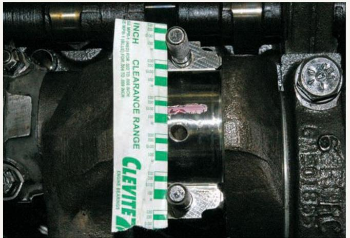
A critical step in any engine rebuild is verifying that all tolerances are within factory specs; here the clearance on one of the connecting rod bearings is being verified with Plastigauge during the assembly process.
