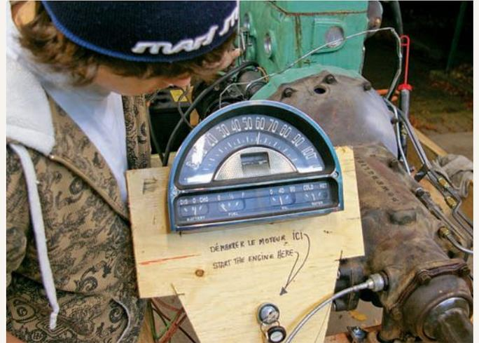
The Pontiac's original gauge cluster was bolted to a piece of plywood, and corresponding connections were made, enabling André to monitor the engine's status during initial break-in testing.
