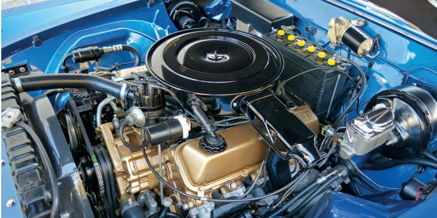
To modernize the drivetrain for William Clay Ford Sr, in late 1968, Ford engineers installed a contemporary 460-cu.in. V-8, C6 automatic and rear end. The engine compartment has since been restored four times—in 1974, the mid-1980s, the mid-1990s and early 2000s.
