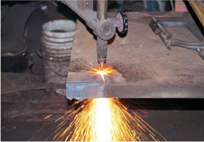
Blocks of solid steel were cut to assist with the process of bending the frame rails to match the jig, after taking internal measurements of the frame rails. The blocks spread the clamping force over a broader area, thereby preventing the formation of kinks or creases.
