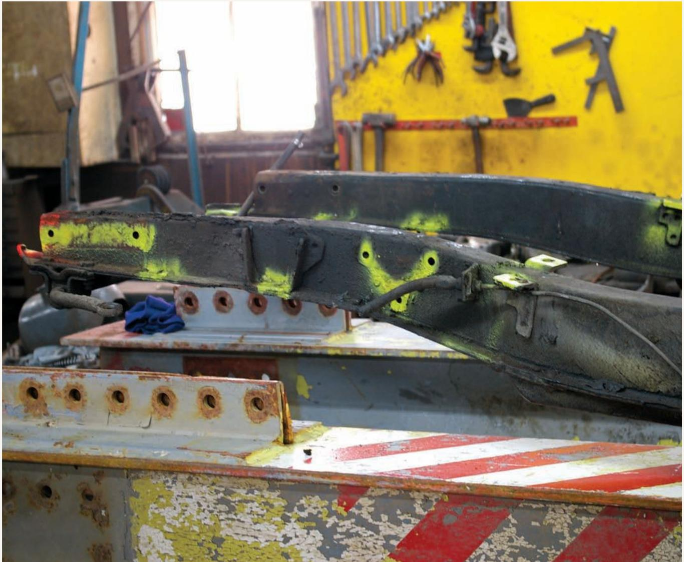
Before attempting any alterations to the replacement, André documented critical mounting points for suspension parts and body mounts on the well-corroded original frame. Here, he has done so using fluorescent yellow paint.
