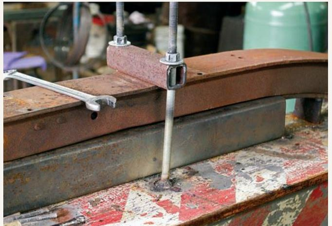
To maintain pressure where needed during the bending process, a makeshift but very effective clamp was fabricated using box tubing, threaded rods, nuts and washers. This system was employed at several locations along the length of each frame rail.
