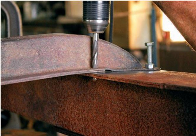
Both frame rails received their corrective treatment, then it was time to begin to reattach the crossmembers. Corresponding mounting holes were cleaned using a drill bit; nuts and bolts were used to hold the crossmember and frame rail together temporarily.
