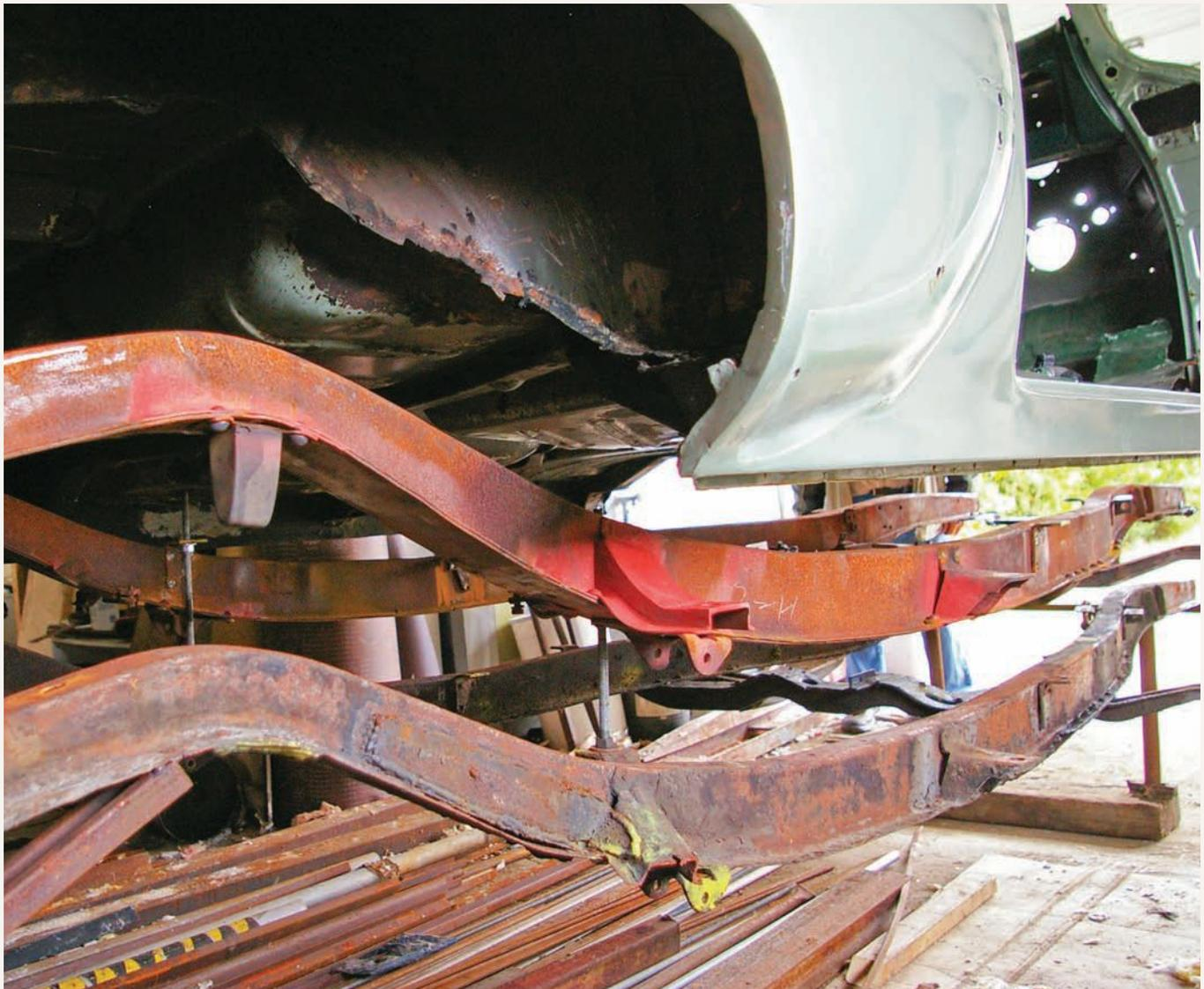
Here, the body has been carefully suspended above the reworked frame, which sits above the original. After a year of meticulous, time-consuming work, the new frame had been reshaped into a nearly perfect match. According to André, that was a huge relief.
