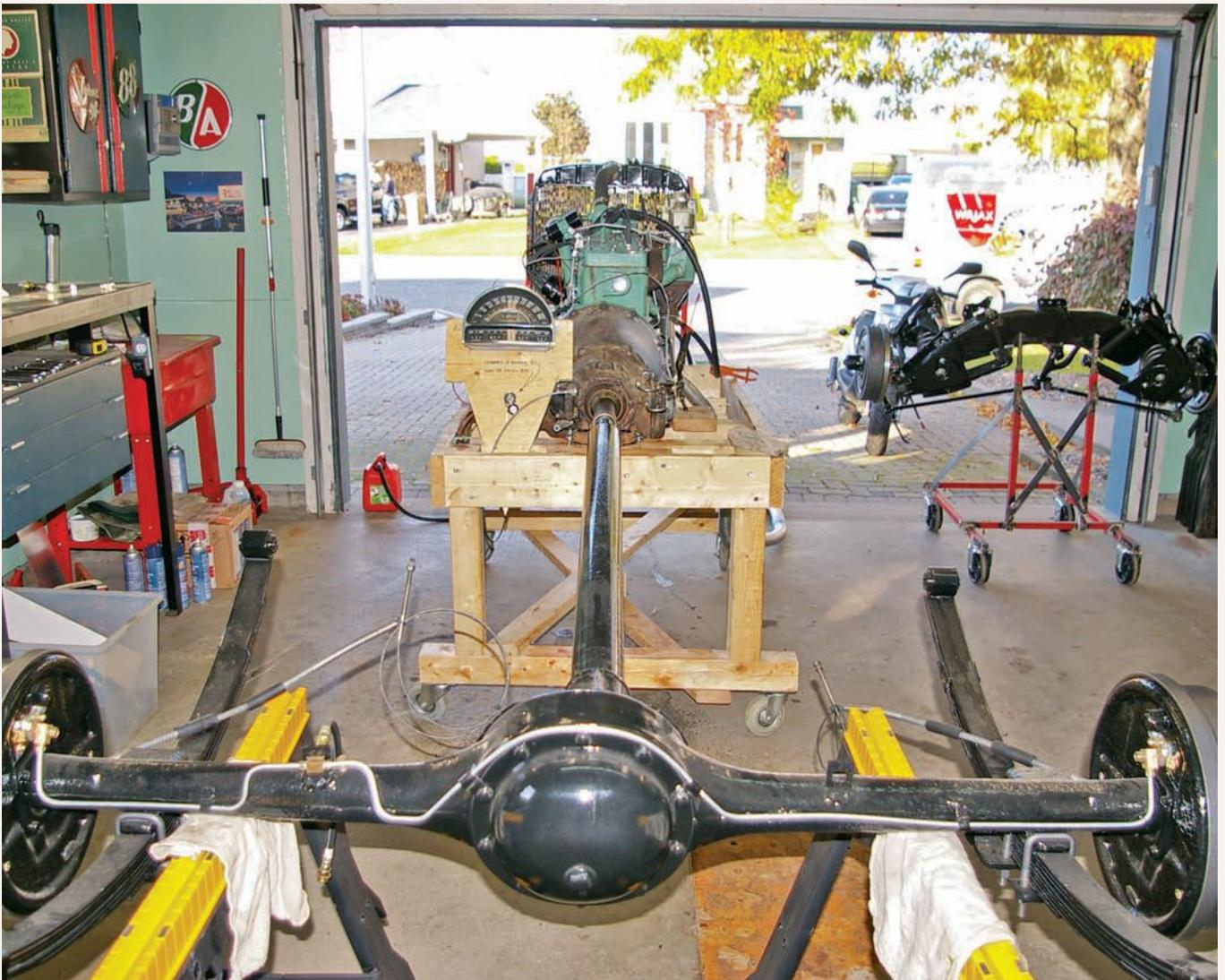
Rebuilt earlier, the differential/torque tube assembly was aligned via sawhorses and bolted to the transmission. Metal flex tubing was clamped to the engine's exhaust manifold and routed out the garage doors in anticipation of testing of the drive systems. Join us in the next issue as we learn about the restoration of this Canadian-born 1953 Pontiac Pathfinder's body.
