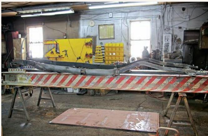
By the time André had obtained the new frame, two years had already passed since he had decided to restore the Pontiac. In this image, the difference in frame design has been discovered; fortunately, despite corrosion damage, the original remained true to its factory dimensions.
