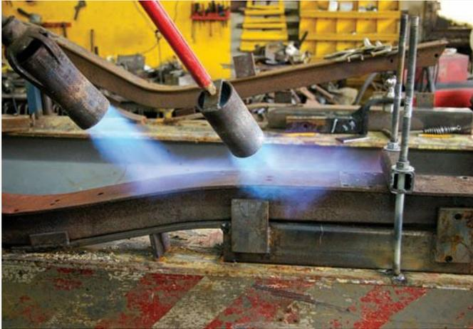
André and his colleague used propane burners to apply heat evenly to the steel, relaxing the metal in stages in order to slowly manipulate its shape to conform to the jig. This slow process would prevent damaging the frame's overall integrity.
