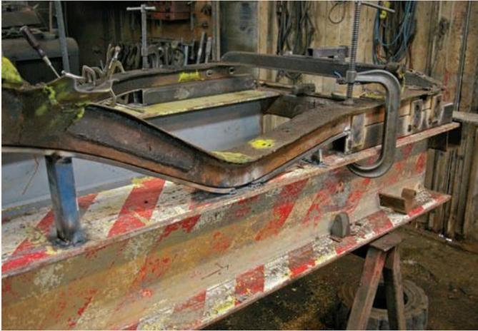
More tubing and strips of plate steel. The former was used to provide support for the latter, as the jig was carefully fabricated to match the contours of the frame. A series of clamps was used to hold everything in place while final adjustments and welds were made.
