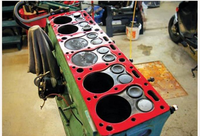
New crankshaft shell bearings have been inserted, and the pistons—installed during the engine's second rebuild in 2005—have been reinstalled, too, after it was ensured that none of the valves needed attention. Here, the new cylinder head gasket has been positioned.
