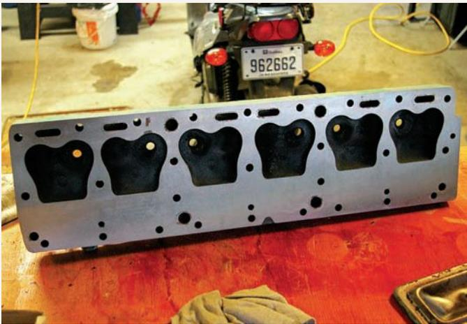
In order to avoid further issues with the top end of the straight-six engine, André had the mating surface of the cylinder head milled. This process provides a better seal between the gasket and head, helping to prevent coolant leaks.
