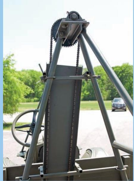
**PTO-connected, chain-driven prop starter proved a relatively straightforward—and safer—alternative to hand-propping aircraft.**
