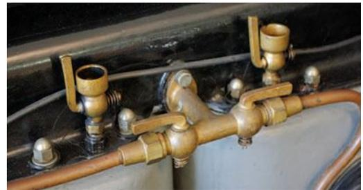
**Straight-six engine features bronze screw-in inserts on the top of the cylinder heads to permit access to the valves; manual levers flip up to disconnect spark plugs; glass fuses and cloth covered wiring make up the electrical system; fuel priming cups ease engine start-up.**
