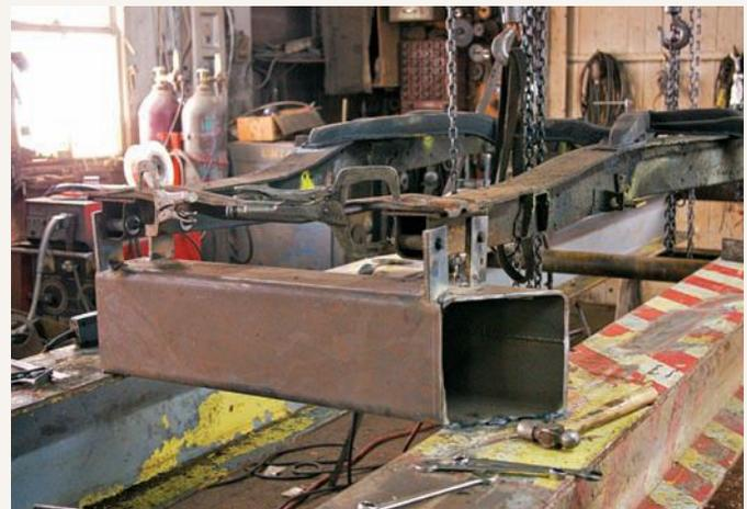
With the mounting points marked, the original frame was flipped over in order to begin to make a jig. To compensate for the frame's undulations, the front and rear mounts were elevated well above the platform using square tubing and plate steel.
