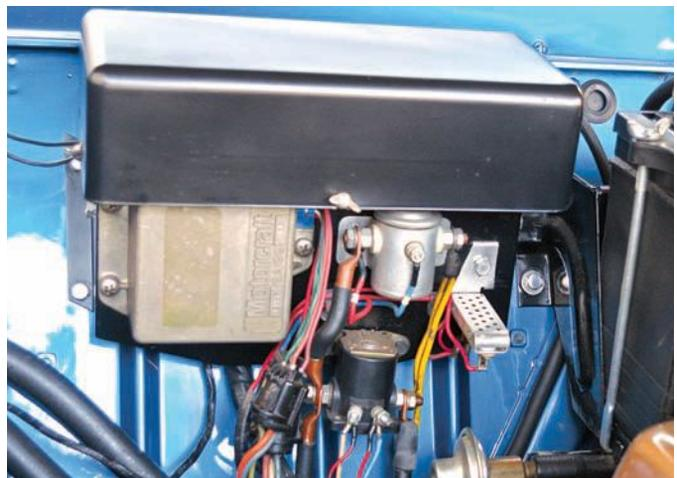
The stock vacuum-powered windshield wiper motor was exchanged for an electric one, the battery is a reproduction and the underhood electrical components are shielded from above.
