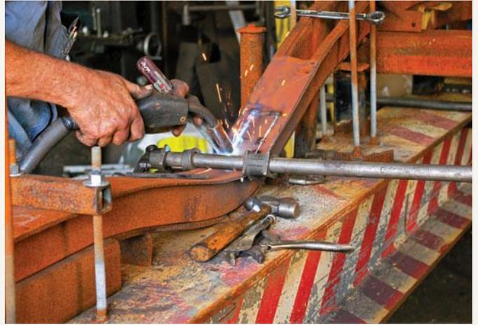
After the frame rails were sufficiently re-contoured, the pieces that had been cut from the bottom of the rails in order to facilitate bending without fracturing were welded back in place. The welds were later dressed to make the splice invisible.
