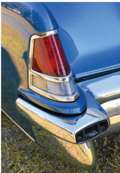
**The left taillamp assembly swings open to reveal the fuel door. To achieve a lower roofline without sacrificing passenger headroom, the compartment floor dropped down between the frame rails. Consequently, the dual exhaust system was routed outside of them. Featuring resonators, mufflers and a crossover pipe near the rear axle, it terminates at bright tips through the rear bumper. Each fin of the wheel covers was hand fitted.**
