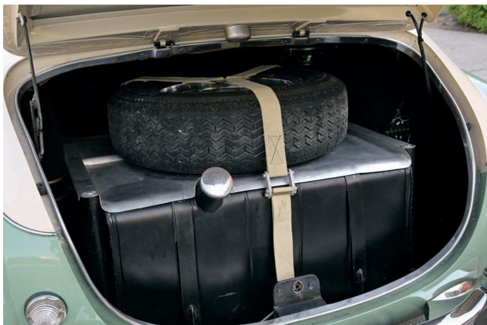
Prepped for racing when new, this was the only C-3 equipped with a massive 40-plus gallon fuel tank that filled the entire trunk; leather straps are also unique.
