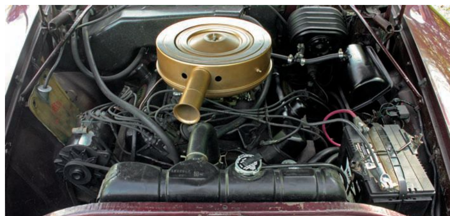
This Imperial's 350-hp, 413-cu.in. V-8 has propelled it just over 41,000 miles in the last 57 years, without requiring major work. The four-wheel drum brakes are assisted by a booster (upper right); the current owner added the factory deep-tone accessory horn (lower right).
