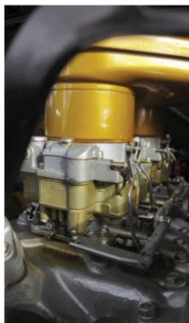
A 341-cu.in. Hemi V-8 engine featuring two Carter four-barrel carburetors, internal performance upgrades and a 9.25:1 compression ratio was exclusive to the Adventurer.
