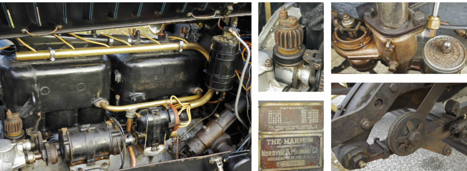
Cylinders are cast in threes on the 447-cu.in. straight-six. Owner guesstimates it will churn out 70 horsepower. Fuel mixture is fired courtesy of Bosch ignition. The functional air compressor is extremely rare. Carburetion is by updraft Stromberg.
