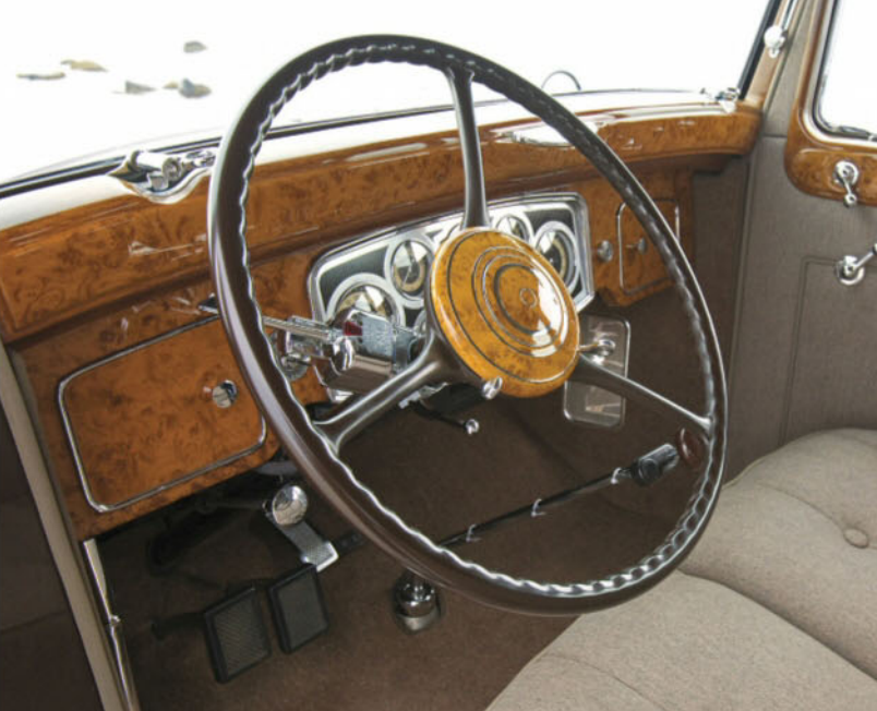
Power assisted by your forearms only, the steering is made somewhat easier on this 4,985-pound car with the large diameter wheel. All Eight and Super Eight models received a brown steering wheel for 1934.
