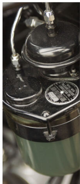
Packard's 145hp, 384.8-cu.in. straight-eight is everything you have heard: a paragon of smoothness with an abundance of torque; Bijur Automatic Lubricator was rebuilt by the owner and automatically lubes the chassis.
