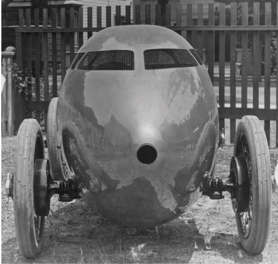
A rear view of the Miller's tapered aluminum bodywork shows the exit for the exhaust positioned in the center of the tail. This was cutting-edge design for its era.
