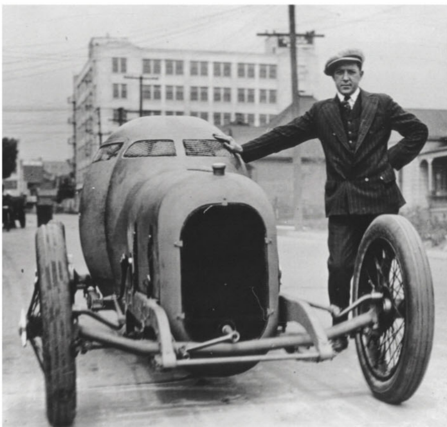
Outside the Miller factory in Los Angeles, the Golden Submarine shows off its dropped tubular front axle. The unknown man demonstrates its low profile.
