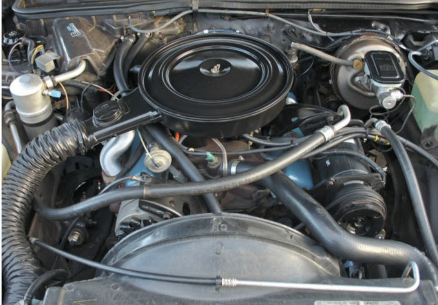
This Chevrolet 305-cu.in. V-8 has not been apart in more than a quarter-million miles. Retrofitting an R134A-compatible A/C compressor is a project for this winter.
