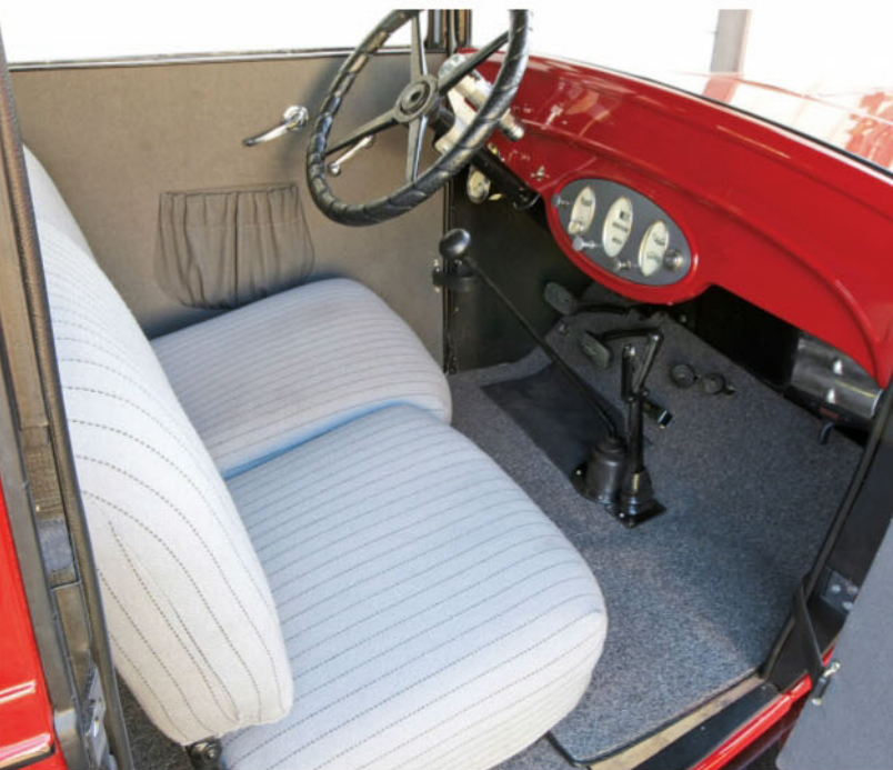
The interior was restored with materials from LeBaron Bonney. The instruments remain untouched, but the speedometer is still giving good service. The original plate glass was replaced with modern alternatives.
