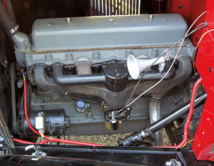
The 194-cu.in. engine was the first Chevrolet straight-six in an uninterrupted string that would continue until 1984. The six-volt electricals were deemed adequate and retained.
