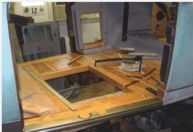
With a considerable amount of the wood framing completed, portions of the body could then be re-secured, enabling Tom to start with metal repairs. Only the lower sections were corroded, which were corrected with fabricated patch panels.
