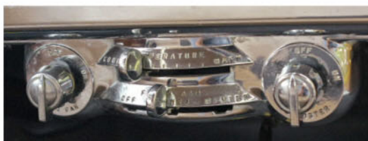
Fresh air/temperature/fan control sits below radio with clock on right. Interior door panels are made of thin wood paneling.
