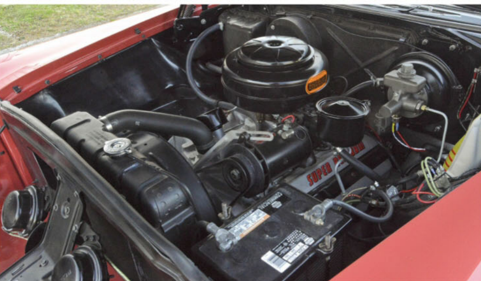
Dodge's top engine in 1955 was this Super Red Ram OHV V-8 with hemispherical combustion chambers. Performance, as a result, is strong.
