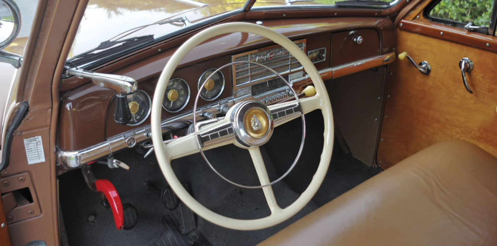
Steering wheels in the P-18 series measured 17½-inches in diameter, 1/2 inch larger than in the P-17 series. Red handle is parking brake.
