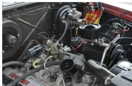
Dodge's top engine in 1955 was this Super Red Ram OHV V-8 with hemispherical combustion chambers. Performance, as a result, is strong.
