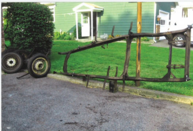
Once the floor and rear body-support framing was completed, the sub-structure was removed from the frame, the latter then stripped of the remaining running gear and suspension systems. They were subsequently media blasted to bare metal and sealed in primer.
