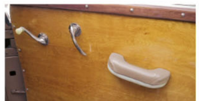
Fresh air/temperature/fan control sits below radio with clock on right. Interior door panels are made of thin wood paneling.
