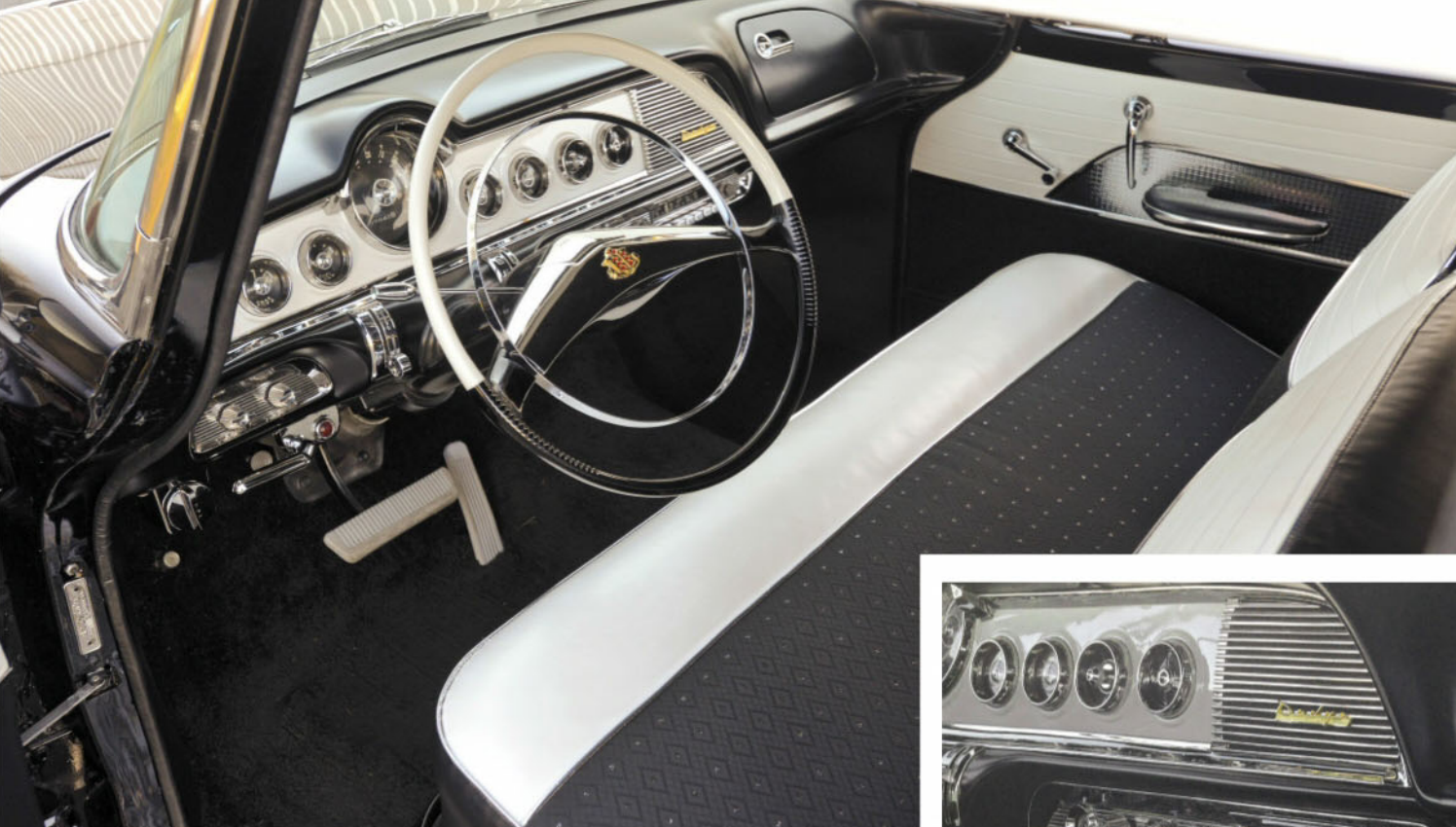
Black-and-white interior color scheme was commonplace on premium Dodges in 1955. Note the total absence of dashboard padding. That dash does, nonetheless, boast full instrumentation and extensive use of chromed accents.
