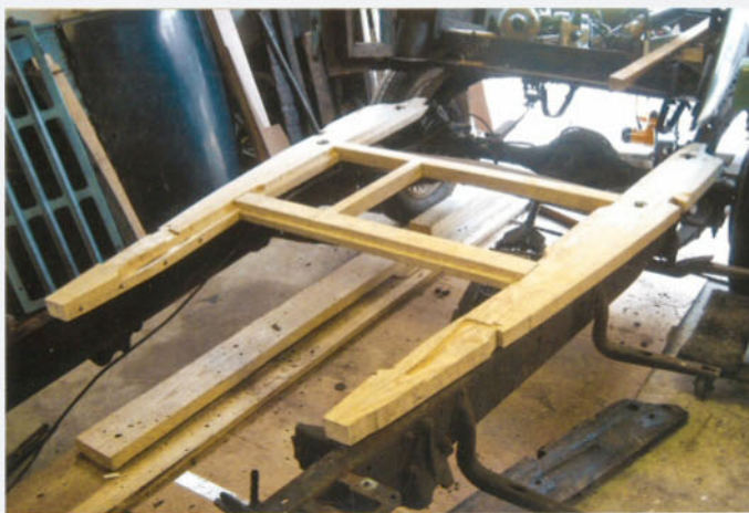
Restoration work began again, with the body support rails that would be secured to the steel frame. Since so little was left of the originals, only a vague pattern could be made; it then took time and patience to massage the wood to its final functional form.
