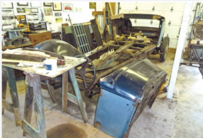
The car's disassembly began right away, made easy by the fact that nearly all of the factory wooden framing behind and below the body had rotted to pulp. Non-stock engine and transmission followed, at which point the project was put on hiatus.
