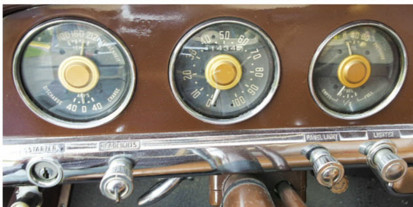
Metal instrument panel features water temp/amp meter, left; 100 MPH speedometer, center; oil pressure/fuel, right. Radio grille standard.
