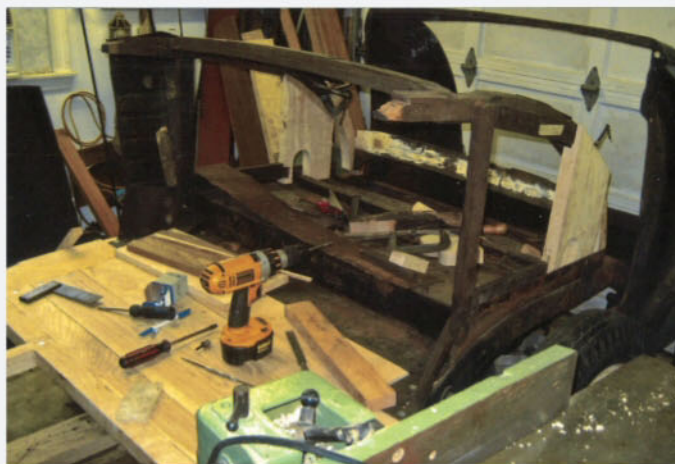
Wood fabrication then progressed to the floor and rumble seat frame, a small portion of which still existed. Tom chose ash over oak due to its lighter weight; besides, it's more durable, resists excessive flexing and is also easier to work with.
