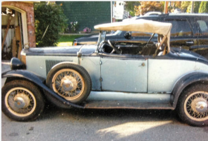
The 1931 Graham Model 46 Roadster as it appeared at the time of its 2008 purchase. Clearly tired, it was essentially missing its interior upholstery, the top was heavily weathered and the body wore a blue two-tone paint scheme over its original black color.
